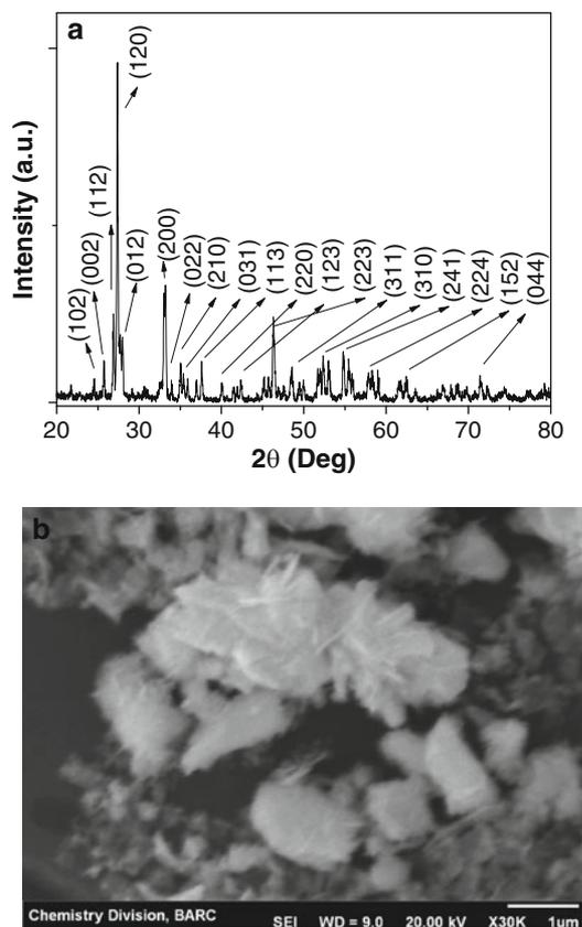
**Fig. 8.2** (a) XRD pattern and (b) SEM image of sonochemically synthesized  $\text{Bi}_2\text{O}_3$
