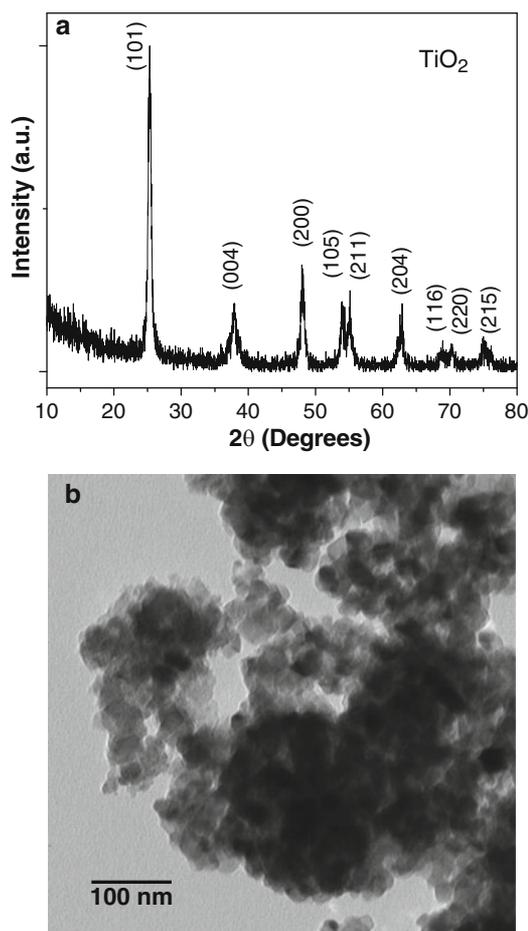
**Fig. 8.1** (a) Powder XRD pattern. (b) TEM image of TiO<sub>2</sub> nanoparticles
