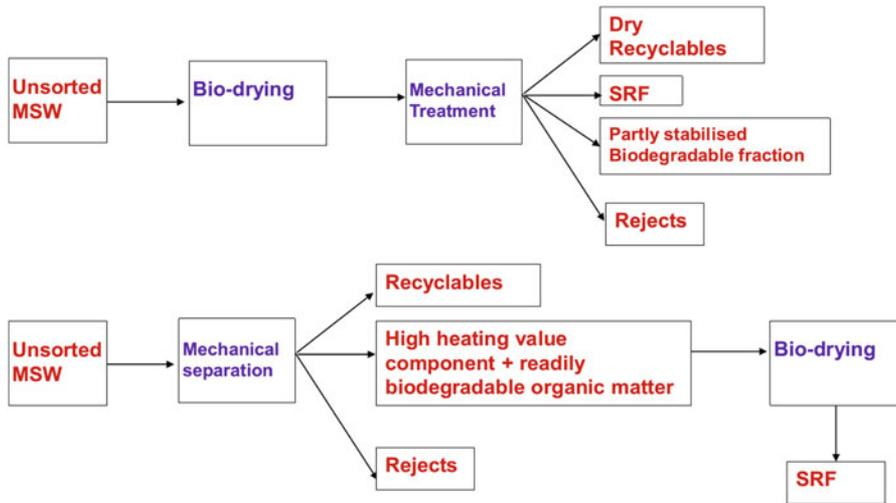
**Fig. 1.3** Simplified configurations of MBT process (Source: Anurag Garg 2012)
