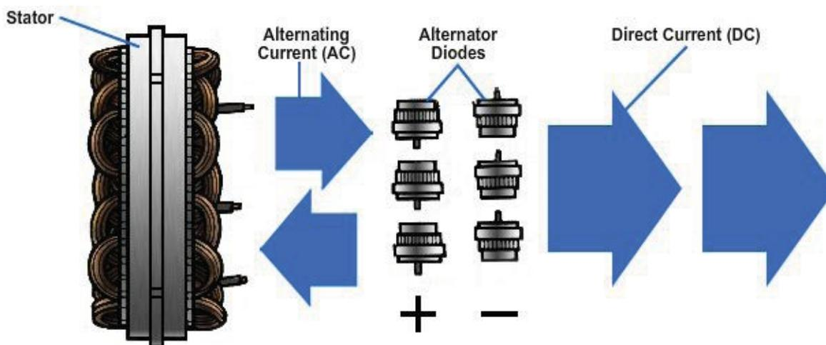
**Figure 6-16 – Several diodes are needed to convert AC into DC.**
