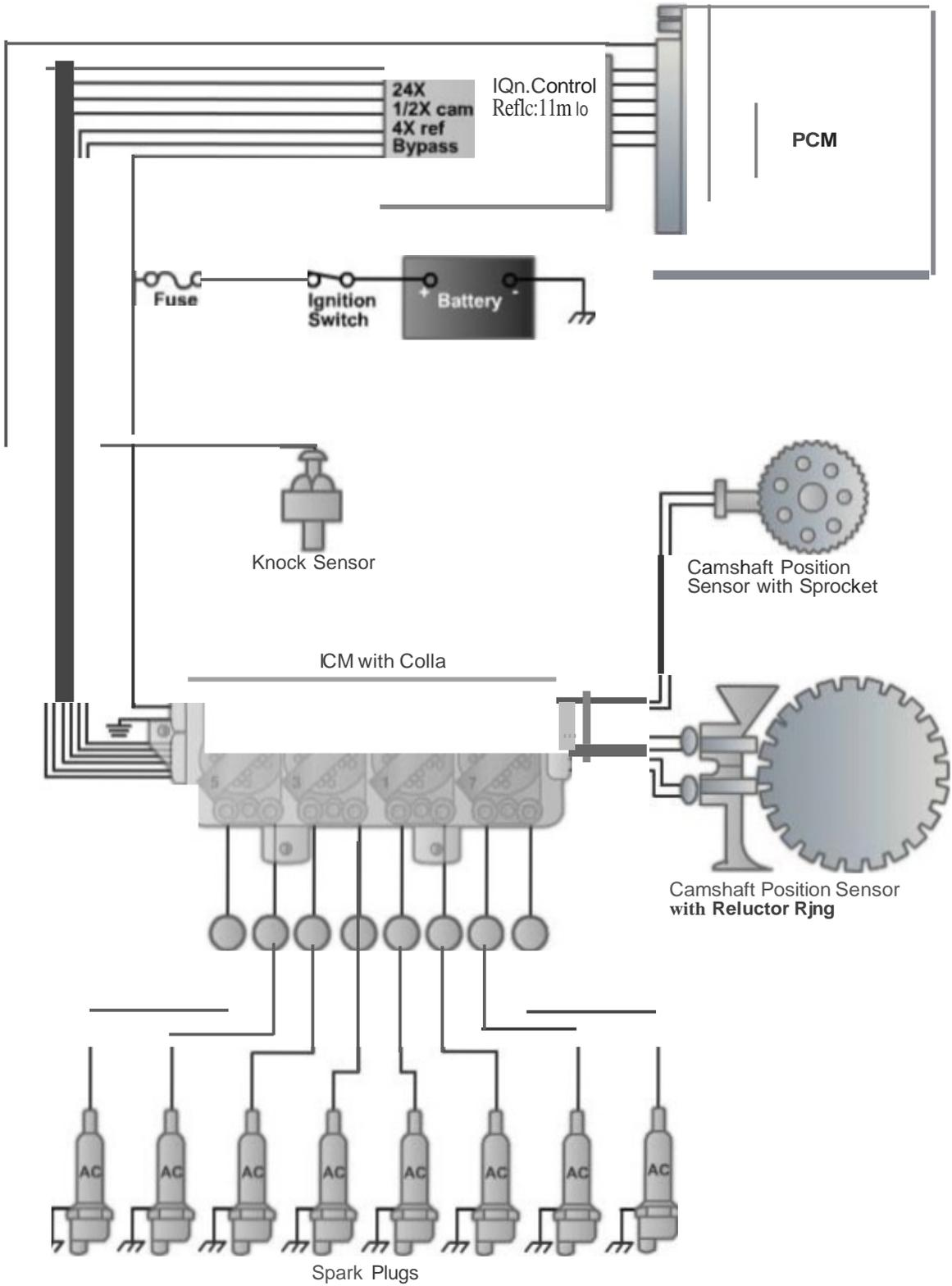
Figure 6-33 -Schematic distributorless ignition system.
