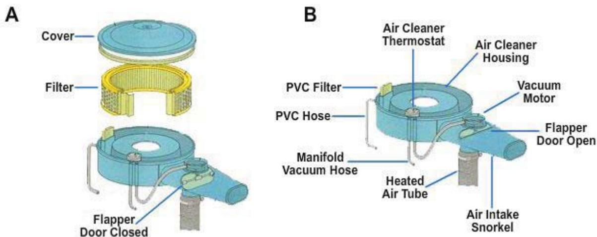
**Figure 5-119 - Checking the operation of a thermostatic air cleaner.**
