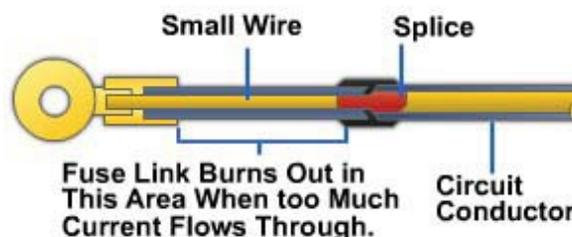
**Figure 6-50 – A typical fuse link.**
