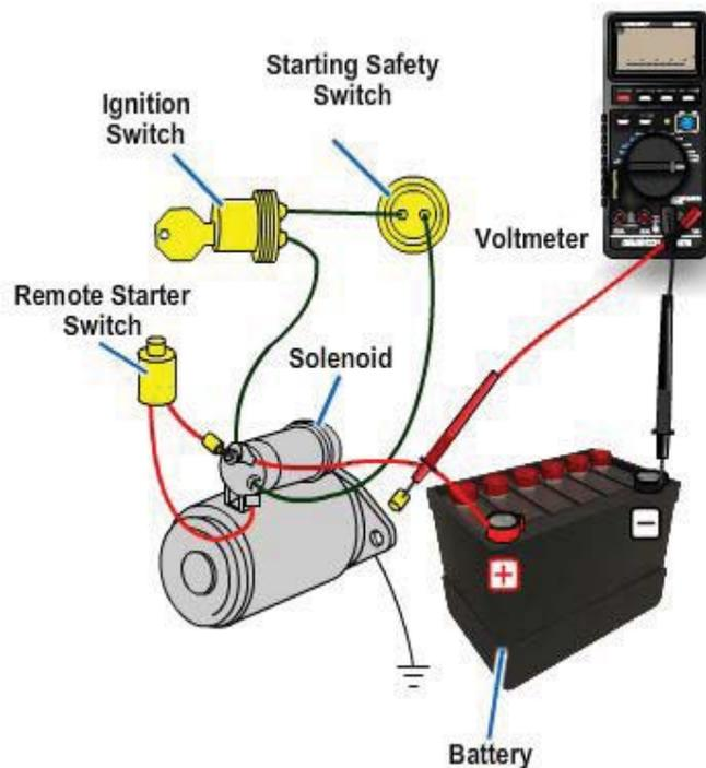
Figure 6-29 - Starter ground circuit resistance test.
