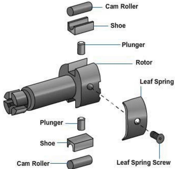
**Figure 5-63 – Exploded view of a rotor assembly showing the cam rollers and shoes.**
