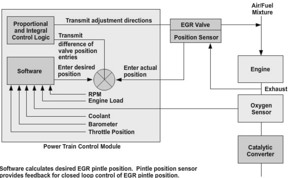
**Figure 5-124 - Block diagram represents the relationship between a power train control module and the EGR system.**
