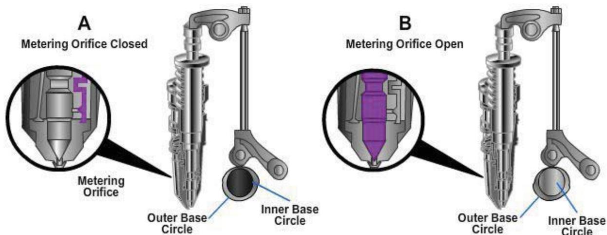
**Figure 5-84 - A PT fuel system, the camshaft actuated injector.**
