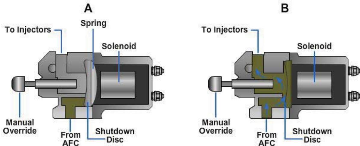
**Figure 5-91- Operation of PT fuel pump shutdown valve.**
