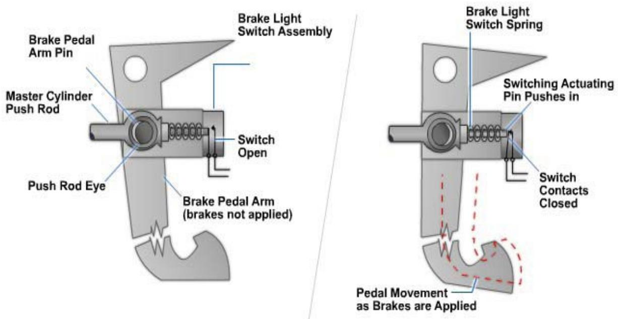
**Figure 6-53– Brake light switch action.**
