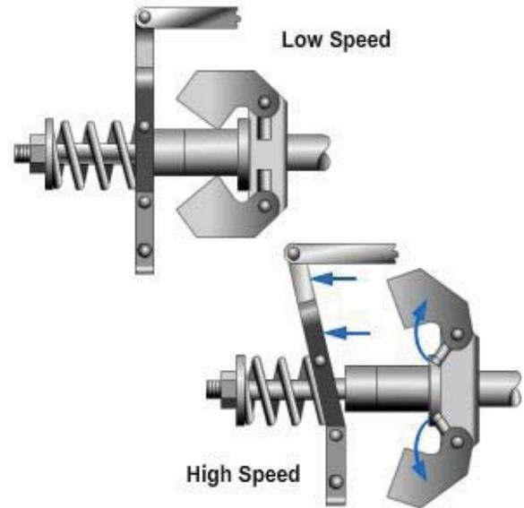
**Figure 5-87 - As rotational speed increases, the centrifugal force of the governor flyweights force the governor plunger to the right.**
