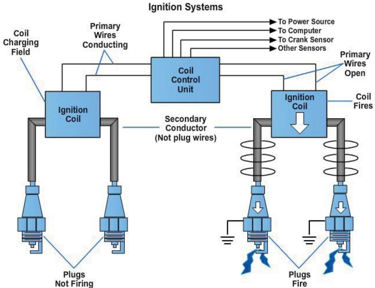
**Figure 6-34 - Illustration of a distributorless ignition operation.**
