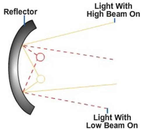
**Figure 6-42 – Light beam projection is controlled by filament placement.**
