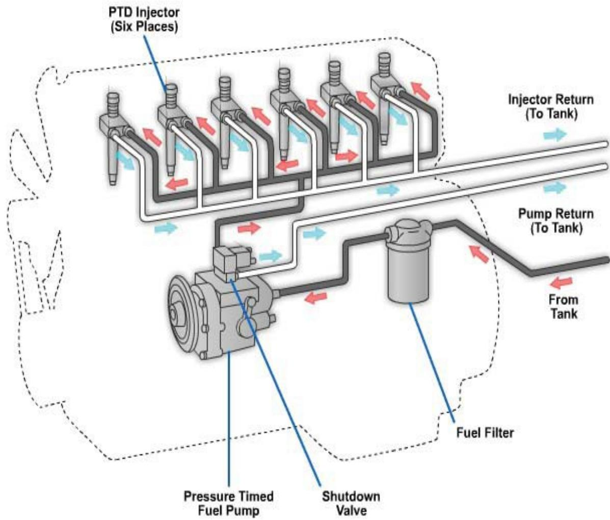
**Figure 5-83 - Basic components of the Cummins Pressure-Time Fuel injection system.**
