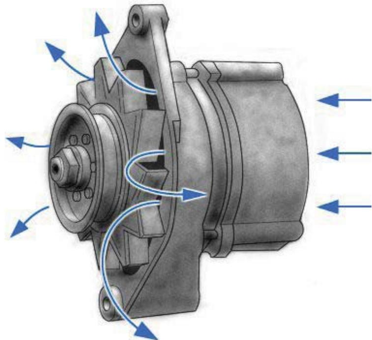
**Figure 6-11 -Cooling fan draws air through to cool the diodes.**
