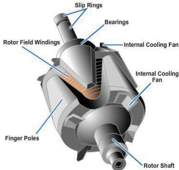
**Figure 6-5 – Components of a rotor.**
