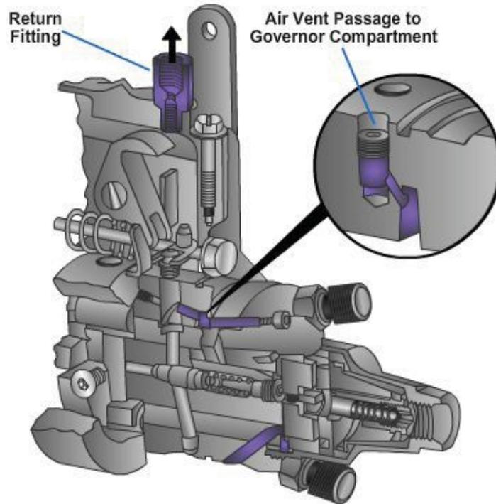
**Figure 5-68 – The oil return circuit allows excess oil in the distributor pump to return to the fuel tank.**
