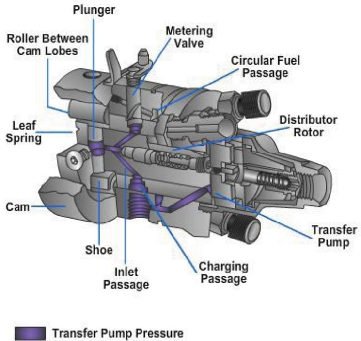
**Figure 5-66 -Fuel flow during the opposed plunger pump's charging cycle.**
