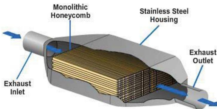
**Figure 5-132 - Monolithic catalytic.**
