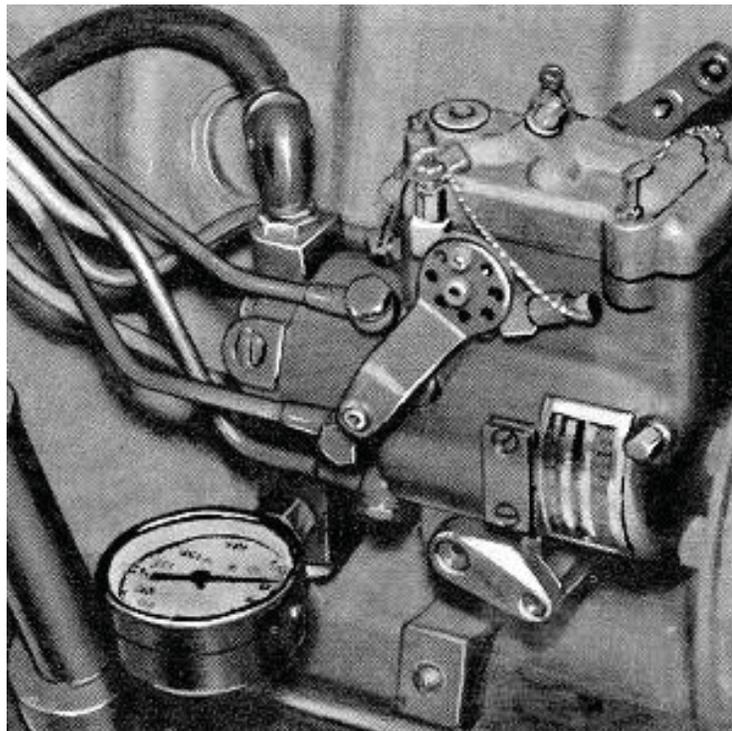
**Figure 5-72 Gauge installed for checking transfer pump pressure.**
