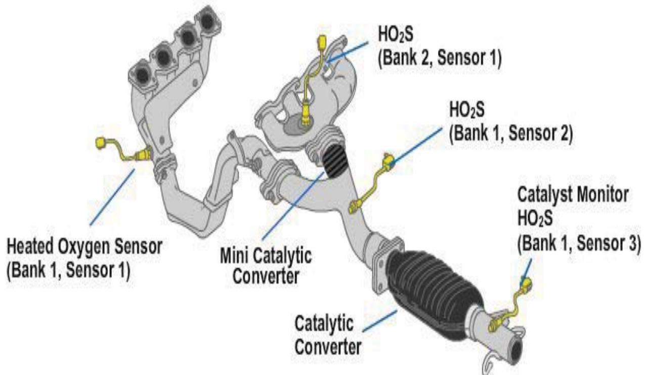
**Figure5-134- This engine is equipped with a mini catalytic converter and a main converter.**
