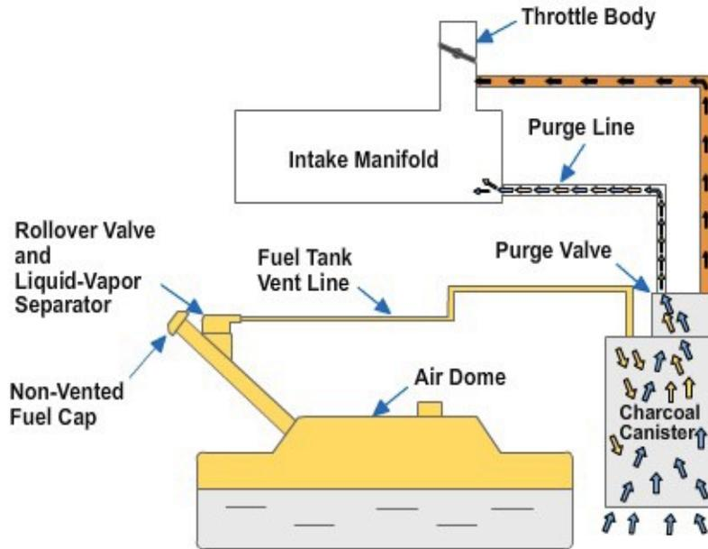
**Figure 5-111 - Evaporative emissions control.**
