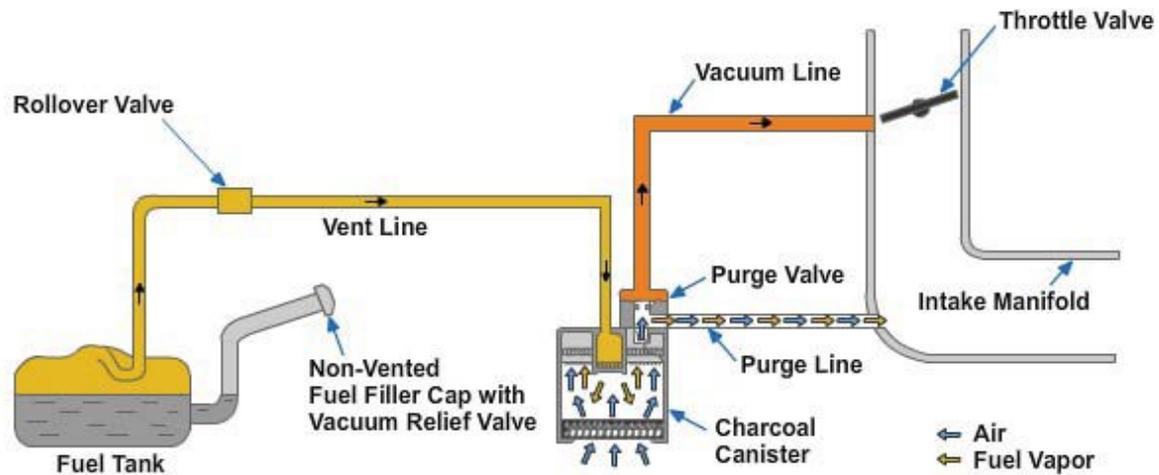
**Figure 5-113 - The operation of an evaporative control system and its related components.**
