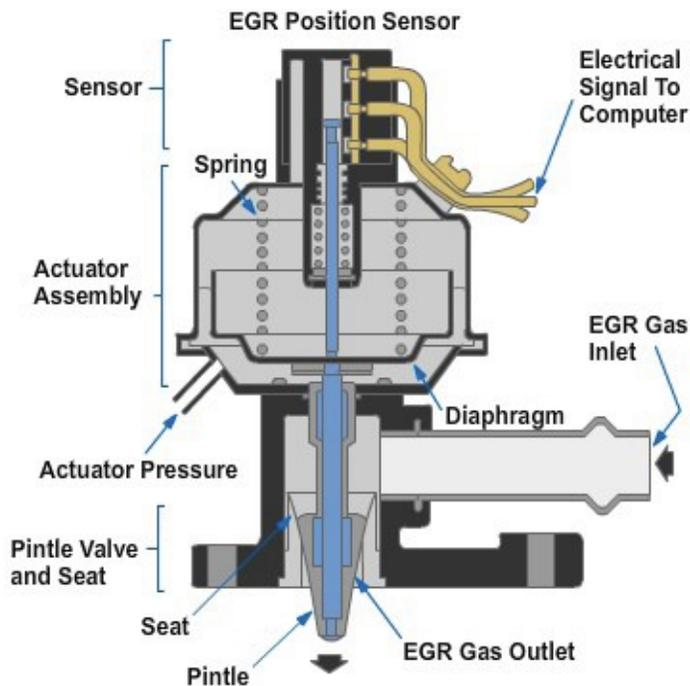
**Figure 5-122 - Cutaway of an Electronic-Vacuum EGR valve.**
