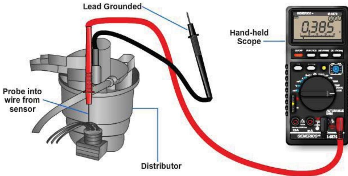
**Figure 6-37 - Testing a Hall-effect sensor.**
