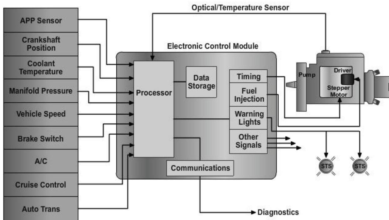
**Figure 5-82 - Example of an electronically controlled distributor fuel injection pump.**
