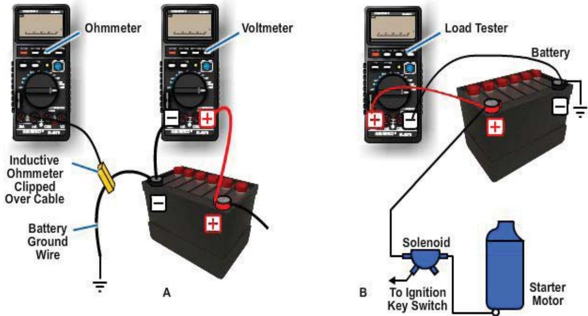
**Figure 6-27 – Starter current draw test.**
