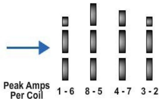
**Figure 6-40 – DIS coil amperage draw.**
