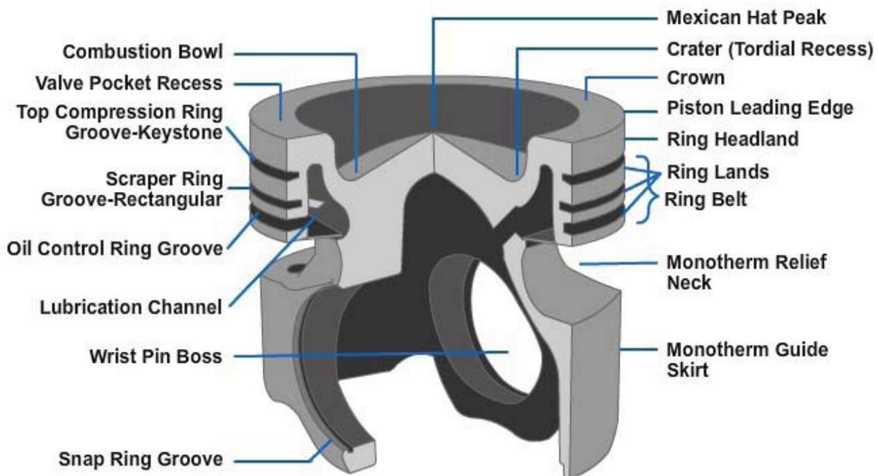
**Figure 5-150 - Cutaway view of a forged steel trunk Mahle Monotherm® piston.**
