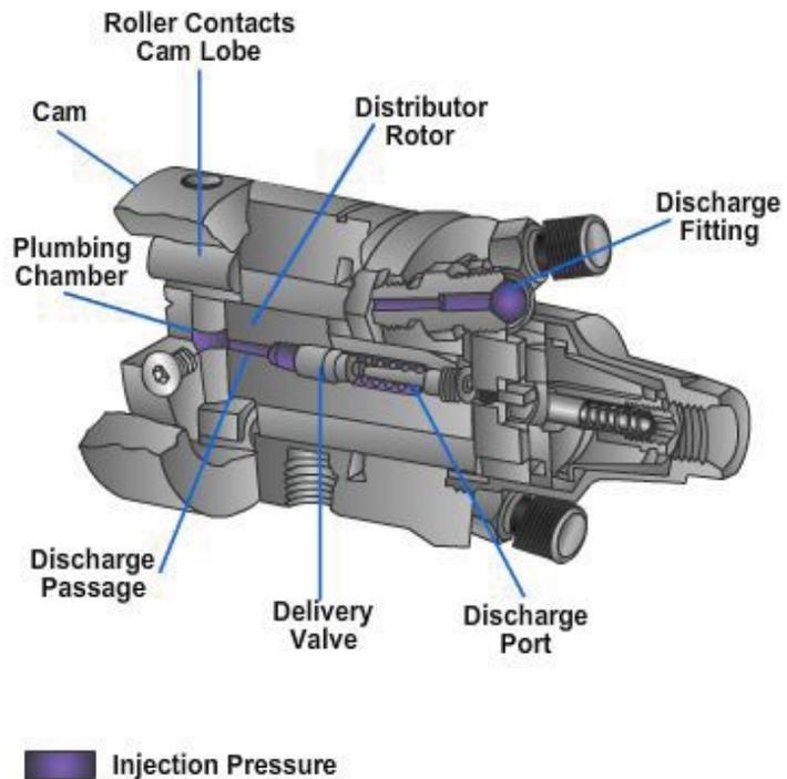
**Figure 5-67 -Cutaway showing the opposed plunger pump's discharge cycle.**
