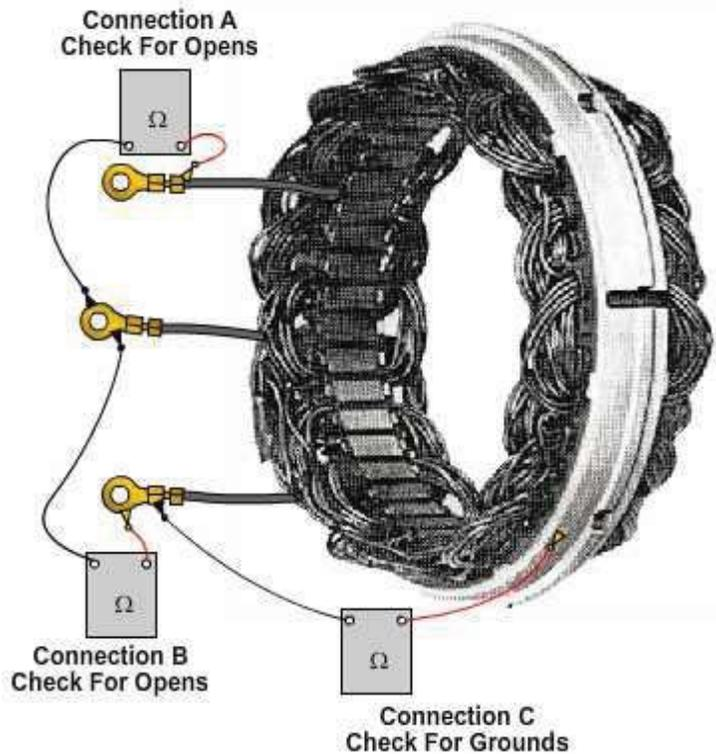
**Figure 6-25 – Stator test.**
