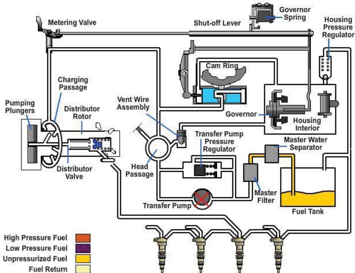
**Figure 5-64 - Fuel flow during the pumping cycle in a Stanadyne DB2 distributor injection pump.**
