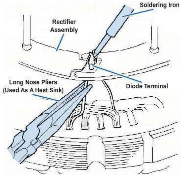
**Figure 6-23 – Soldering diode leads or stator to rectifier wires.**
