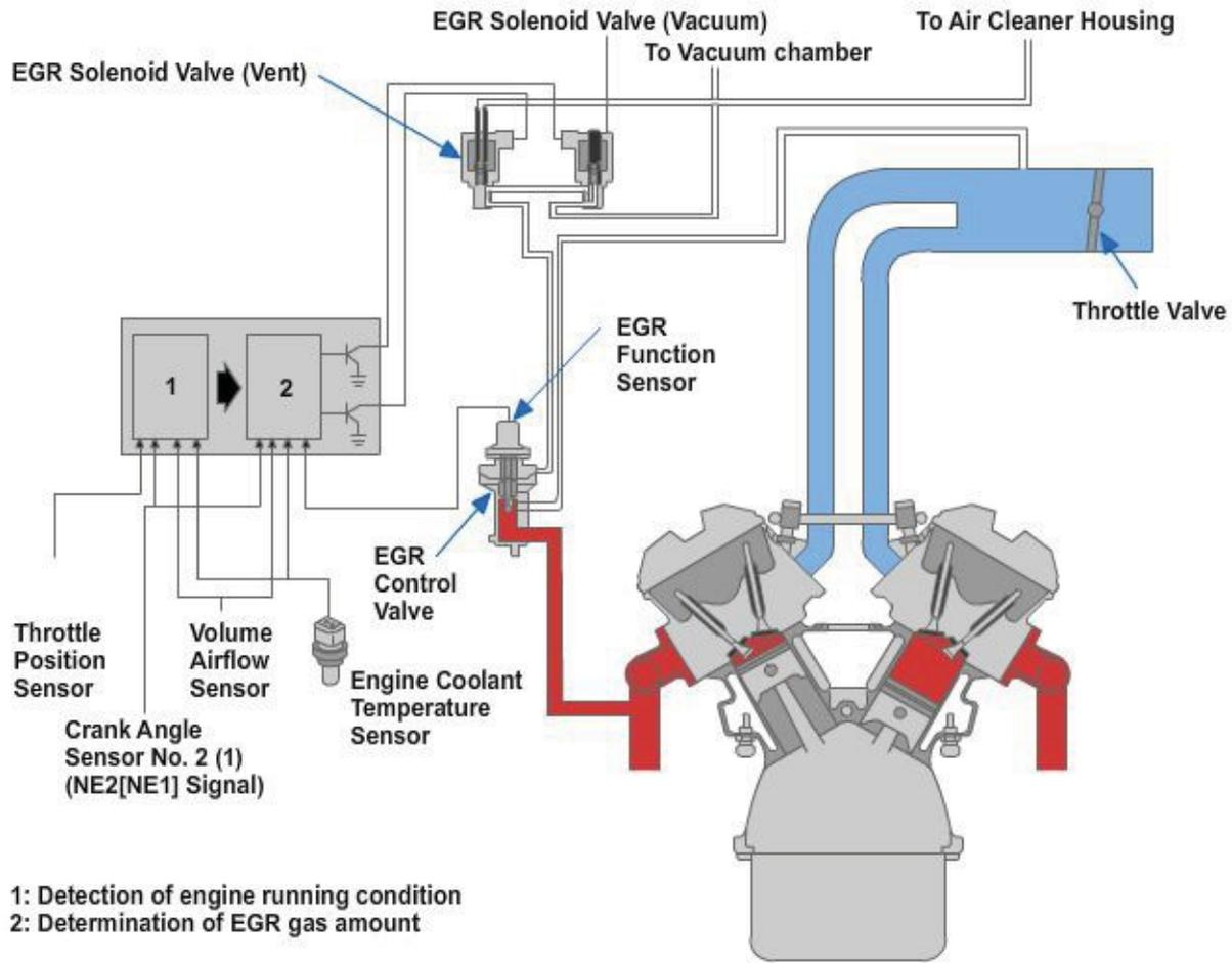
**Figure 5-123 - Diagram of control module monitoring and controlling vacuum-operated EGR valve.**
