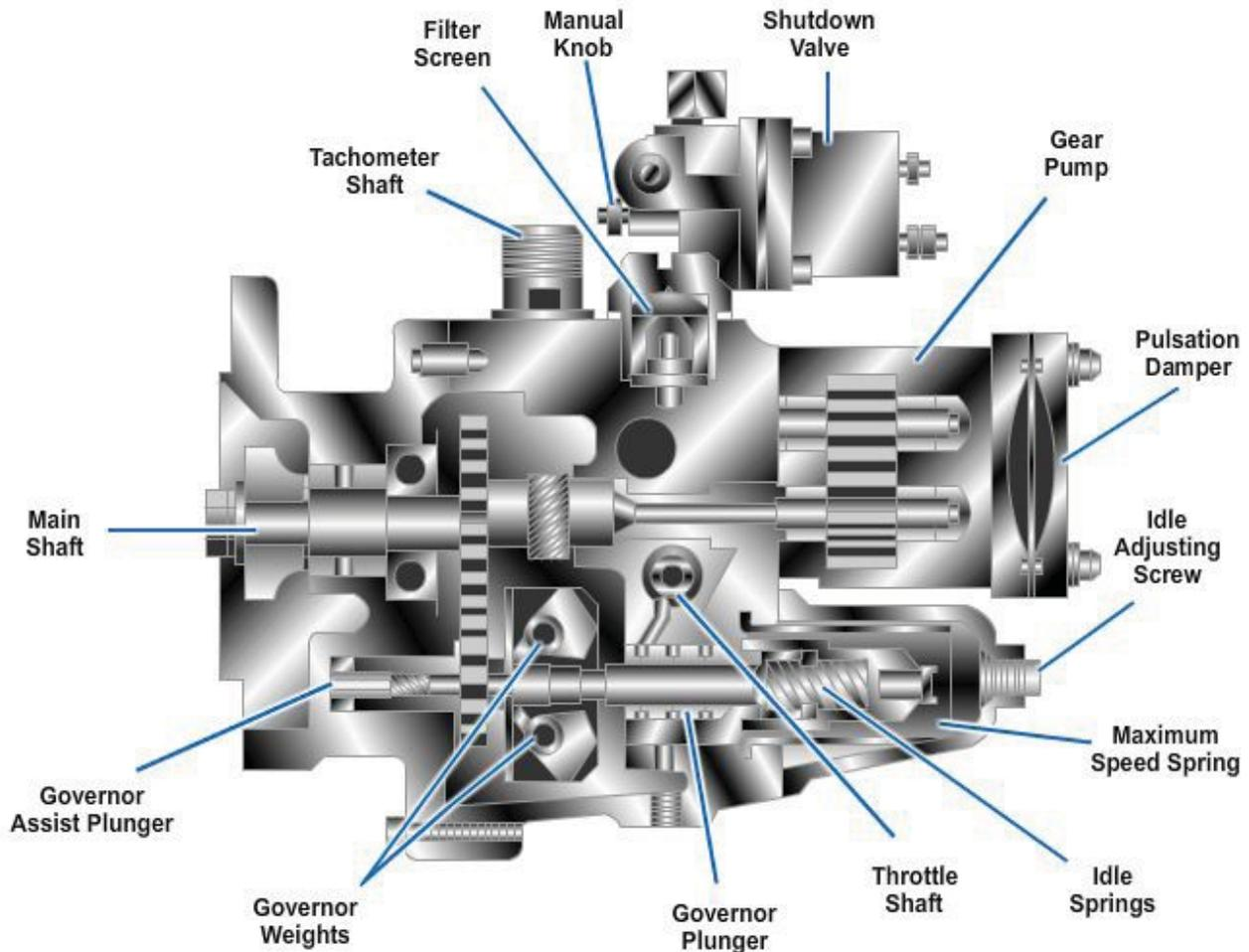
**Figure 5-85 - Components of the Pressure-Time Governed Air-Fuel Control (PTG-AFC) fuel pump.**
