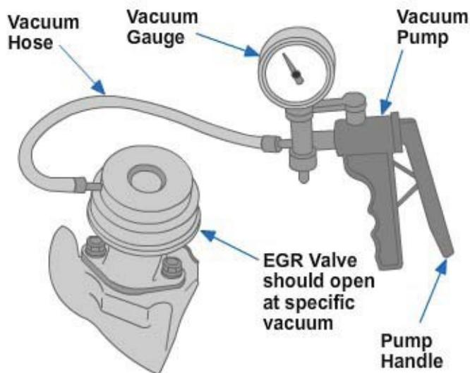
**Figure 5-126 – Testing the EGR system with a hand vacuum pump.**
