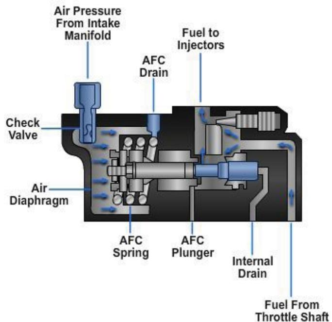
**Figure 5-90 - Cutaway showing components and fuel flow through the air-fuel control (AFC) assembly.**
