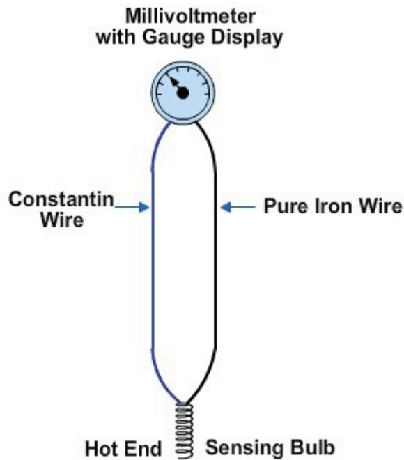
**Figure 5-146 – A pyrometer.**
