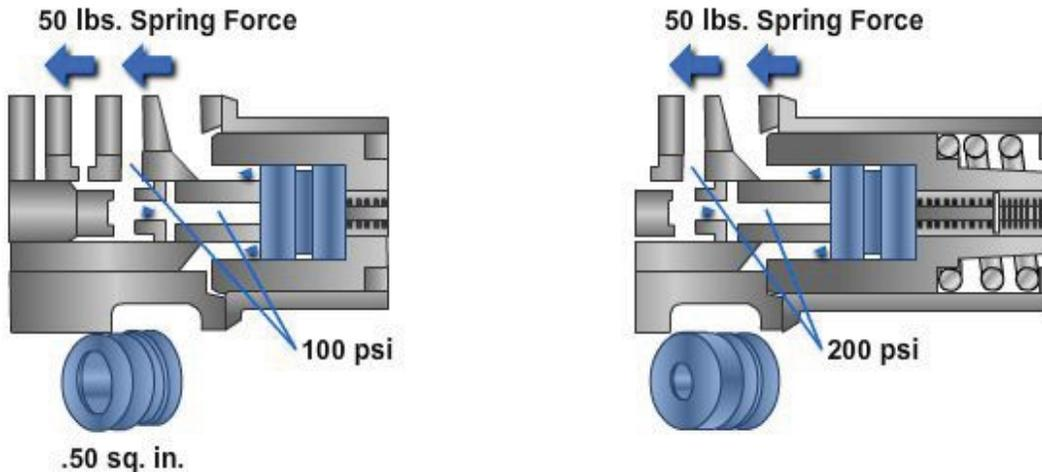
**Figure 5-88 - Button valve pressure regulator.**
