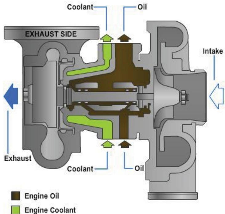
**Figure 5-101 – Oilflow through a turbocharger's center section.**
