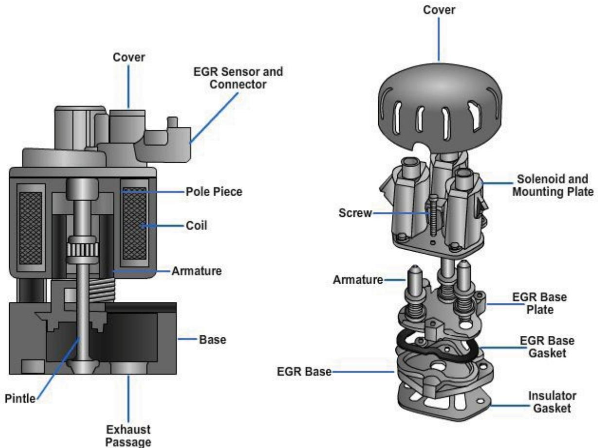
**Figure 5-125 – Cutaway view showing components of an electronic or digital EGR valve and a multistage EGR valve that uses three separate solenoids and valves.**
