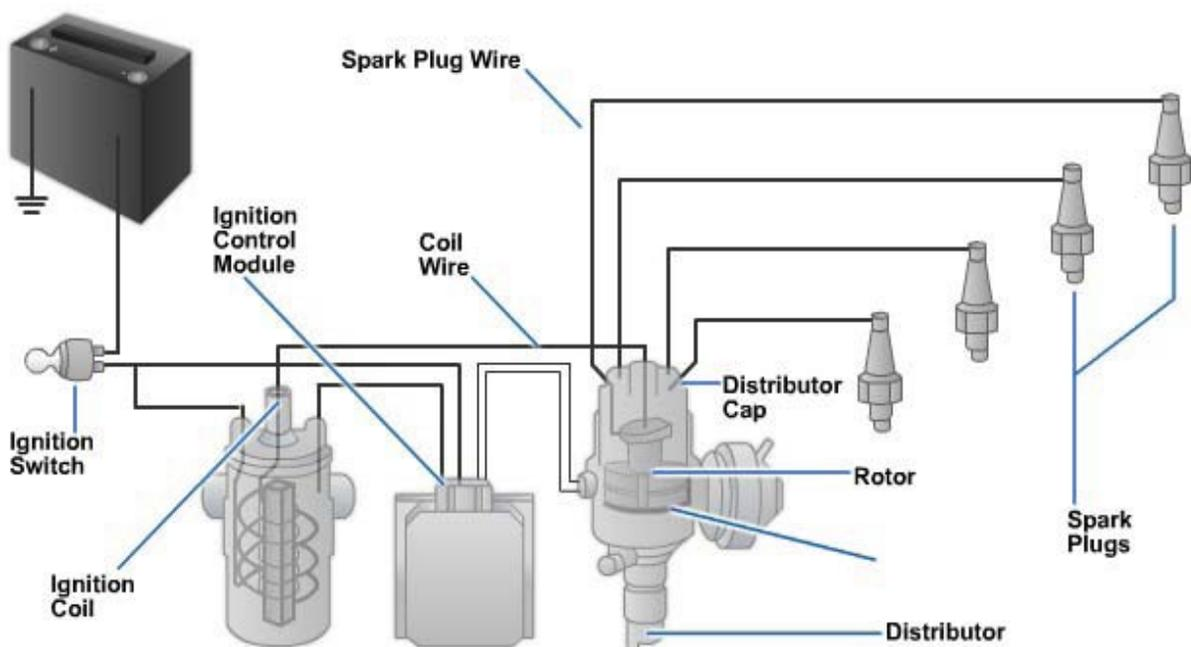
Figure 6-30 - Electronic ignition system.
