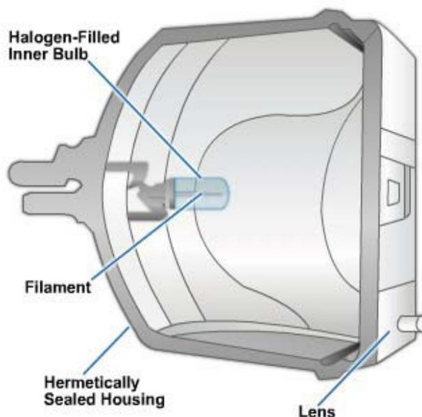
**Figure 6-41 - Halogen sealed-beam headlight with an iodine vapor light.**
