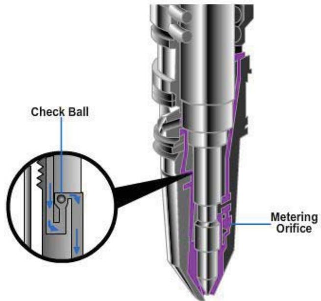
**Figure 5-95 - Injector cup operation.**
