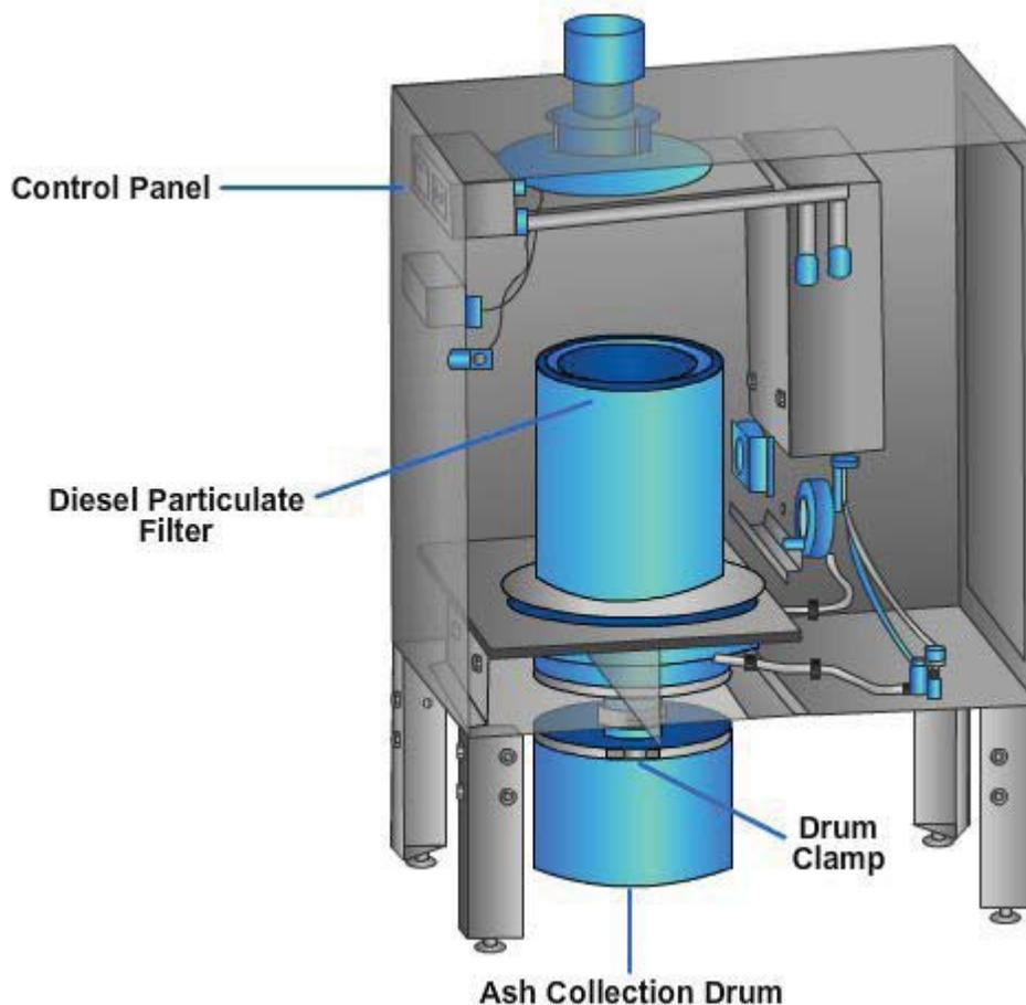
**Figure 5-147 - Diesel particulate filter cleaning system.**
