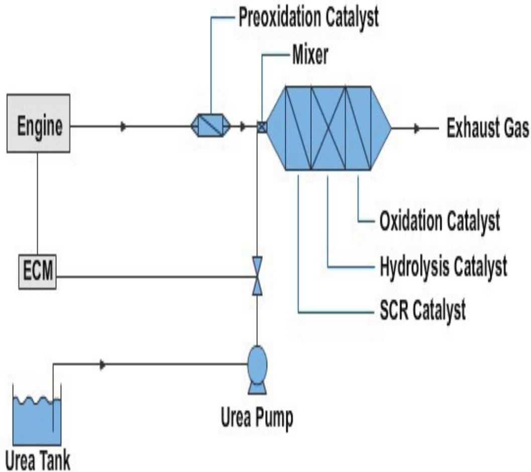
**Figure 5-148 - Schematic of a selective catalytic reduction components and operation.**
