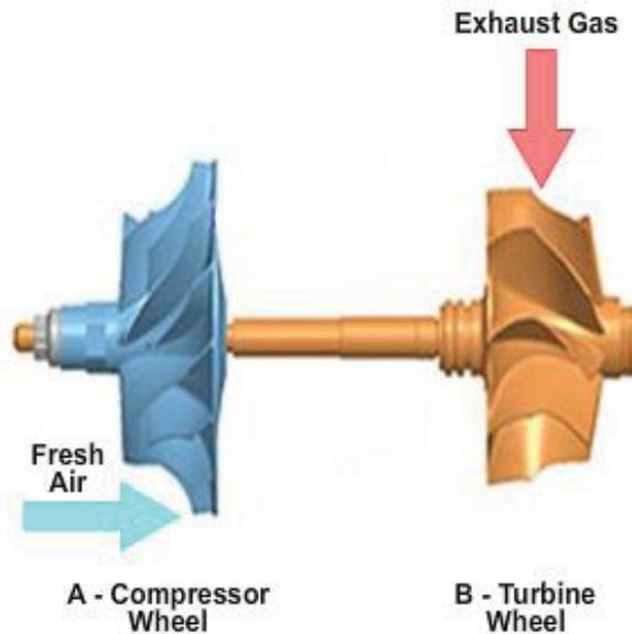
**Figure 5-100 - A-Compressor wheel and B-Turbine wheel.**
