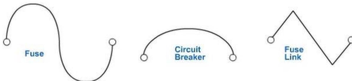
**Figure 6-47 - Electrical symbols for common circuit protection devices.**
