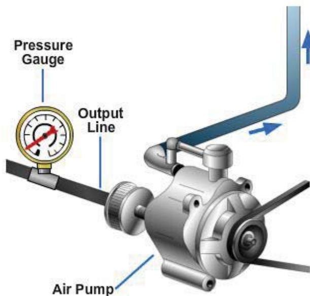
**Figure 5-131 – A pressure gauge can be used to check air pump output.**
