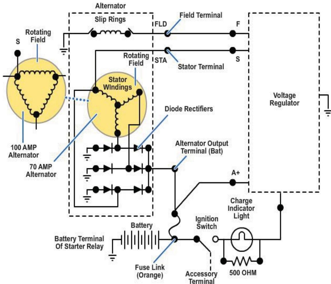
**Figure 6-13 - Wiring diagram showing the relationship between stator windings, rotor windings, diodes, and electrical connections.**
