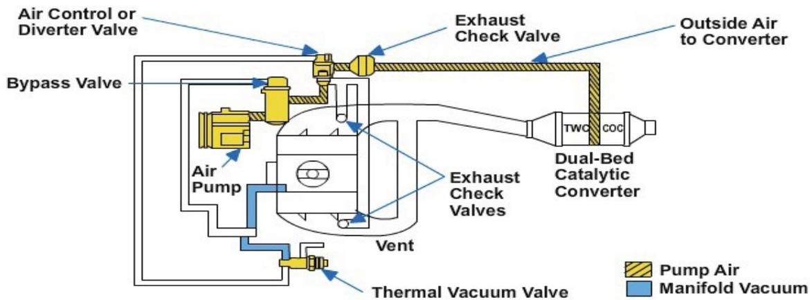
**Figure 5-136 - Diagram shows how an air pump forces oxygen into a dual-bed catalytic converter.**
