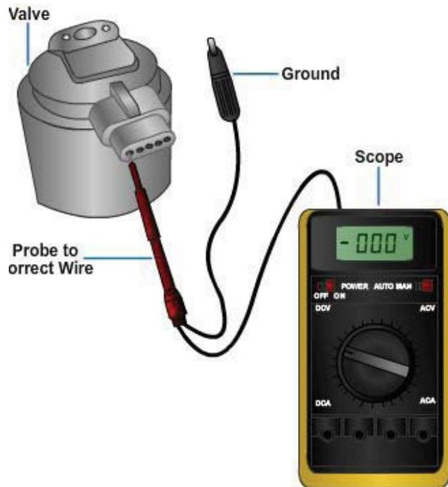
**Figure 5-127 – An oscilloscope can be used to check digital EGR valves and their ECM control circuits.**
