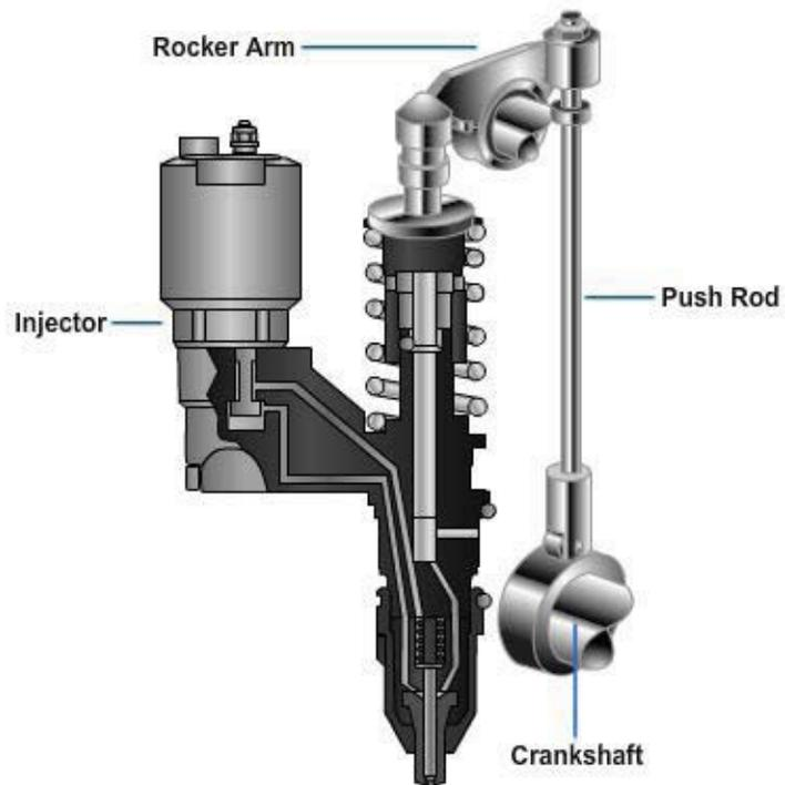
**Figure 5-79 – Example of an engine electronically controlled/mechanically actuated unit injector.**
