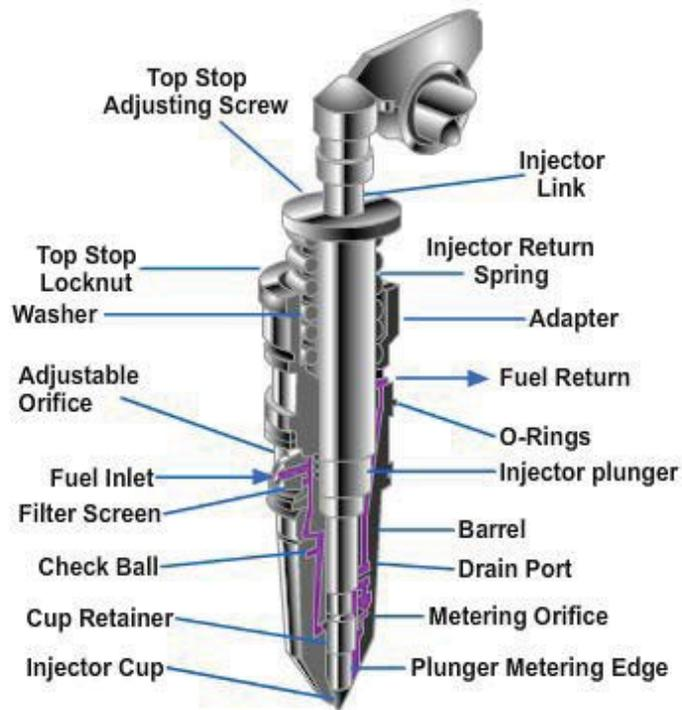
**Figure 5-92 – Components of a PTD Top Stop Injector.**
