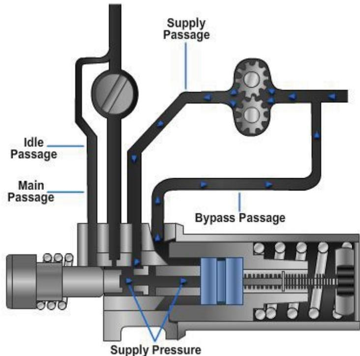
**Figure 5-89 - Fuel bypass occurs when the button is unseated.**
