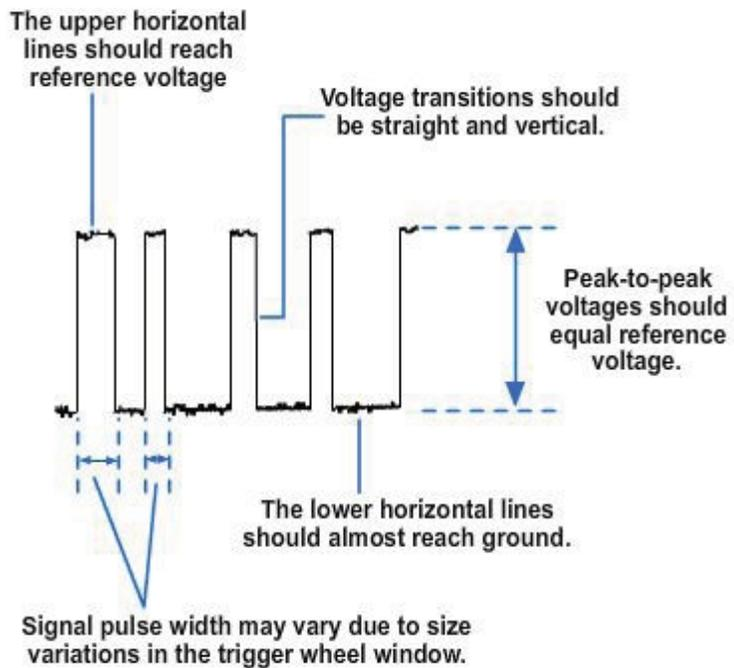
**Figure 6-38 - Typical waveform generated by an optical sensor.**
