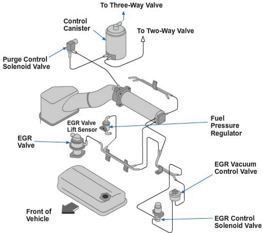
**Figure 5-115 -Vacuum hose routing diagram as it appears in a service manual.**
