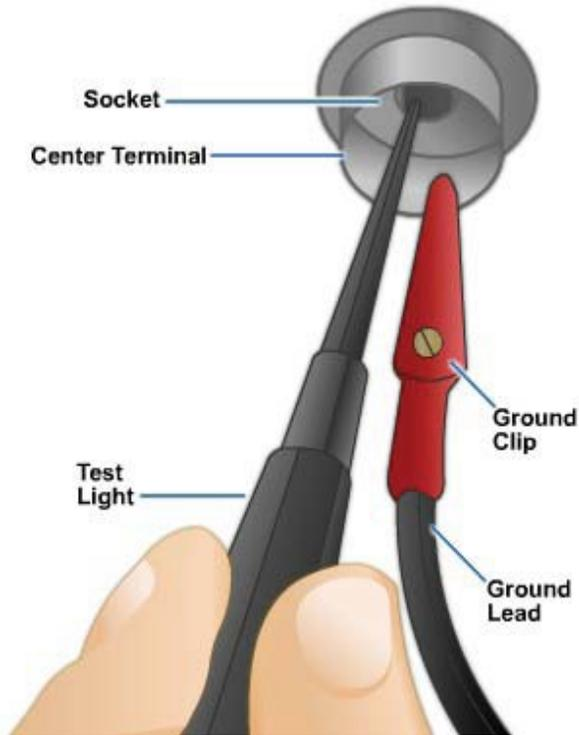
**Figure 6-45 – Check the socket with a test light.**
