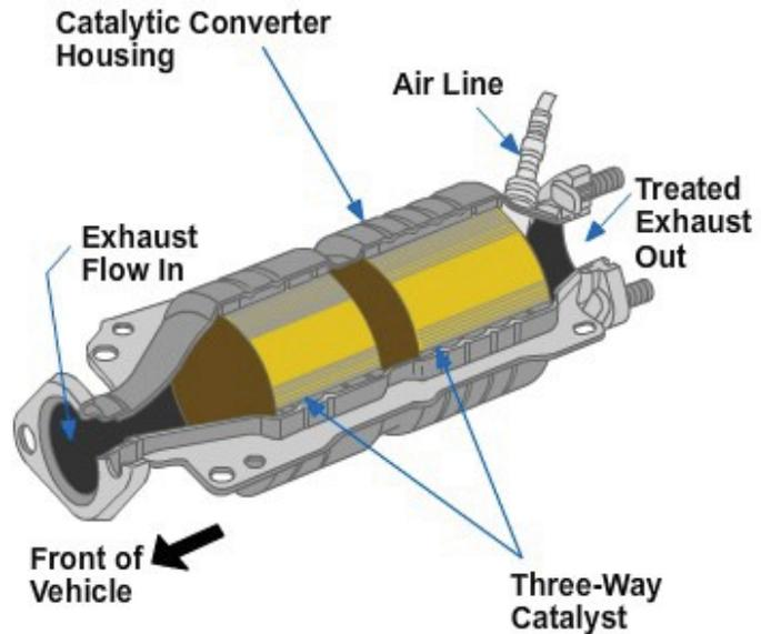
**Figure 5-135 – Cutaway of a dual-bed catalytic converter.**
