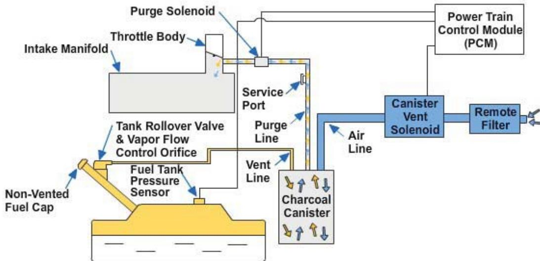
**Figure 5-114 - The canister evaporative emission system.**
