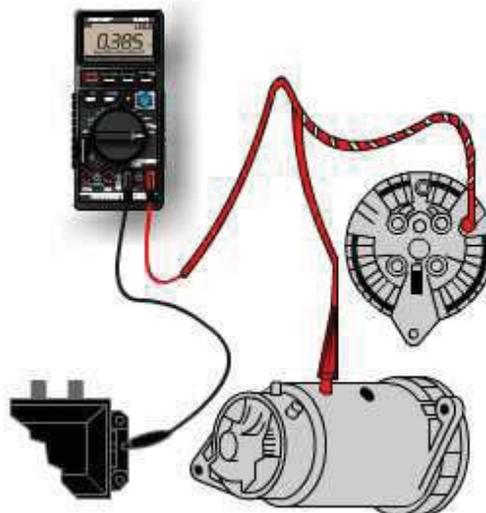
**Figure 6-20 – Regulator ground circuit resistance test.**
