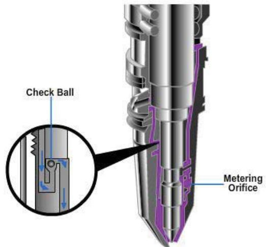
**Figure 5-93 – Fuel flow into the PTD Top Stop injector.**
