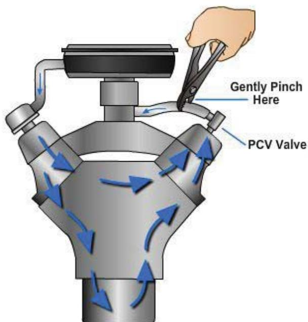
**Figure 5-117 -Pinch PCV hose with pliers. Ensure to wrap something around the hose so the hose is not damaged by the pliers.**
