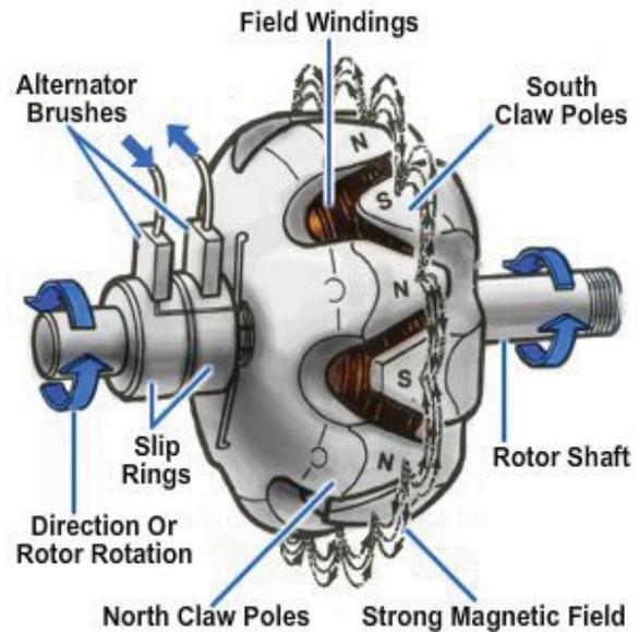
**Figure 6-4 – The rotor has claw poles that surround its windings.**
