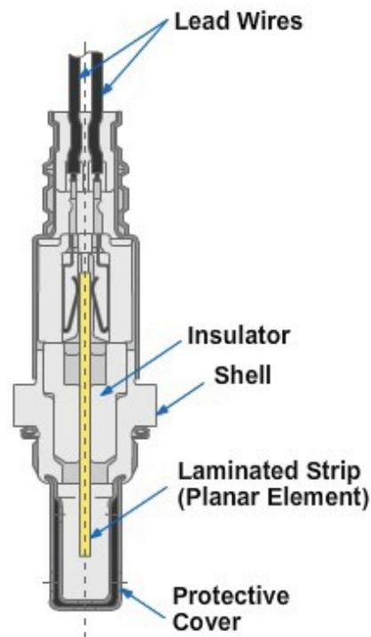
**Figure 5-142 – Cutaway of a planar oxygen.**
