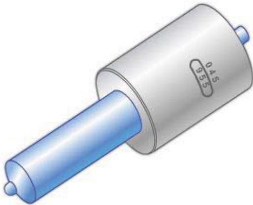
**Figure 5-76 - External view of a multi-orifii injector nozzle.**
