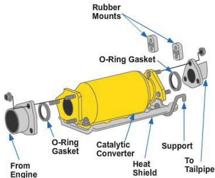
**Figure 5-138 – Exploded view of a catalytic converter installation.**
