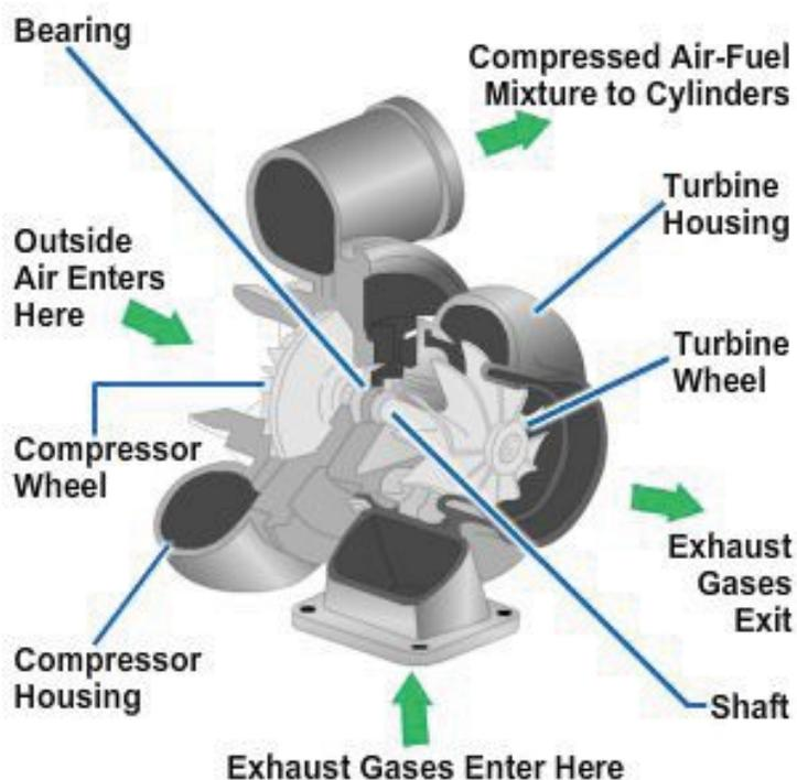
Figure 5-99 – The components of a turbocharger.
