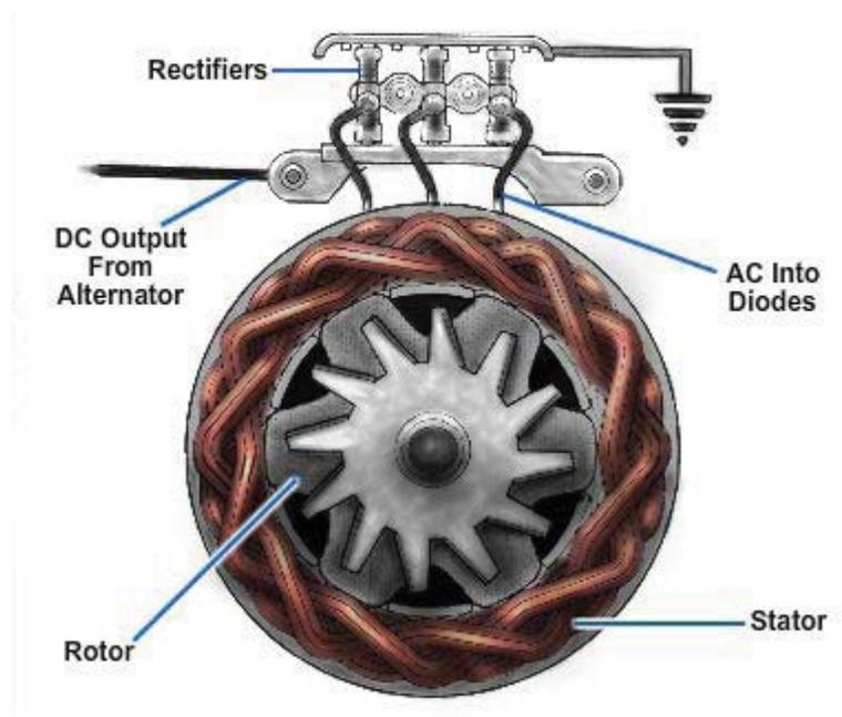
**Figure 6-14 – Converting AC to DC.**
