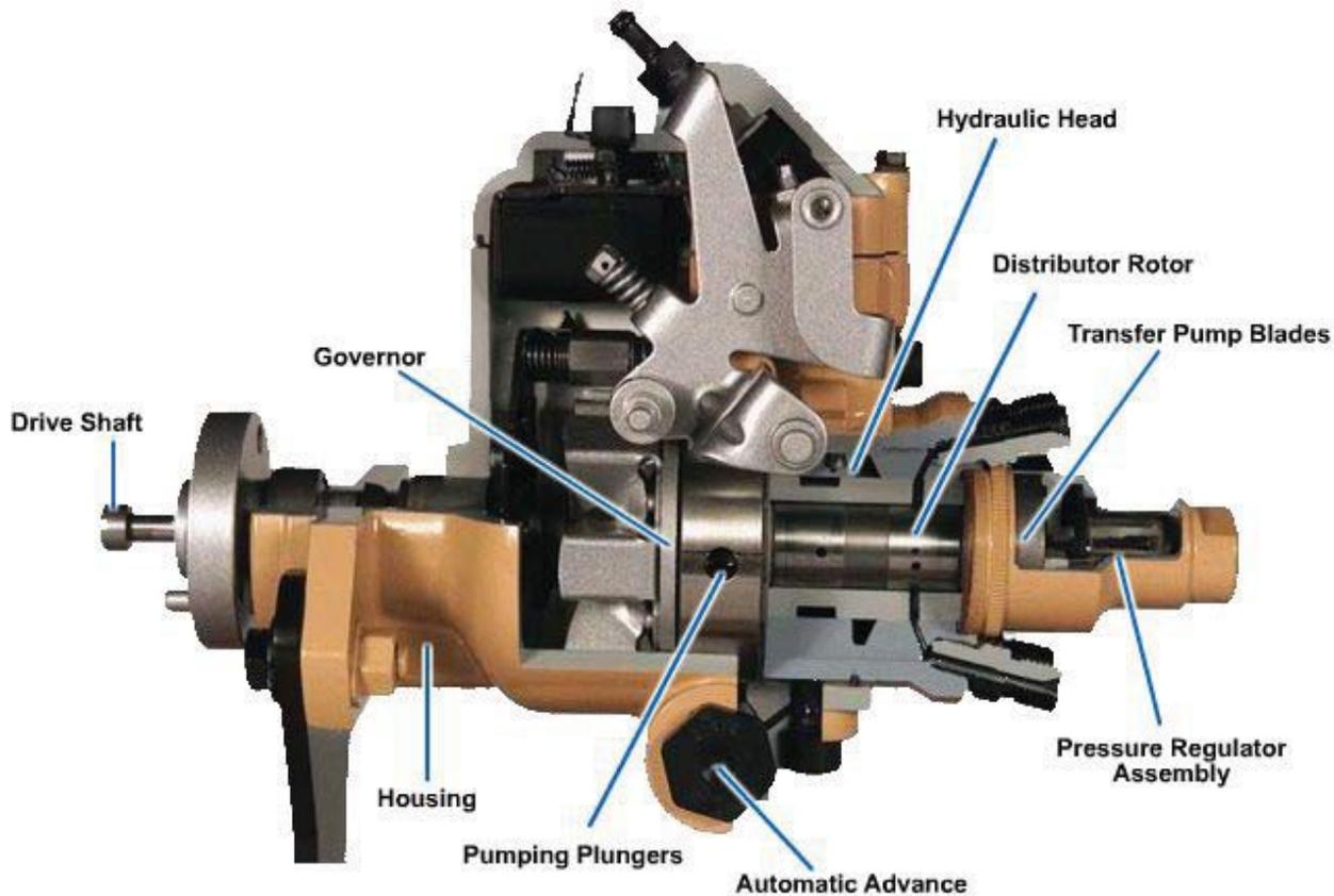
**Figure 5-62 - The Stanadyne DB4 injection pump uses four opposed plungers.**
