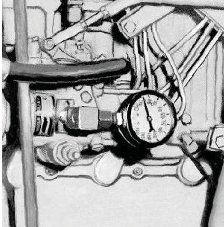
**Figure 5-73 – Testing pump housing pressure.**
