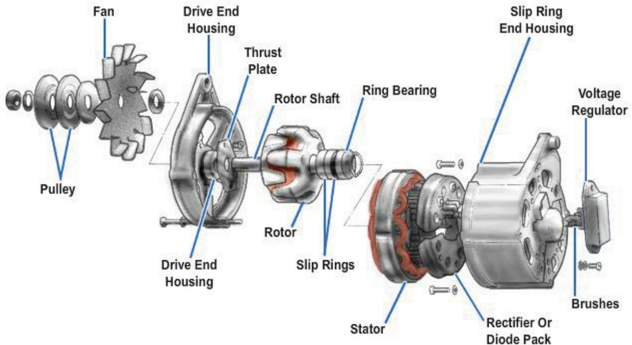
**Figure 6-2 – Exploded view of an alternator.**
