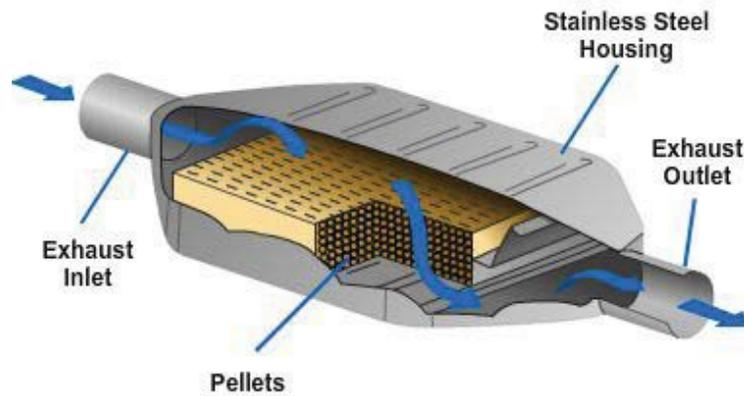
**Figure5-133 – Pellettype catalytic.**
