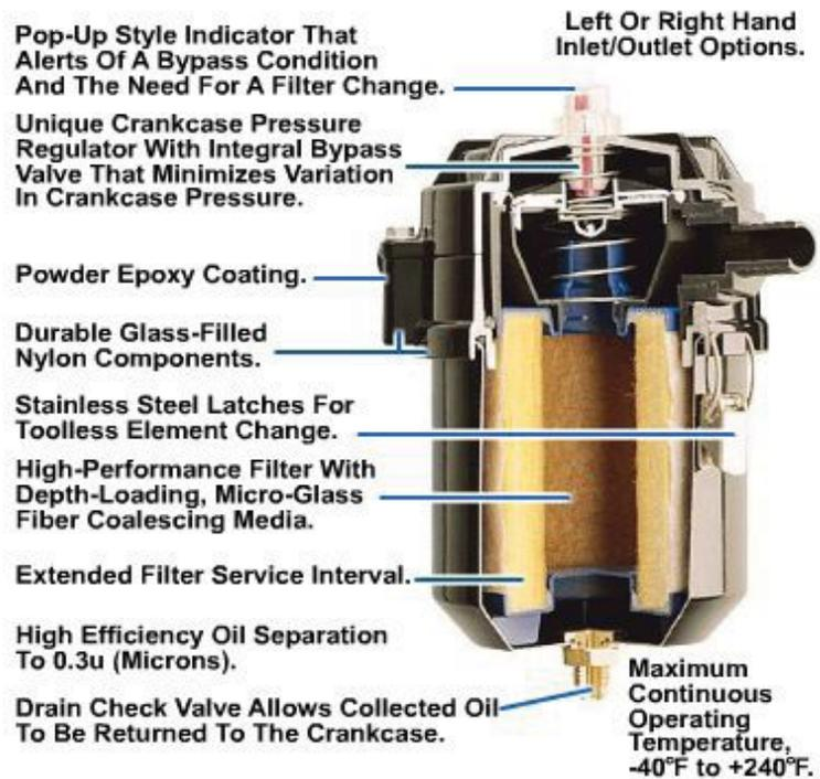
**Figure 5-149 – Cutaway of a Closed Crankcase Ventilation System.**
