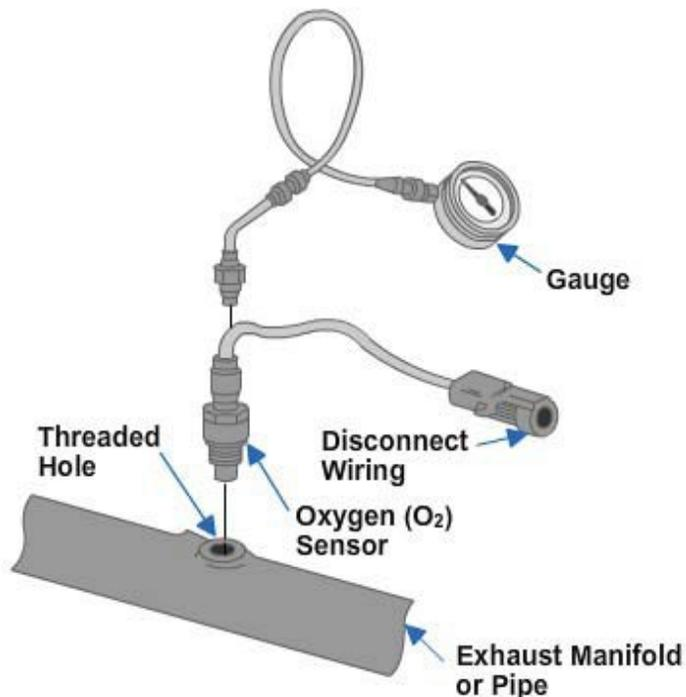
**Figure 5-137 -Testing the exhaust system's back pressure.**
