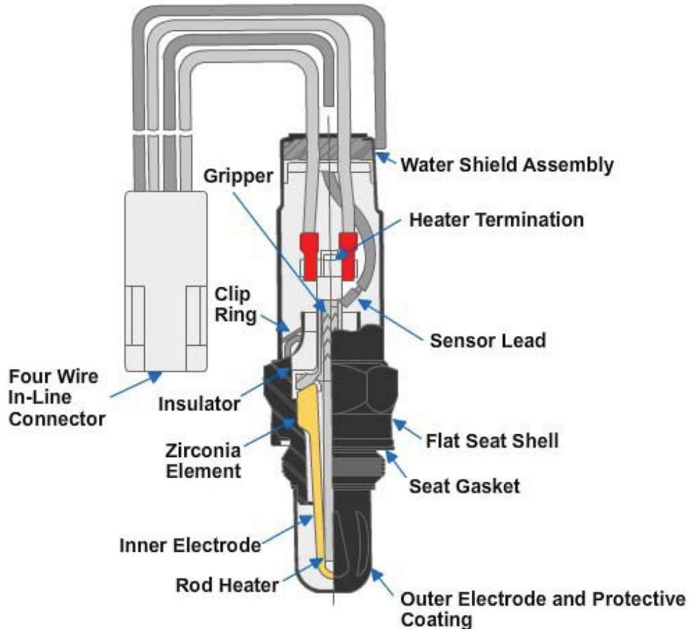
**Figure 5-141 - Cutaway view showing the internal parts of a heated zirconia oxygen sensor.**
