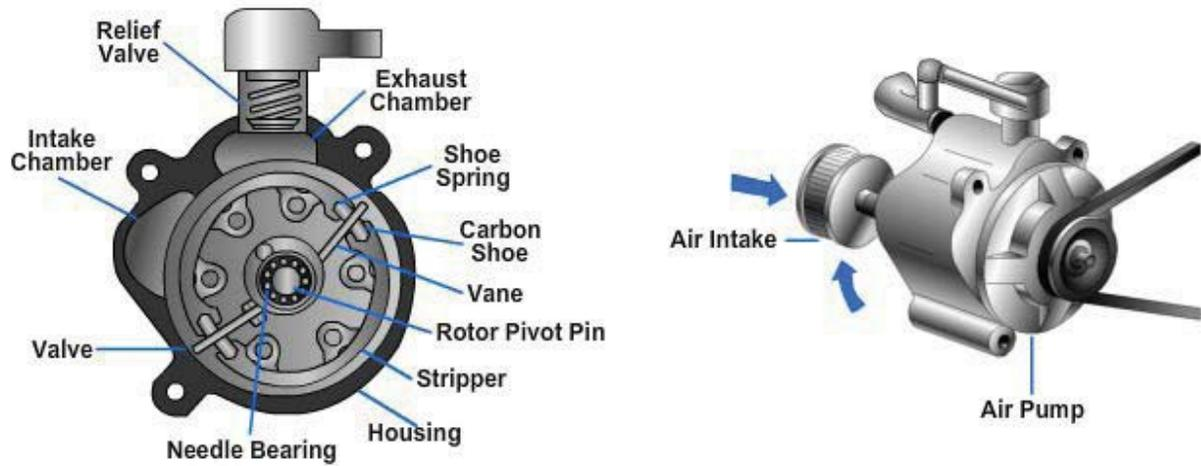
**Figure 5-129 – Rear and side cutaway views of an air pump.**
