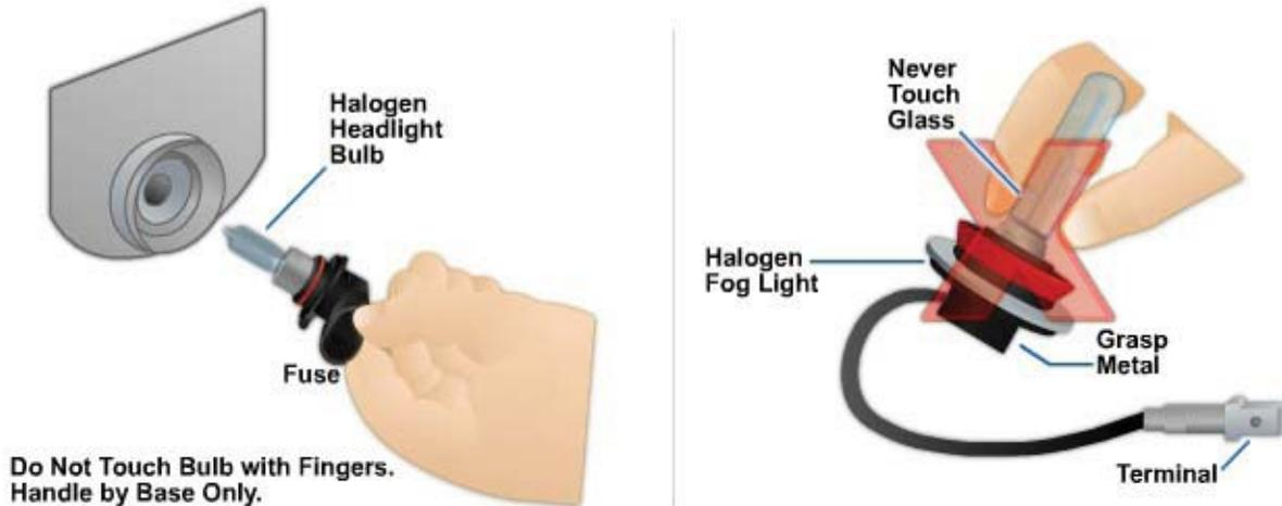
**Figure 6-44 - Handle a high-intensity halogen light properly.**
