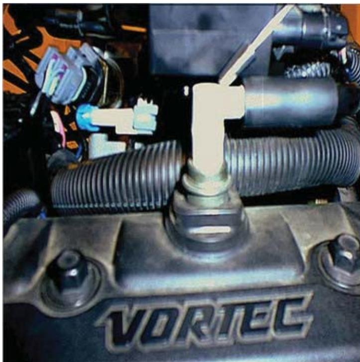
**Figure 5-116 - With the engine running, place your finger over the PCV valve to check for suction.**
