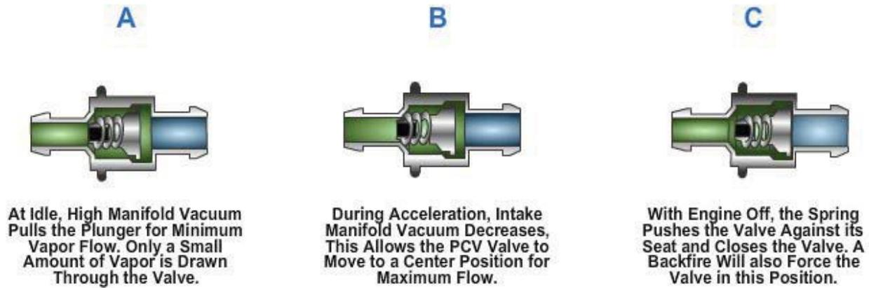
**Figure 5-109 -PCV valve operation under operating conditions.**
