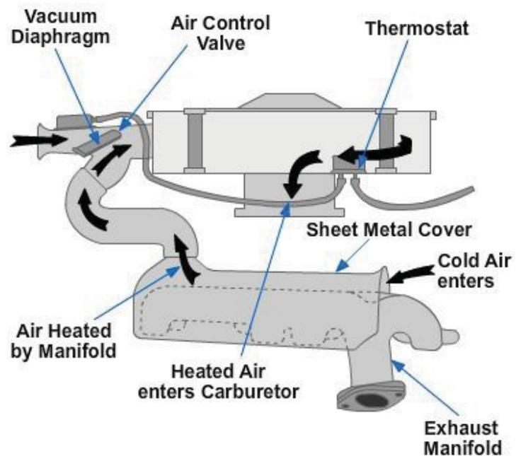
**Figure 5-118 -Thermostatic air cleaner.**
