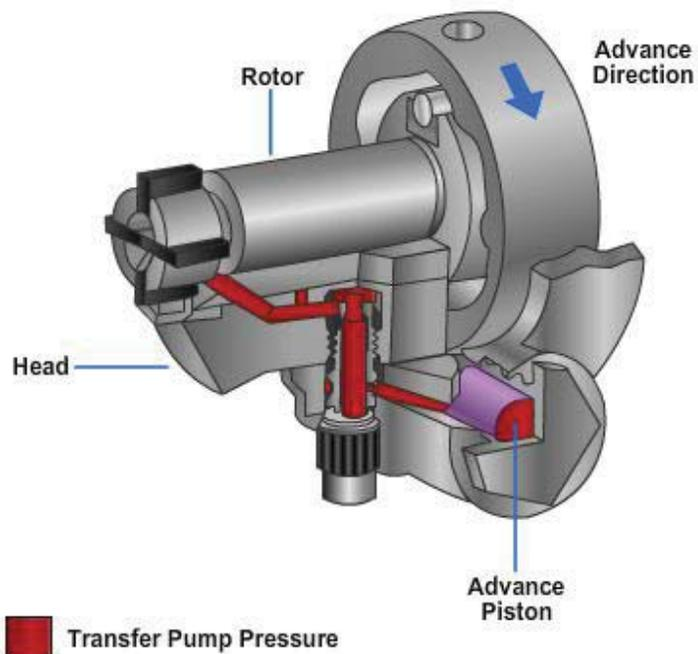
**Figure 5-69 – Operation of the opposed plunger pump automatic mechanism.**
