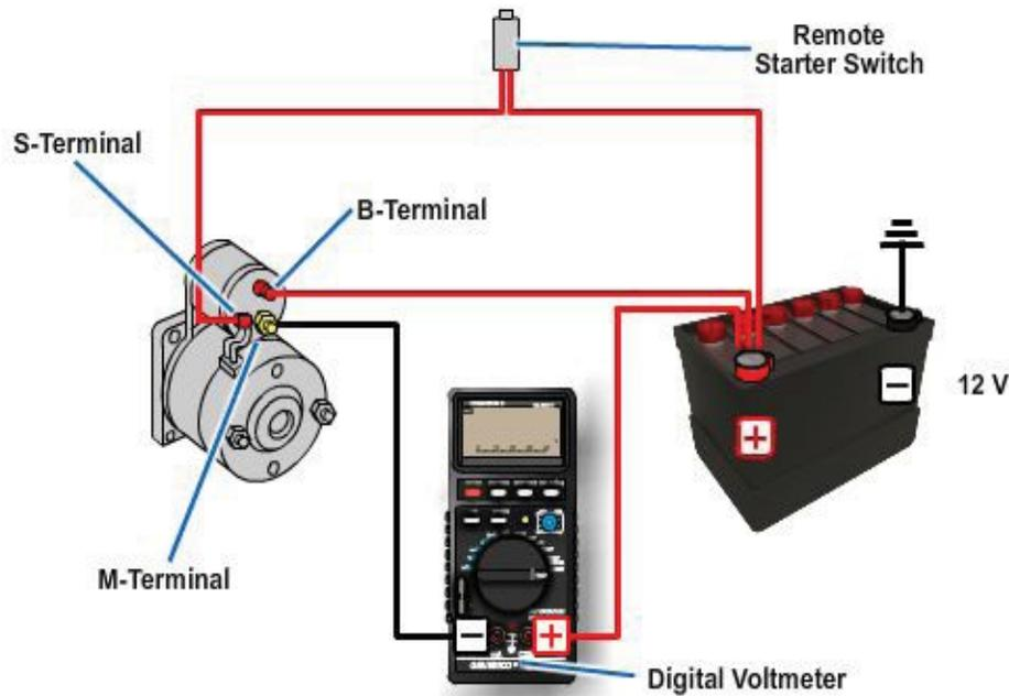
**Figure 6-26- Using a remote starter switch to bypass the control circuit and ignition system.**
