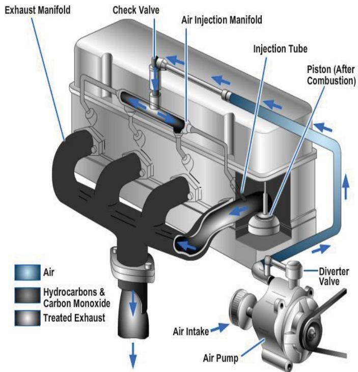
**Figure 5-128 – Diagram illustrating the air injection system.**
