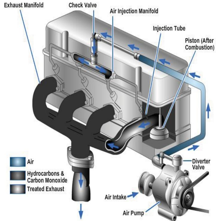
**Figure 5-130 – The basic parts of air injection system.**
