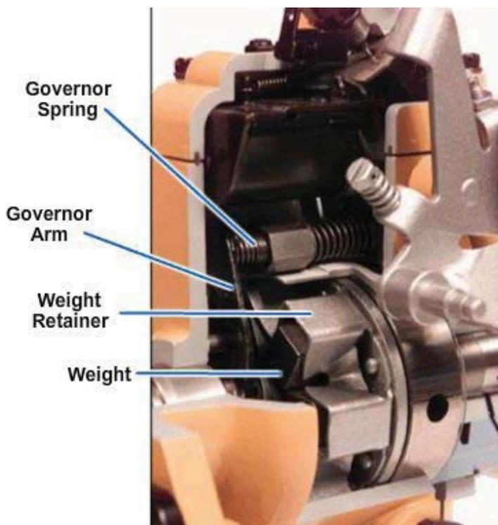
**Figure 5-70 - Components of a mechanical governor.**
