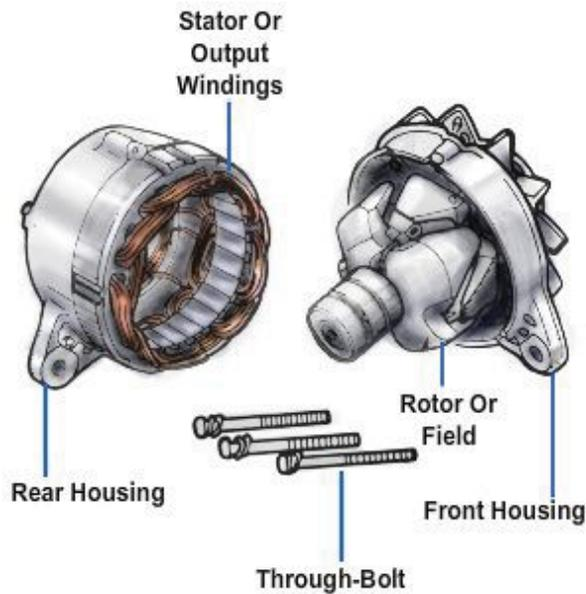
**Figure 6-3 – The rotor mounts inside the stator.**
