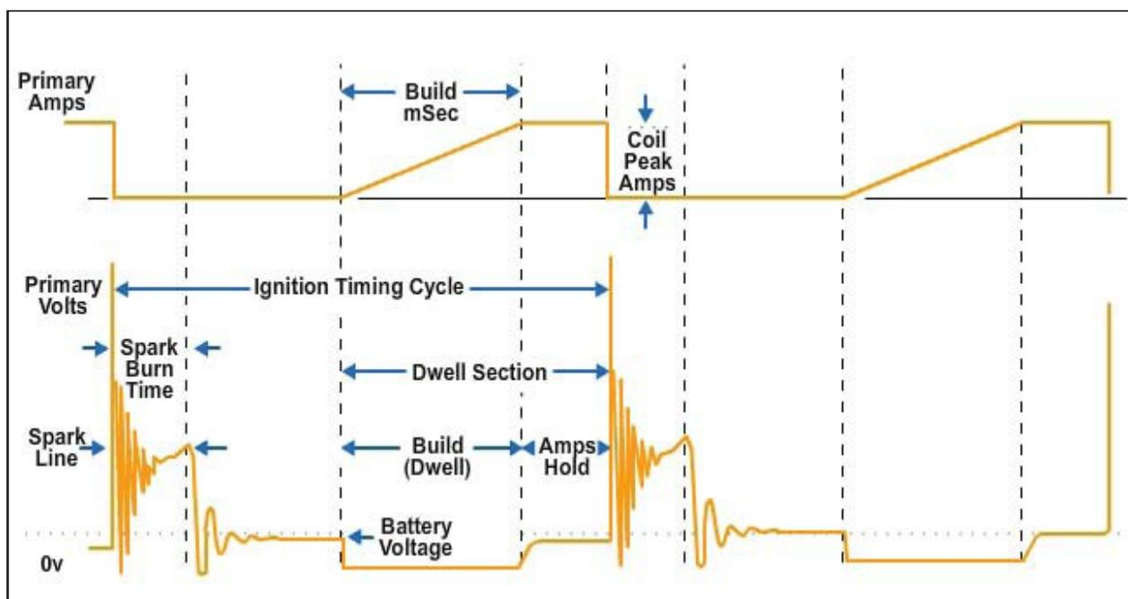
**Figure 6-39 - An illustration showing the primary pattern of a DIS system.**
