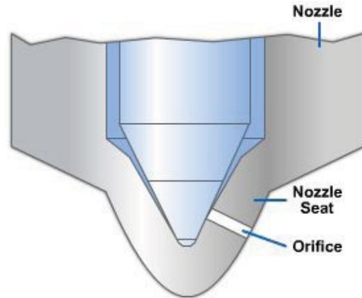
**Figure 5-77 - Sectional view of a valve closes orifice (VCO) nozzle.**
