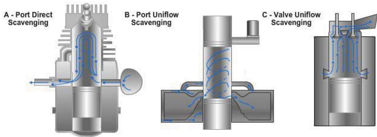
**Figure 5-97 - Methods of scavenging used in diesel engines.**
