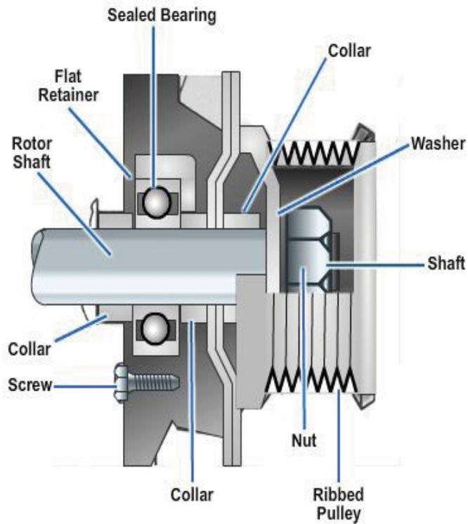
**Figure6-6 – Rotor shaft and bearings.**
