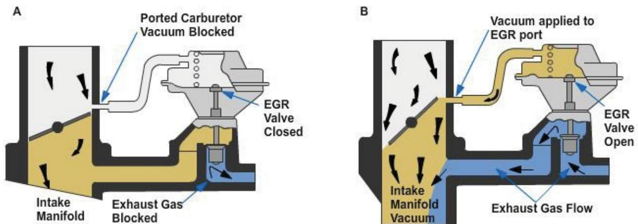
**Figure 5-120 - Basic EGR valve operation.**
