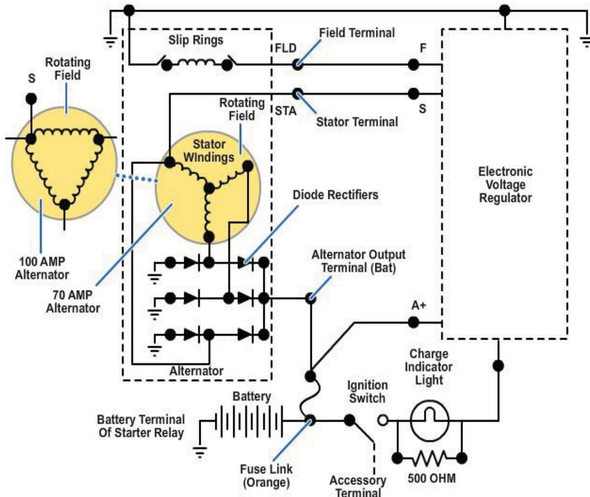
**Figure 6-17 - Schematic with electronic voltage regulator.**
