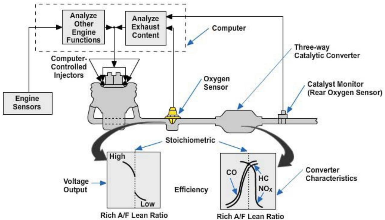
**Figure 5-139 - Diagram oxygen sensor monitoring system.**
