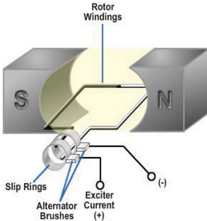
**Figure6-7 – Brushes and sliprings allow current to be fed into rotor windings.**
