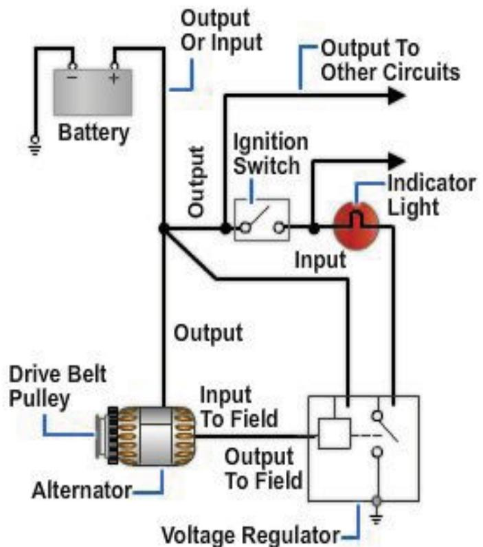
**Figure 6-1 – Schematic of a basic charging circuit.**
