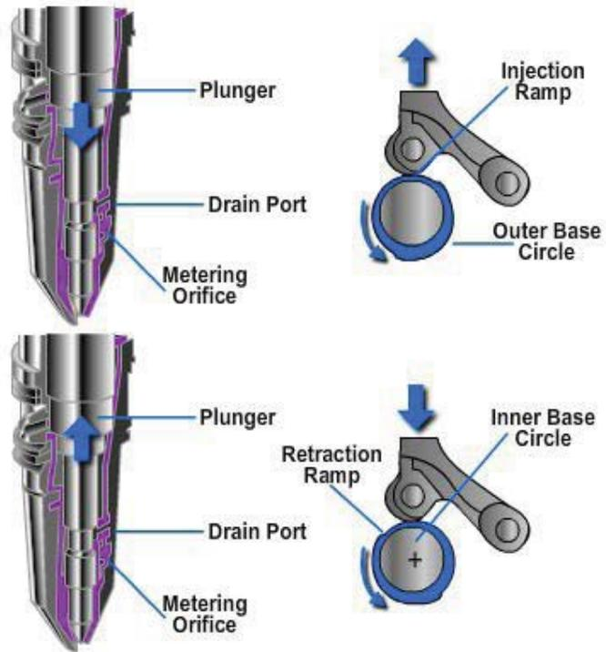
**Figure 5-94 – Metering of fuel in the PTD Top Stop Injector.**
