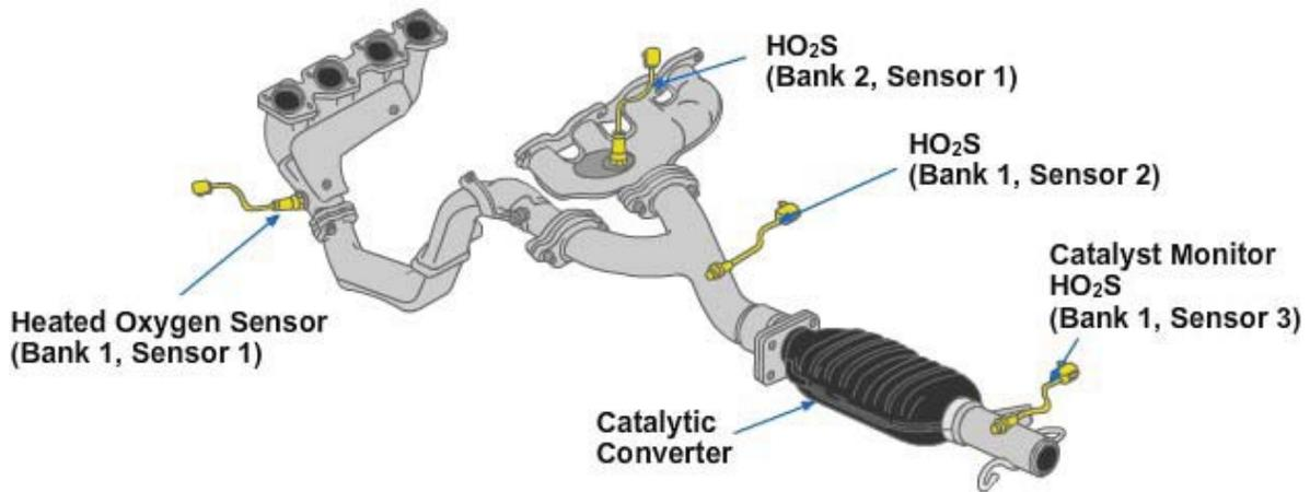
**Figure 5-140 - Oxygen sensor location and identification.**
