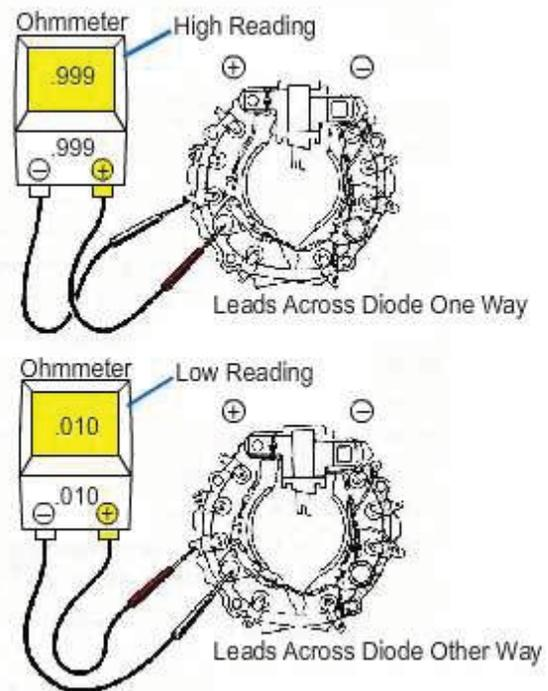
**Figure 6-22 – Testing diodes.**
