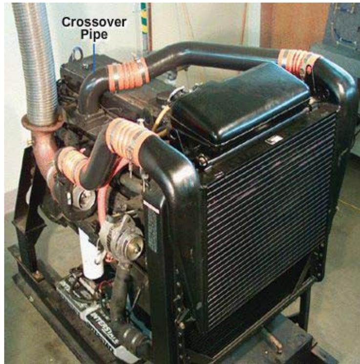
**Figure 5-102 - Typical image showing the location of the crossover pipe or tube.**
