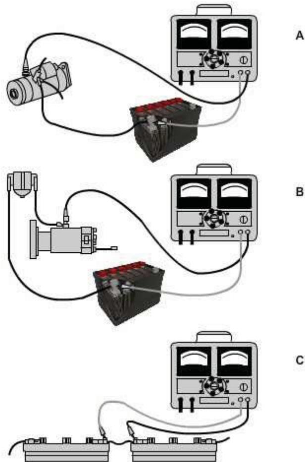
Figure 6-28 - Starter insulated circuit resistance test.
