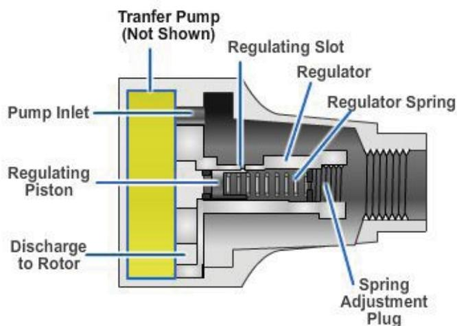
**Figure 5-65 - Pressure regulating valve operation.**
