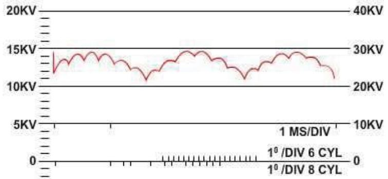
**Figure 6-24 – Poor diode pattern.**
