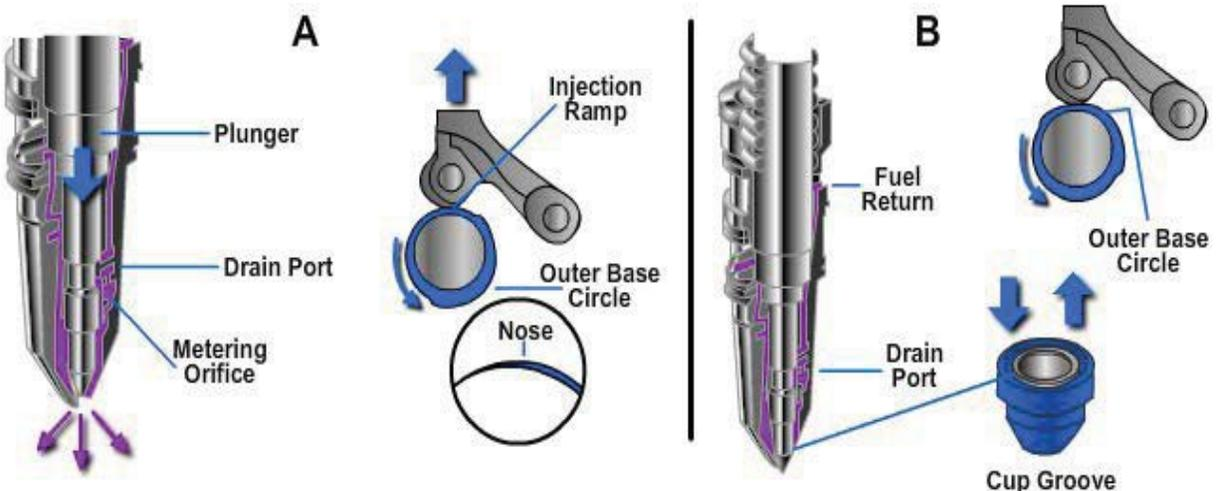
**Figure 5-96 - PTD fuel injector fuel flow.**
