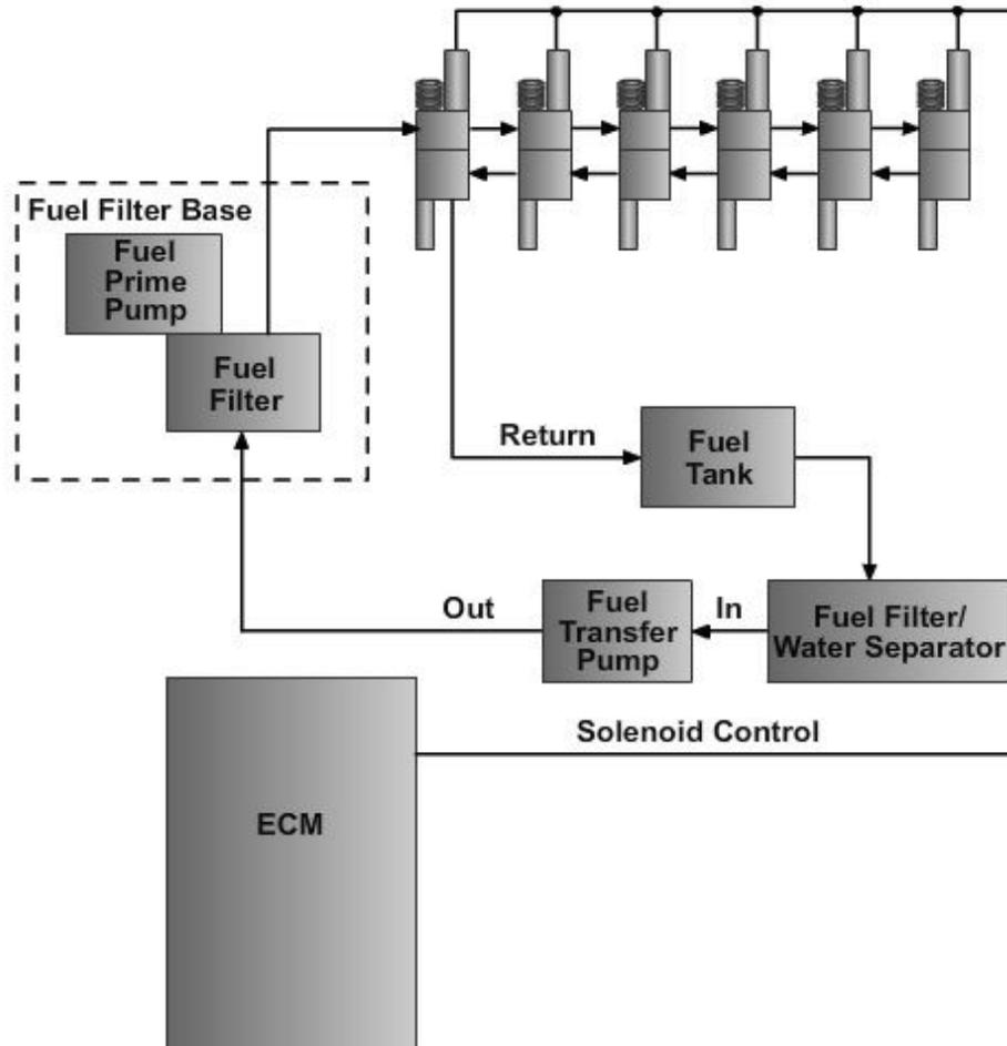
**Figure 5-74 -Example fuel system layout.**
