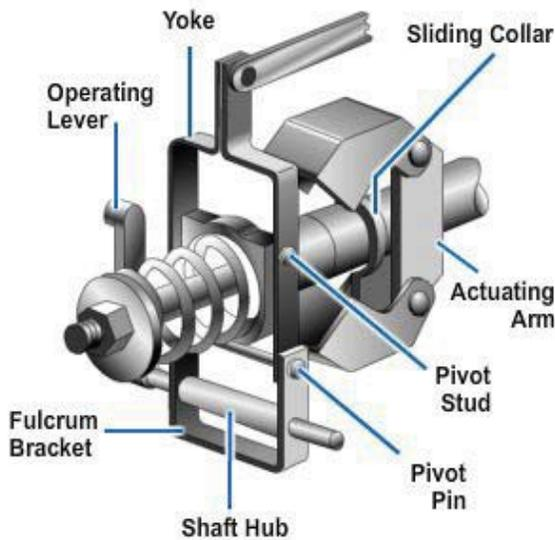
**Figure 5-86 - Components of a Cummins PT fuel pump mechanical flyweight governor.**
