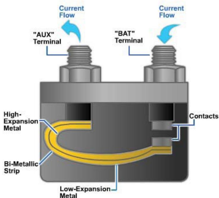
**Figure 6-51 – Cutaway view of a circuit breaker.**
