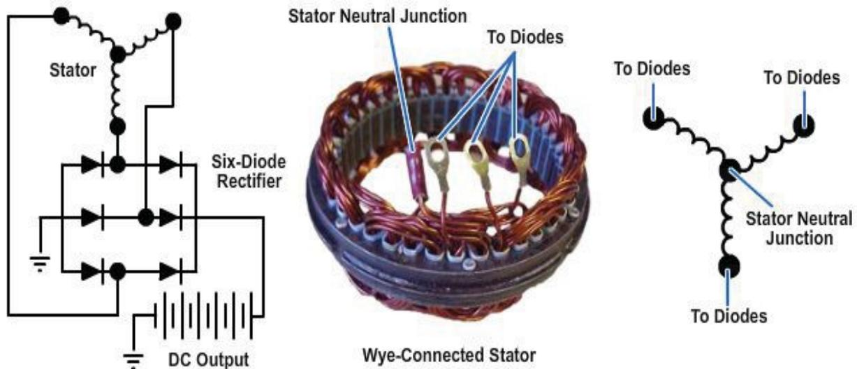
**Figure 6-9 - Y-type stator windings.**
