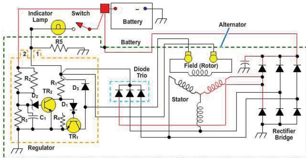
**Figure 6-18 - Wiring diagram of a charging circuit with a diode trio.**
