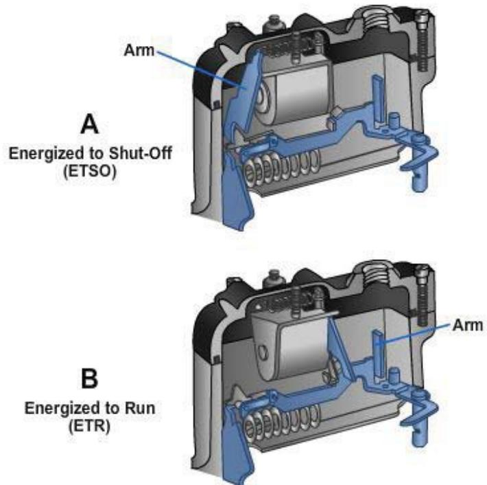
**Figure 5-71 - Electrical solenoid activated fuel shut-off mechanisms. A-Energized-to shut-off. B-Energized-to-run.**
