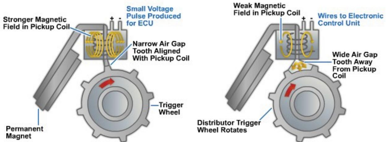
**Figure 6-31 - Electronic ignition system trigger wheel and pickup coil.**
