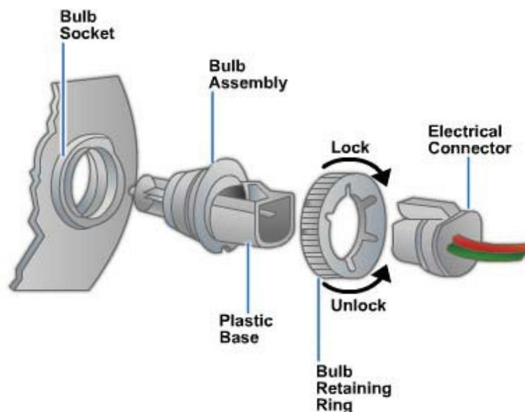
**Figure 6-43 - Typical mounting assembly of a replaceable halogen light.**
