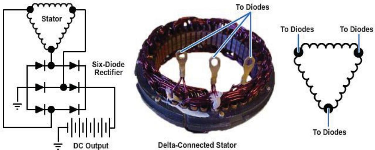
**Figure 6-10 - Delta-type stator windings.**
