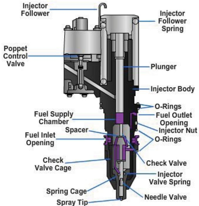
**Figure 5-80 – Cutaway view of a fuel flow unit injector.**
