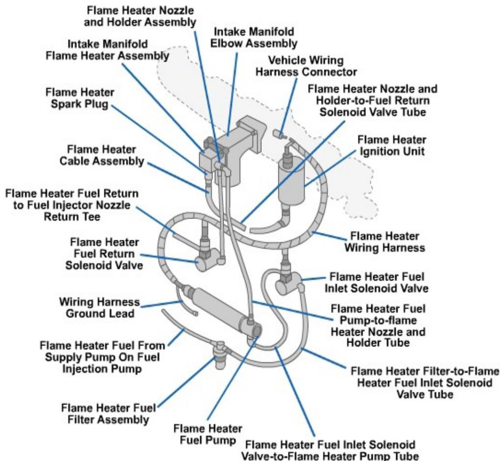
**Figure 5-105-Manifold flame heater system.**
