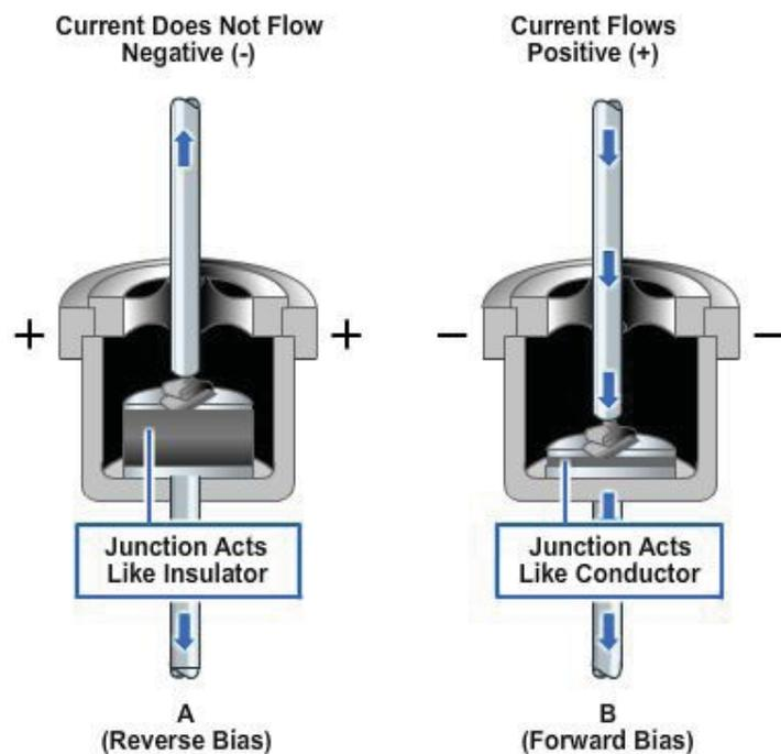
**Figure 6-15 – Cutaway view showing diode operation.**
