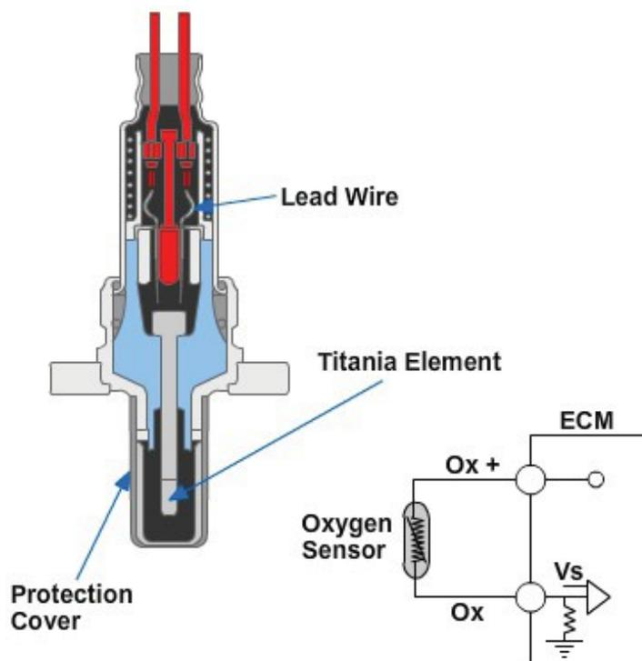
**Figure 5-143 – A Cutaway view of a titania oxygen sensor and basic circuit.**
