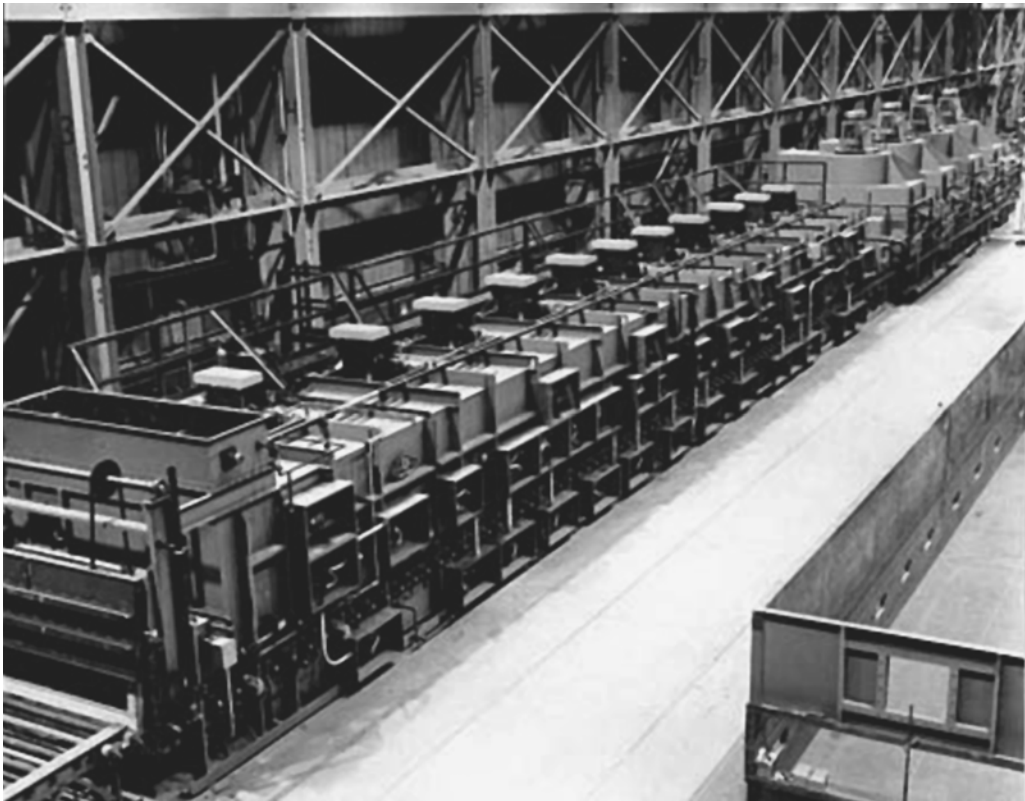
FIGURE 10.21 Photograph of a roller hearth furnace. (Courtesy of Electric Furnace, Salem, OH.)
