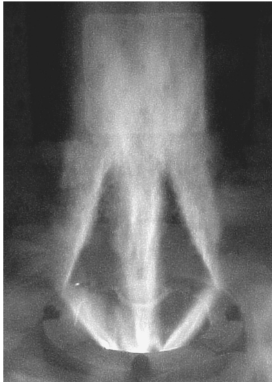
FIGURE 8.3 Example of a low-luminosity gas flame. (Courtesy of John Zink Co. LLC, Tulsa, OK.)
