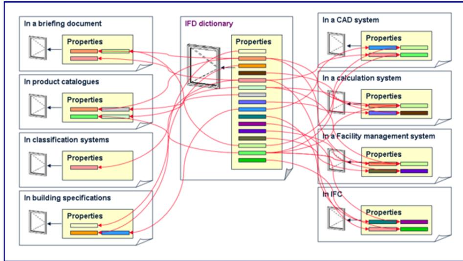
**Figure 2.5-3 – IFD as a Mapping Mechanism:** courtesy Lars Bjørkhaug and Håvard Bell, *IFD in a Nutshell*, IFD Developers wiki, [www.IFD-library.org](http://www.IFD-library.org)
