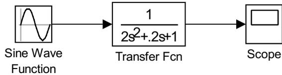
Figure 4.6: The use of the **Transfer Fcn** Block with a **Sine Wave** input and output to a **Scope**.
