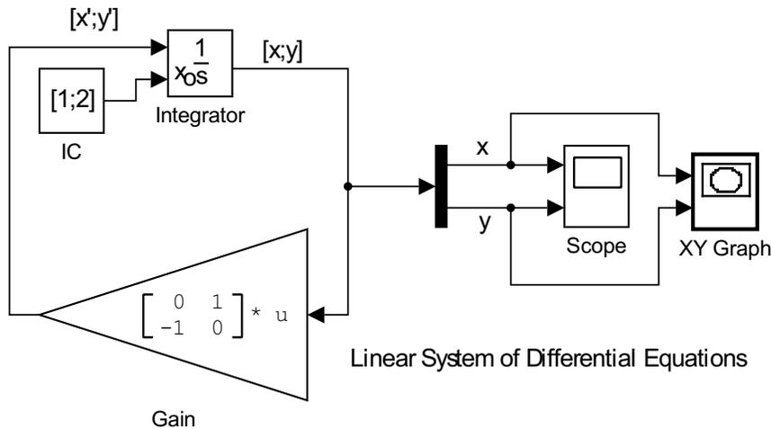
Figure 5.4: Linear system using matrix operation.
