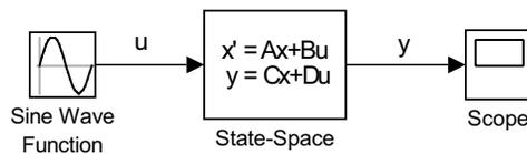
Figure 4.2: The use of the **State Space Block** displaying a **Sine Wave** input and output to a **Scope**.
