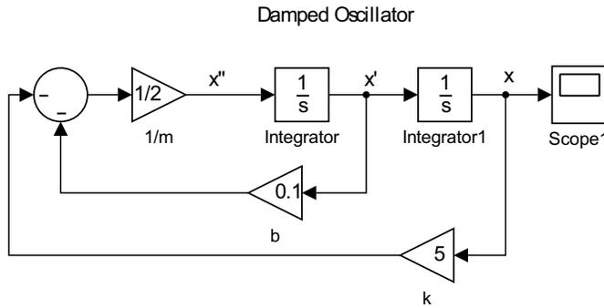
Figure 3.9: A model for damped simple harmonic motion,  $m\ddot{x} + b\dot{x} + kx = 0$ .
