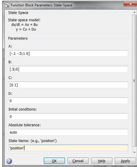
Figure 4.3: State space block parameters.
