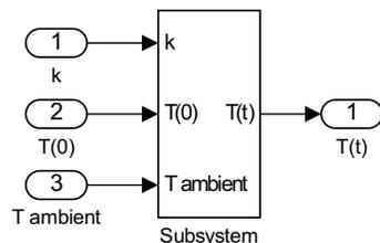
Figure 2.6: Subsystem for Newton's Law of Cooling,  $T' = -k(T - T_a)$ ,  $T(0) = T_0$ .
