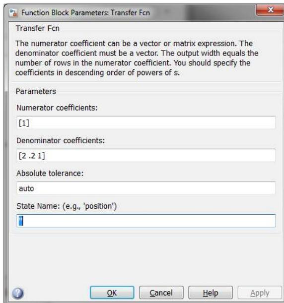
Figure 4.7: Block parameter display for the Transfer Fcn block.
