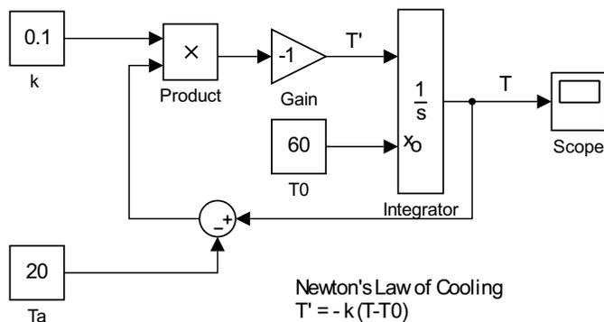
Figure 2.3: Simulation model for Newton's Law of Cooling,  $T' = -k(T - T_a)$ ,  $T(0) = T_0$ . Here we set  $k = 0.1 \text{ s}^{-1}$ ,  $T_a = 20^\circ\text{C}$ , and  $T_0 = 60^\circ\text{C}$ .
