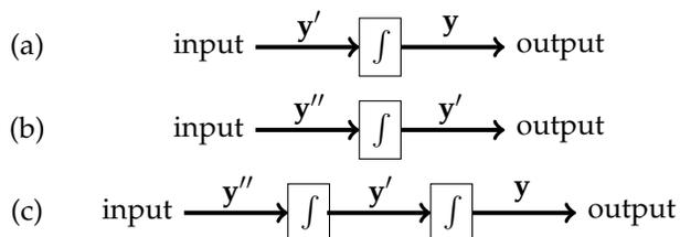
Figure 3.1: Basic schemes for using Integrator blocks for solving second order differential equations.
