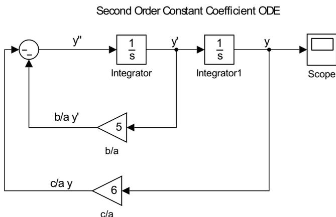
Figure 3.3: Model for the second order constant coefficient ODE  $y'' + 5y' + 6y = 0$ .
