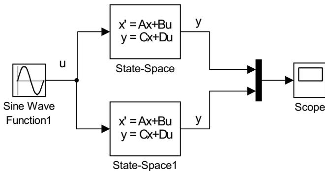
Figure 4.5: The use of the **State Space Block** displaying a Sine Wave input and output to a **Scope**. The **Mux** block (from Signal Routing) is used to feed solutions from two systems using different initial conditions.
