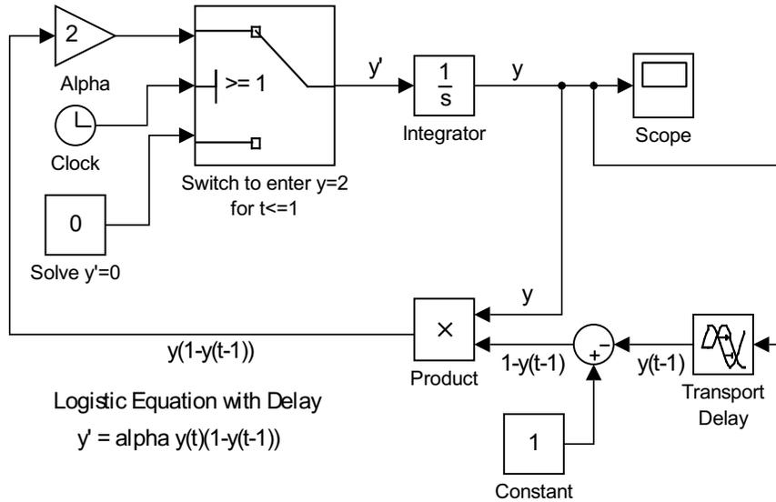
Figure 2.16: Model for the logistic equation with delay,  $y' = ry(t)(1 - y(t-1))$ .
