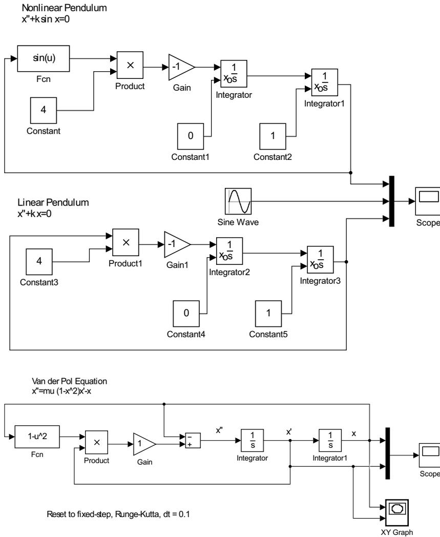
Figure 5.6: Linear and nonlinear pendulum.
