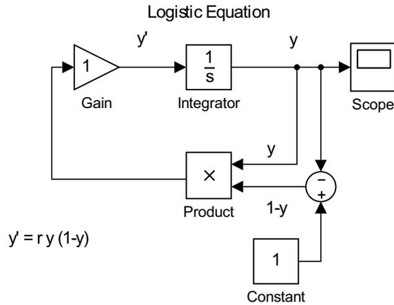
Figure 2.14: Simulink model for the logistic equation,  $y' = ry(1 - y)$ .
