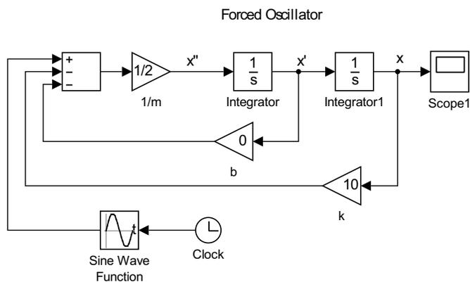
Figure 3.12: A model for forced simple harmonic motion,  $m\ddot{x} + kx = \sin \omega t$ .
