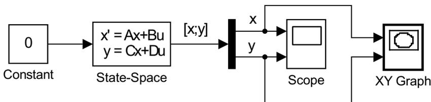
Figure 5.5: Linear system using matrix operation.
