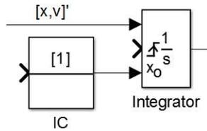
Figure 3.24: Modified Integrator and IC blocks.
