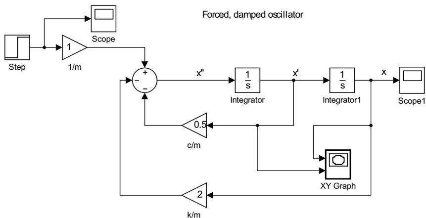
Figure 3.16: Forced, damped oscillator.
