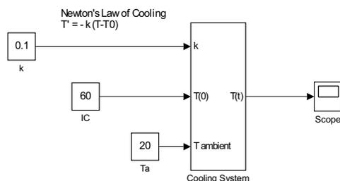
Figure 2.7: Using a user-created subsystem for Newton's Law of Cooling.
