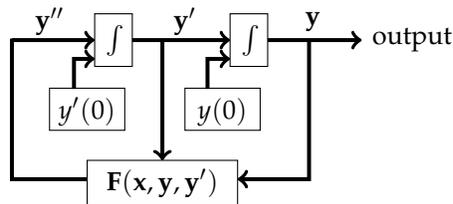
Figure 3.2: This is a general schematic for solving an initial value problem of the form  $y'' = F(x, y, y')$ ,  $y(0) = y_0$ ,  $y'(0) = v_0$ .
