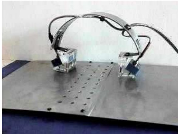
b. double spring “hopping probe” use for the inspection of a lap splice joint
