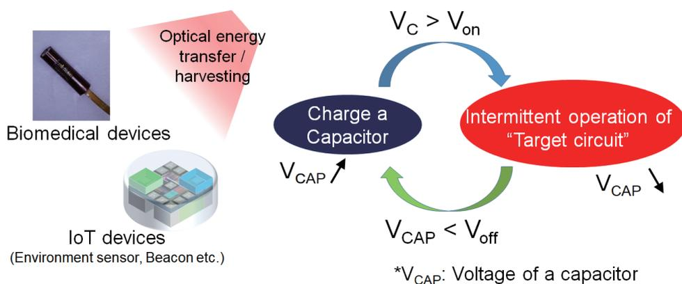
Fig. 1. (Color online) Concept of the CMOS-controlled PV power transfer scheme.
