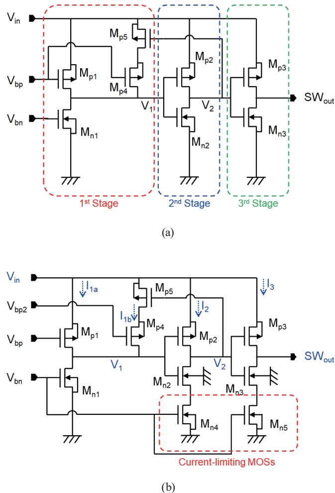
Fig. 3. (Color online) (a) Basic<sup>(15)</sup> and (b) improved<sup>(18)</sup> circuits of the CMOS voltage detector circuit.
