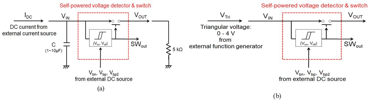
Fig. 9. (Color online) Experimental setups for measurements of (a) minimum operating current and (b)  $V_{on}$  and  $V_{off}$ .
