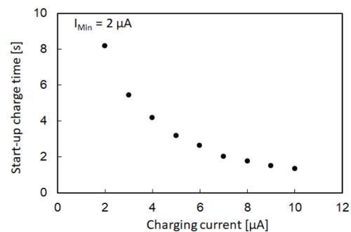
Fig. 5. Start-up charging time as a function of charging current.
