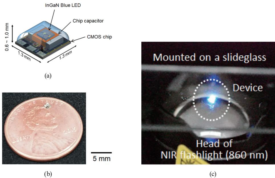
Fig. 12. (Color online) (a) Structure and (b) outlook of a batteryless implantable optogenetic neural stimulator based on the proposed CMOS-based optical power transfer platform. (c) A photograph of the device under operation.<sup>(18)</sup>
