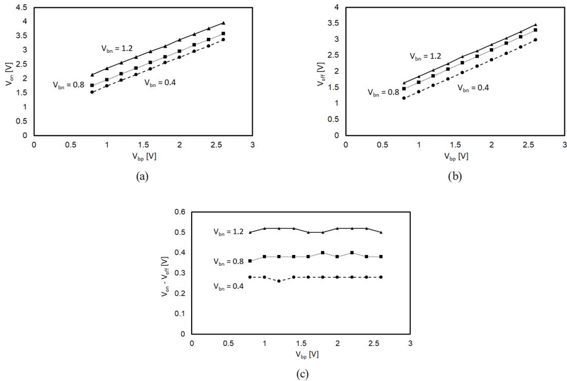
Fig. 6. Threshold voltages (a)  $V_{on}$  and (b)  $V_{off}$ , and (c) hysteresis  $V_{on} - V_{off}$  as functions of  $V_{on}$  and  $V_{bp}$ .
