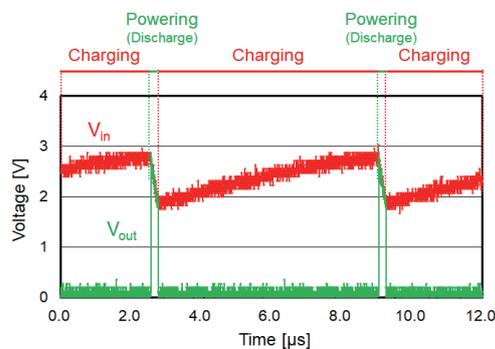
Fig. 4. (Color online) Experimental trace showing the charge and operation cycle.
