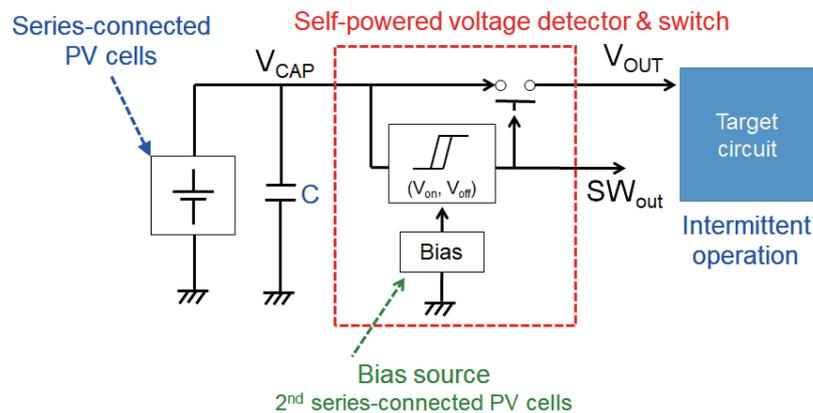
Fig. 2. (Color online) Block diagram of the CMOS-controlled PV power transfer platform.
