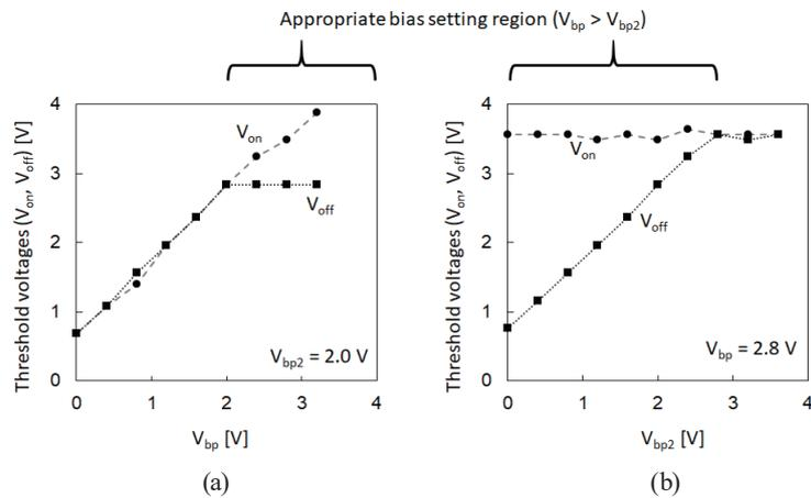
Fig. 11.  $V_{on}$  and  $V_{off}$  as functions of (a)  $V_{bp}$  and (b)  $V_{bp2}$ .  $V_{bp2}$  was fixed at 2.0 V for (a) and  $V_{bp}$  at 2.8 V for (b).
