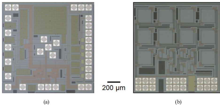
Fig. 8. (Color online) Layouts of the CMOS chips for (a) Chip-A, evaluation of the improved voltage monitoring circuit and (b) Chip-B, functional demonstration.
