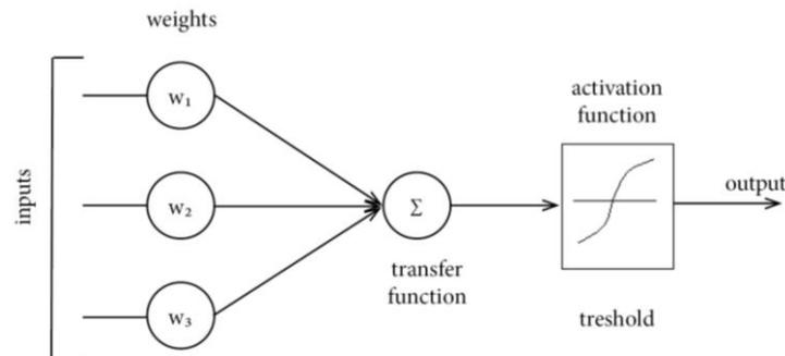
Fig.6 Basic elements of an artificial neuron. [16]
