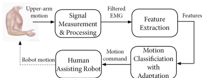
Fig. 11 EMG-based upper arm robot control system
