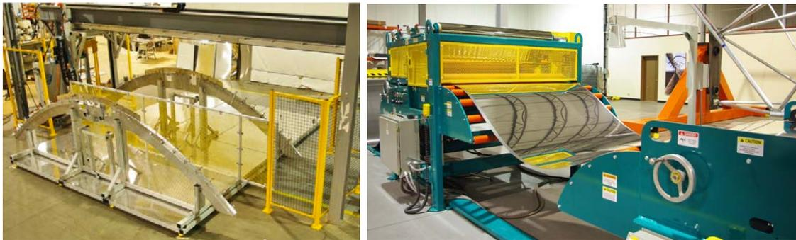
**Figure 28. SkyFuel aluminum parabolic rib assembly machine and Reflectech Plus manufacturing**
