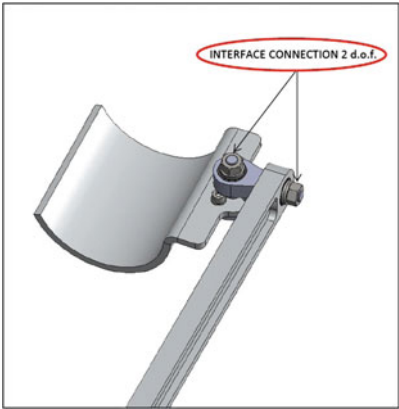
Fig. 3 Detailed view of the two revolute joints of the interface connection
