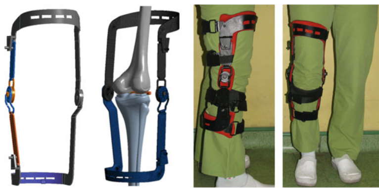
Fig. 13 Virtual model an phisical prototype of the proposed orthotic device
