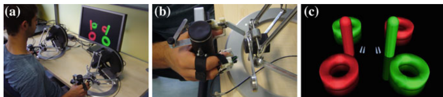
Fig. 3 Experimental setup. a General overview of the setup. b Detail of one hand wearing the cutaneous devices. c Virtual environment with surgical pliers
