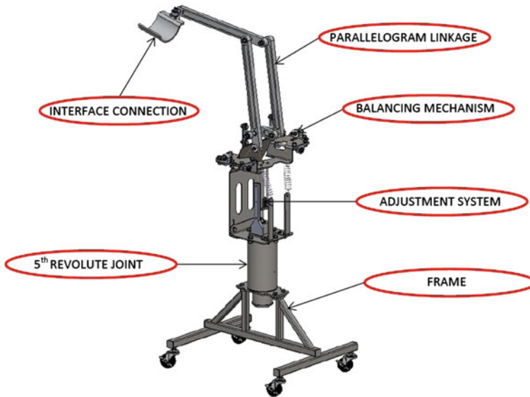
Fig. 2 3D CAD model and subcomponent labels
