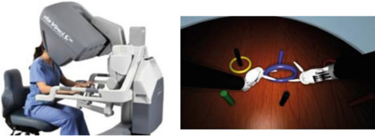
Fig. 1 The da Vinci Skills Simulator contains a variety of scenarios ( right ) designed to give surgeons the opportunity to improve their proficiency with the da Vinci console controls ( left )
