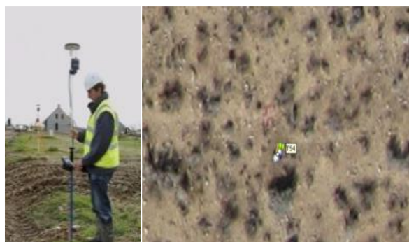
Step3: Operation of making BMs and signalized GCPs based on network design and their positioning by GPS.
