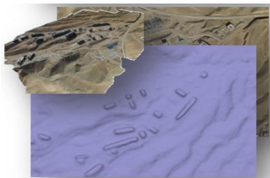
Step7: Initial DSM generation for ortho-image-mosaic and 3D textured realistic model generation.
