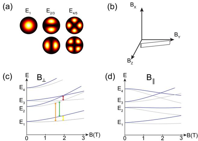
**Figure 4.** (a) Probability density of the first five sub-bands of a cylindrical nanowire. (b) Orientation of the nanowire with respect to the magnetic field axes. (c,d) Numerical simulations of the sub-band dispersion of a InSb nanowire in perpendicular (c) and parallel (d) magnetic field. The levels  $E_{n\uparrow}$  are drawn in gray and  $E_{n\downarrow}$  in blue.
