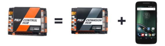
The Control Hub, which has its built-in Android device connected directly to the Expansion Hub using an internal serial bus, eliminates the need for an external USB connection between the Android Robot Controller and the I/O module.
