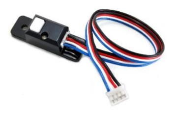
2. Plug the other end of the 4-pin JST PH cable to digital I/O port labeled "0-1" on the Hub.
