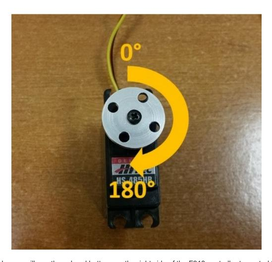
In this example, you will use the colored buttons on the right side of the F310 controller to control the position of the servo. Initially, the op mode will move the servo to the midway position (90 degrees of its 180-degree range). Pushing the yellow "Y" button will move the servo to the zero-degree position. Pushing the blue "X" button or the red "B" button will move the servo to the 90-degree position. Pushing the green "A" button will move the servo to the 180-degree position.
