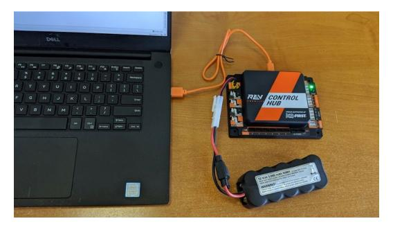
When using the Control Hub, please make sure you use the Type C port (and not the USB Mini port) to connect the Control Hub to your development laptop.
