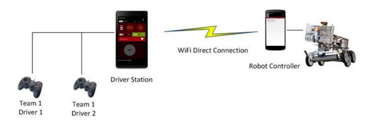
One Android device is mounted onto the robot and is called the *Robot Controller*. The Robot Controller acts as the "brains" of the robot. It does all of the thinking for the robot and tells the robot what to do. It consists of an Android device running an FTC Robot Controller app. There are two hardware options currently being used: REV Robotics Expansion Hub or the REV Robotics Control Hub.
