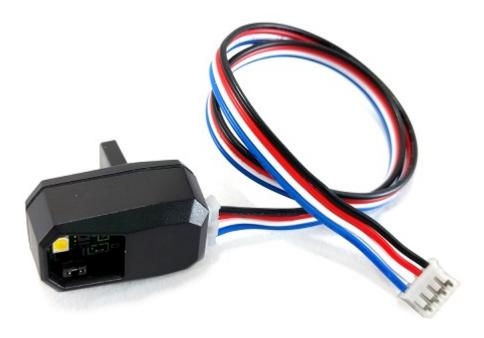
2. Plug the other end of the 4-pin JST PH cable to the I2C port labeled "0" on the Hub.
