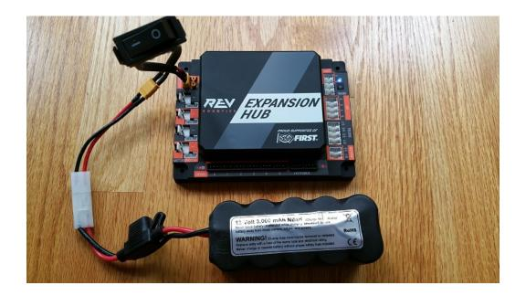
6. Turn off the switch and verify that the Hub is off. Note that the Hub's LED should not be illuminated.
