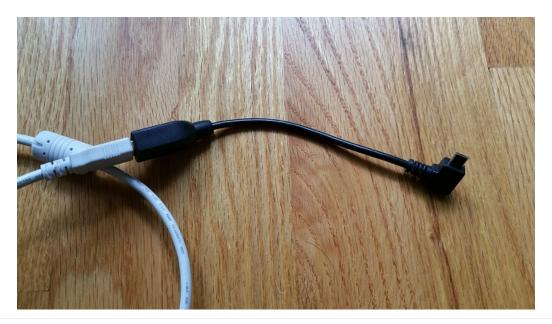
4. Verify that your Robot Controller smartphone is powered on and unlocked. Plug in the USB Micro OTG adapter into the OTG port of the Robot Controller phone.
