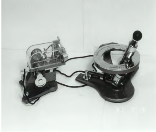
A.S. Aloe Co. Pneumatic Micro-manipulator de Fonbrune, Series A, No. 119 c. 1942
