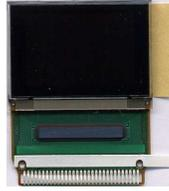
Fig. 1.4: Sample of a commercial OLED device with integrated driver chip
