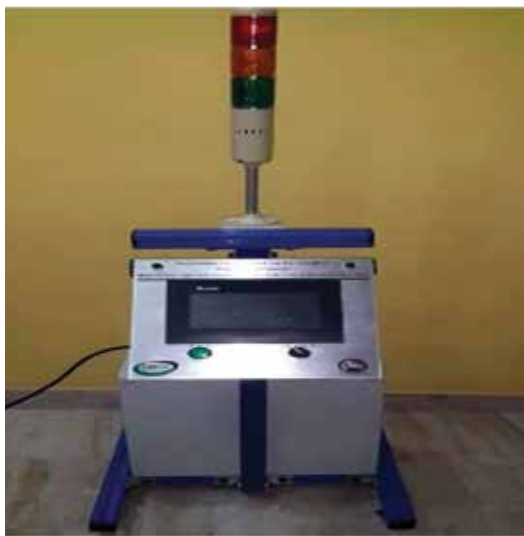
Fool proof centralized voting machine using automation system
