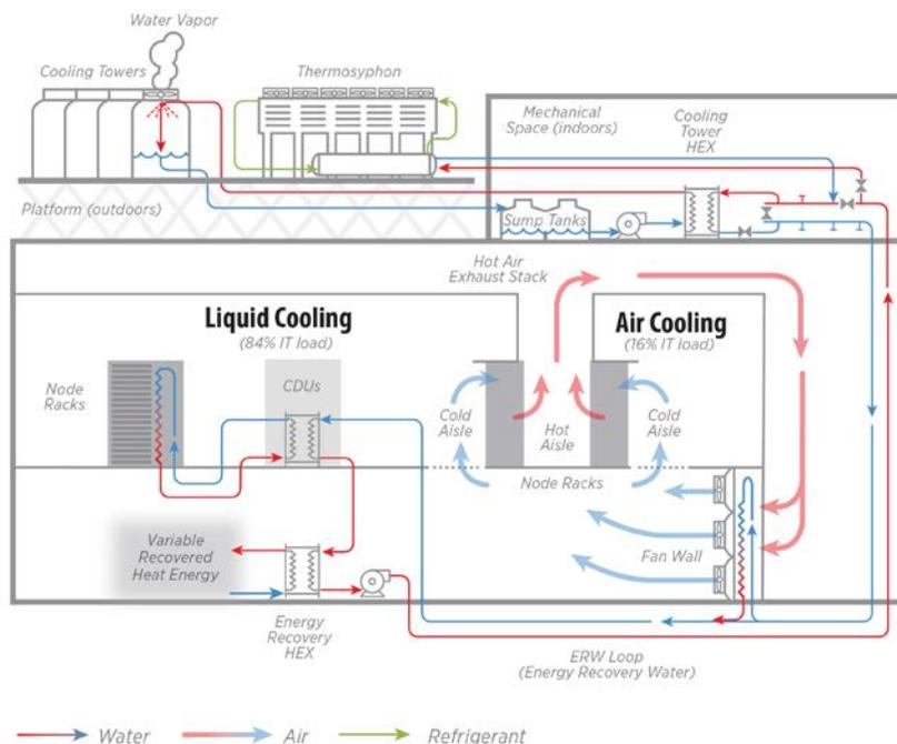
**Figure 2** Cooling system schematic for the HPC data center located in the ESIF.
