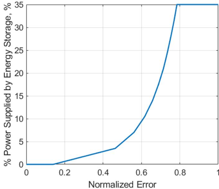
**Fig. 13 Energy storage device power fraction schedule**
