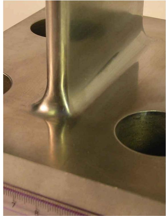
**Figure 7.10:** Shape optimised trailing edge transition specimen.
