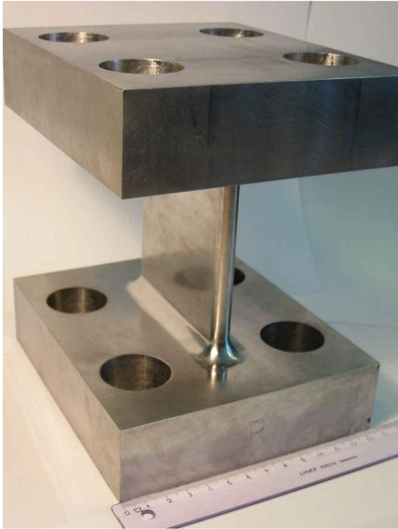
**Figure 7.9:** Circular-shaped trailing edge transition specimen.
