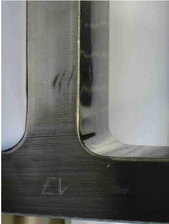
**Figure 7.1:** T-joint specimen. Standard quarter-circular transition.
