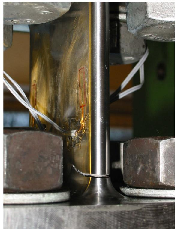
**Figure 7.14:** Trailing edge test specimen RI. Failure due to crack growing from stress concentration.
