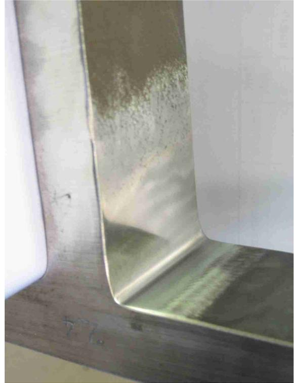
**Figure 7.2:** T-joint specimen. Shape optimised transition (case D).
