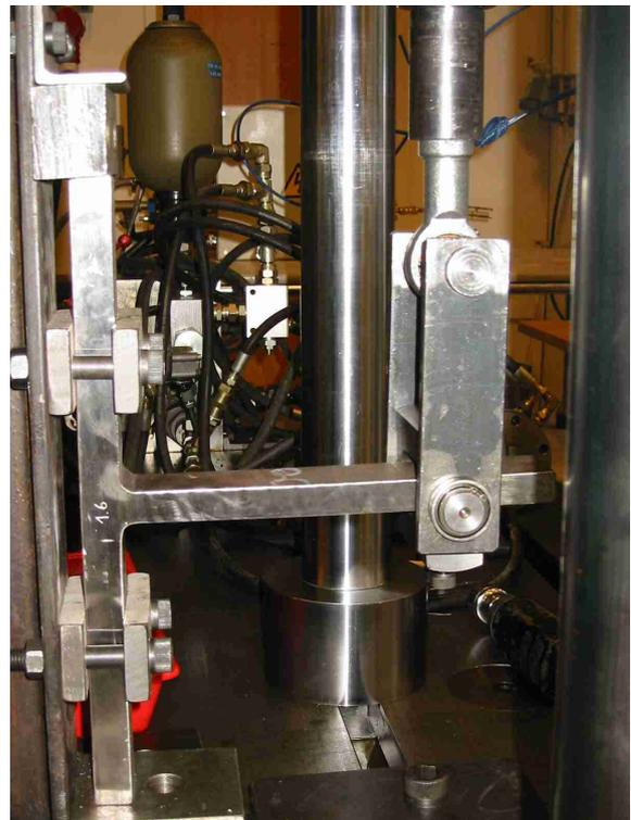
**Figure 7.4:** T-joint test mounted.
