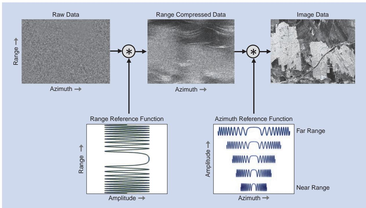
**FIGURE 3.** Summary of SAR processing steps where the range compressed data result from a convolution of the raw data with the range reference function. In a second step the azimuth compression is performed through a convolution with the azimuth reference function, which changes from near to far range. Here the “\*” represents the convolution operation.
