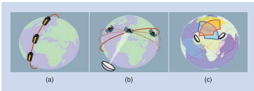
**FIGURE 30.** Concepts for a future constellation of radar satellites for quasi-continuous monitoring of the Earth. (a) Low Earth Orbit (LEO) satellites, (b) Geostationary Earth Orbit (GEO) transmitter with a large reflector and LEO receivers, and (c) Medium Earth Orbit (MEO) satellites using a large reflector.
