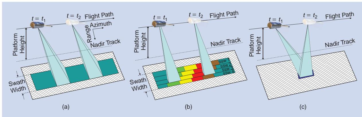
**FIGURE 6.** Illustration of different SAR operation modes which are used to increase the swath width (ScanSAR) or improve the azimuth resolution (Spotlight) compared to the Stripmap mode. (a) Stripmap. (b) ScanSAR. (c) Spotlight.
