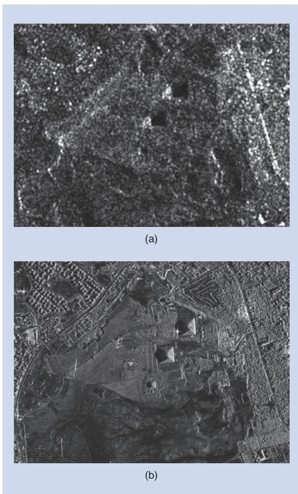
**FIGURE 1.** Comparison of a SAR image corresponding to the state of the art during the 90s [(a) ca. 20 m resolution, C-band, radar illumination from the left] and the current generation of SAR satellites available since 2007 [(b) 1 m resolution, X-band, radar illumination from the right]. The images show the pyramids of Giza, Egypt.
