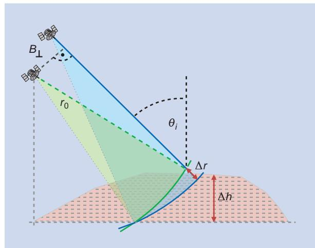
**FIGURE 11.** Across-track SAR interferometry employs antennas that move on parallel but mutually displaced flight paths (the flight paths are not shown since they are pointing into the page). The slant range  $r_0$ , the incident angle  $\theta_i$  and the effective baseline  $B_{\perp}$  are all defined in a plane perpendicular to the flight paths. A change in the surface height by  $\Delta h$  causes a change in the range difference by  $\Delta r$ .
