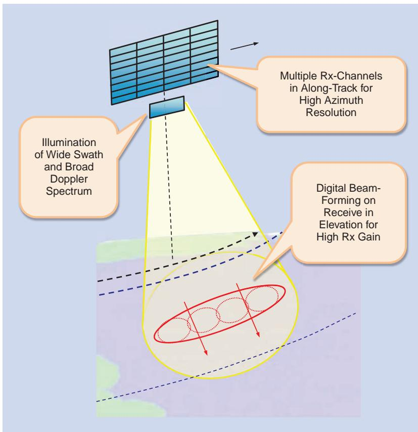
**FIGURE 26.** High-resolution wide-swath (HRWS) SAR system. The displaced phase center technique in azimuth is combined with real-time digital beamforming on receive in elevation to overcome fundamental limitations of conventional SAR systems. This enables the mapping of a wide image swath with high geometric resolution. In the meantime this concept has been extended to use the same antenna for transmit and receive.
