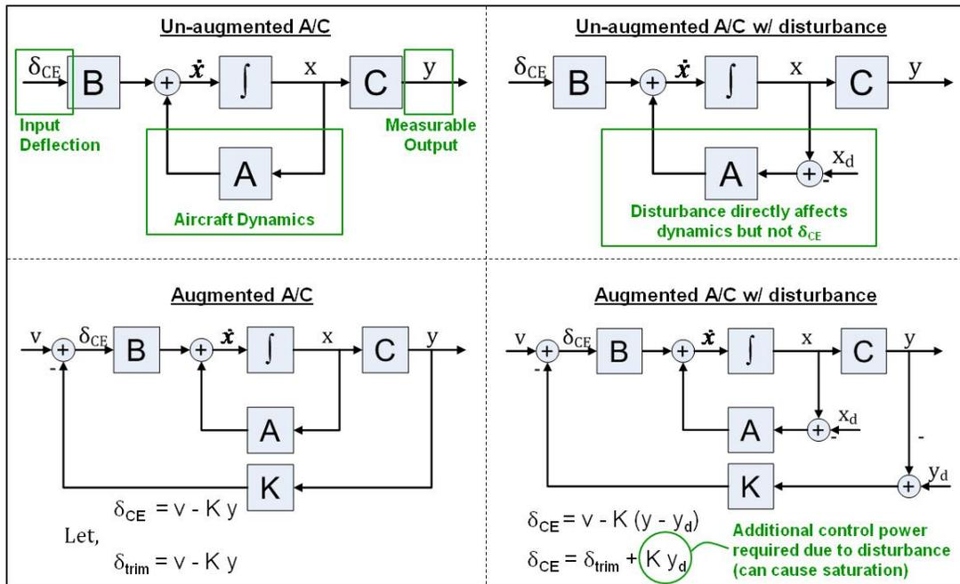
Figure 2.4 block diagrams showing increase in control power requirement
