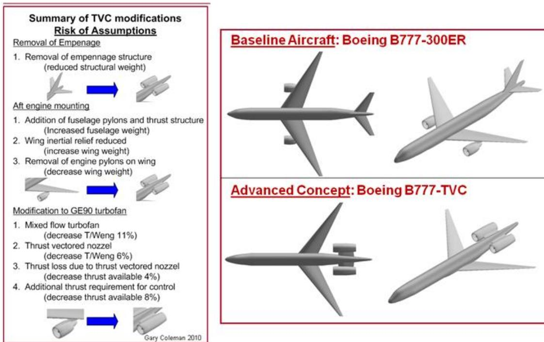
Figure 5.2 Modifications to the B777-300ER for Thrust Vector Control (Coleman 2010, 404)
