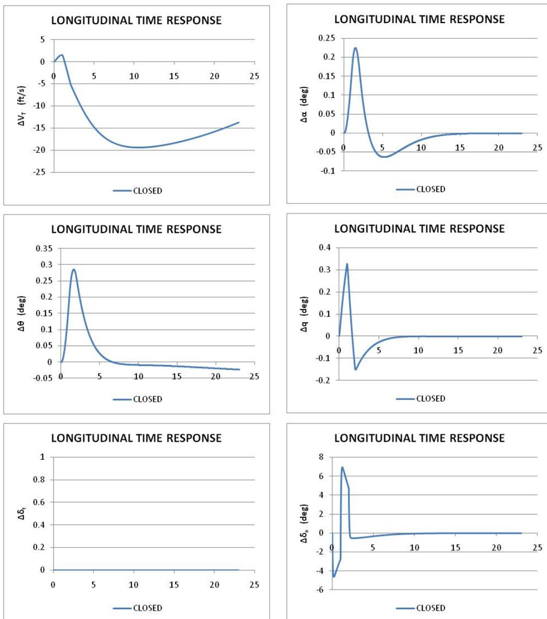
Figure 5.15 Closed loop time response of the TVC transport to a 5 deg elevator doublet
