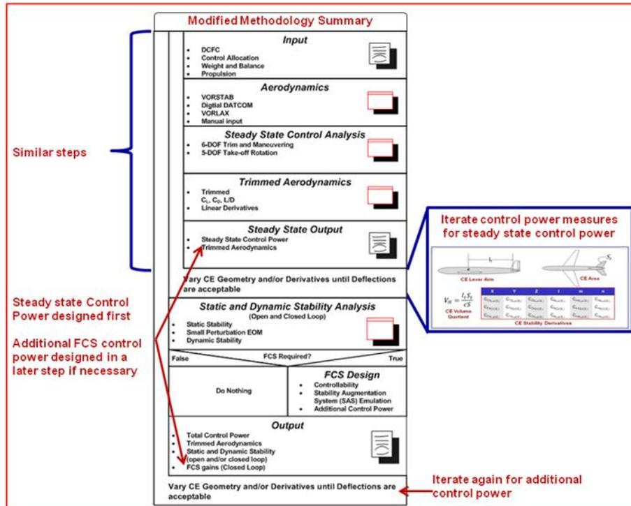
Figure 5.1 *AeroMech* methodology showing iteration steps for control power
