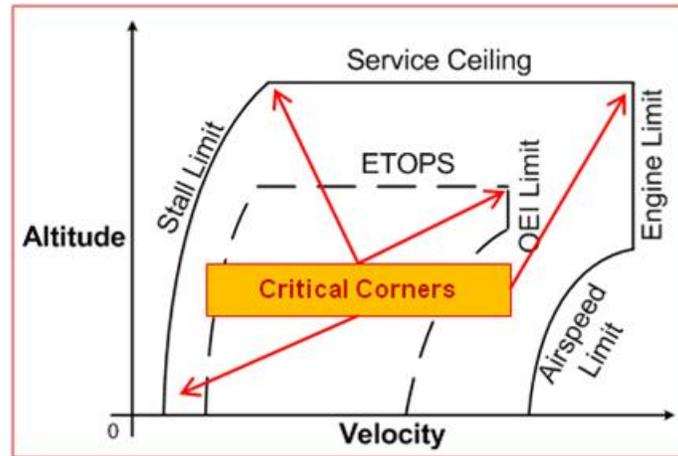
Figure 4.2 A typical flight envelope and the some critical corners
