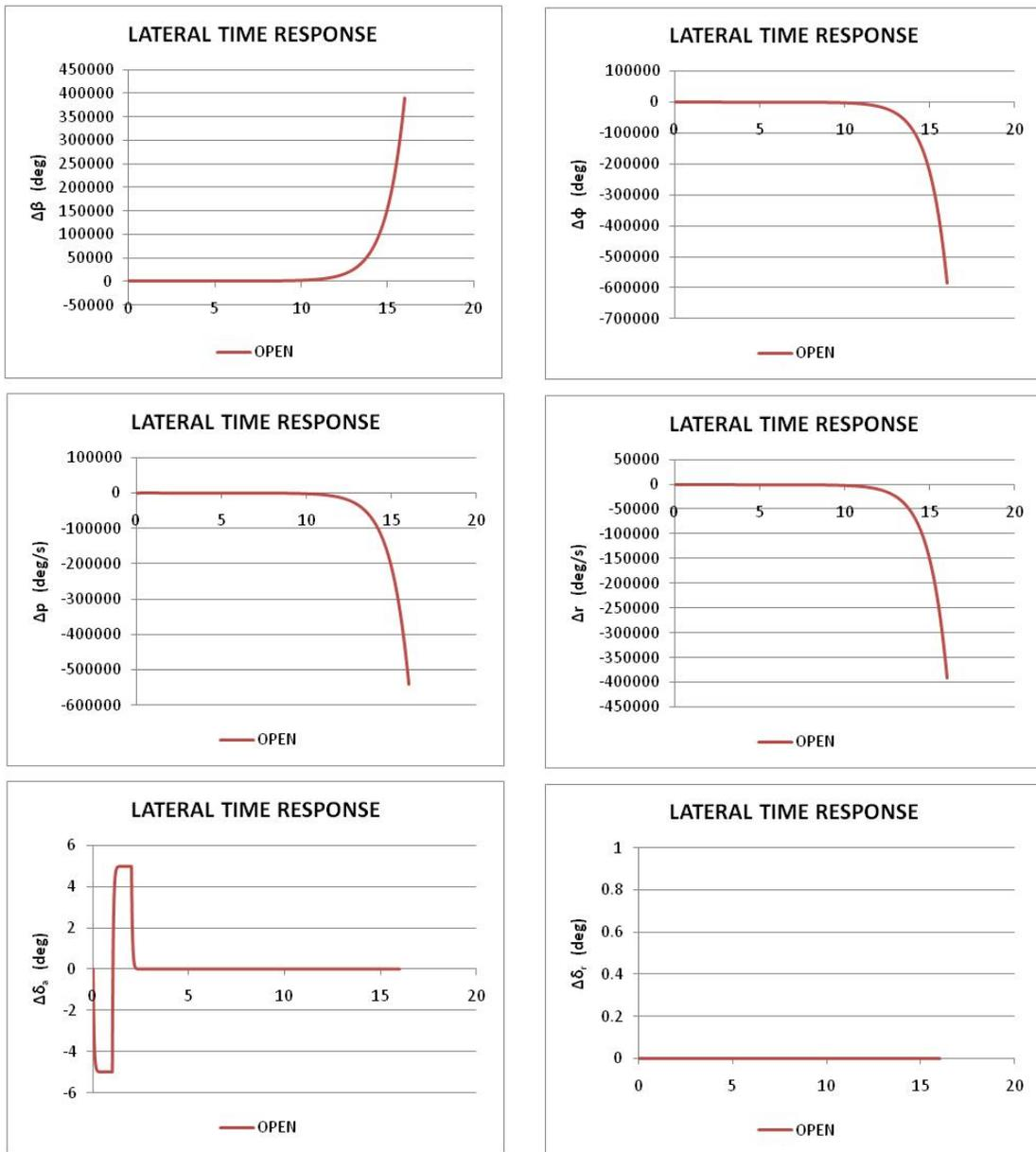
Figure 5.12 Open loop time response of the TVC transport to a 5 deg aileron doublet
