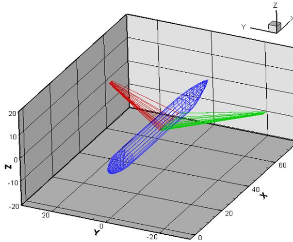
Figure 5.4 the Digital DATCOM model of the TVC aircraft
