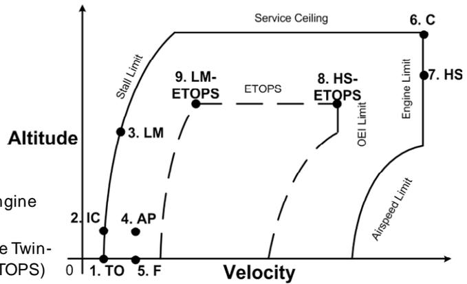
Figure 5.3 Critical corners of the flight envelope for control power assessment of a TVC transport
