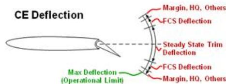
Figure 2.3 Control power representation using control effector deflection
