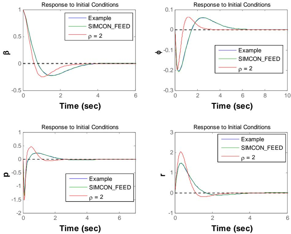
Figure 3.4 Response of system design with proposed algorithm to initial sideslip
