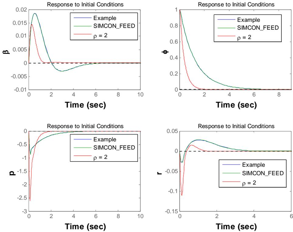
Figure 3.5 Response of system design with proposed algorithm to initial bank angle
