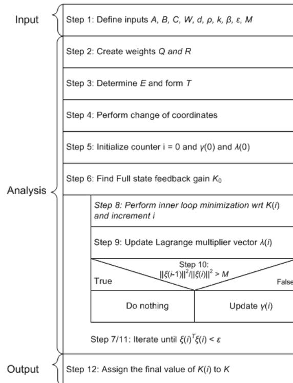
Figure 3.1 Summary of algorithm for constrained output feedback of similar system
