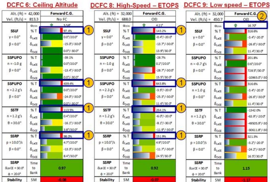
Figure 5.9 Control power assessment chart for engine limit conditions
