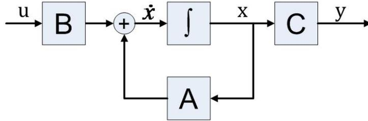
Figure 2.2 Block diagram of aircraft LTI model with feedback control
