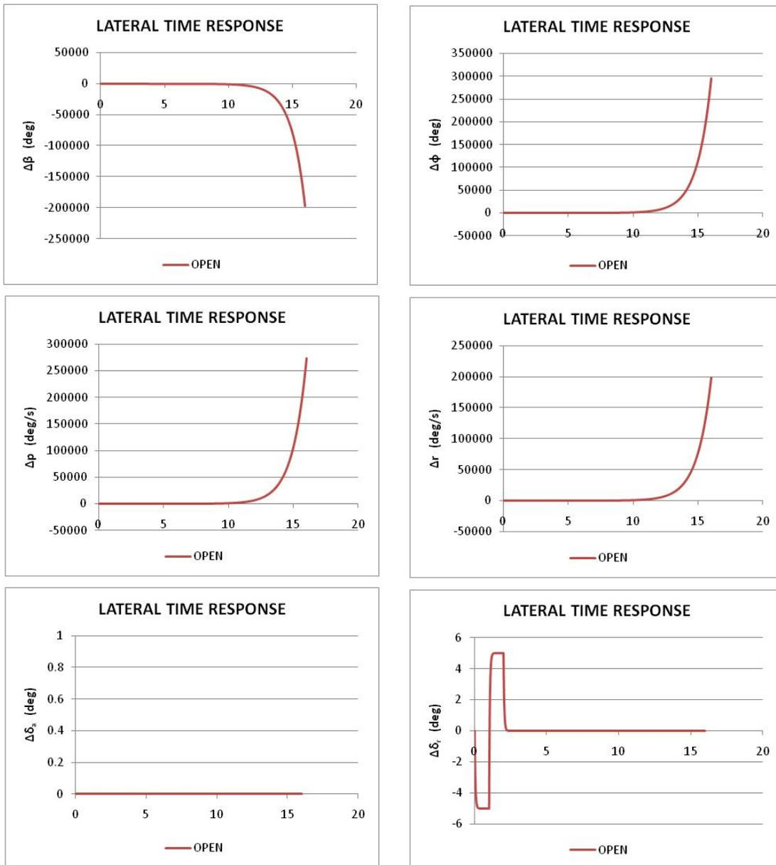
Figure 5.13 Open loop time response of the TVC transport to a 5 deg rudder doublet
