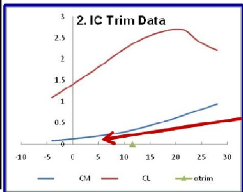
Figure 5.7 Control power assessment charts and trimmed aerodynamic data for the stall conditions IC and LM
