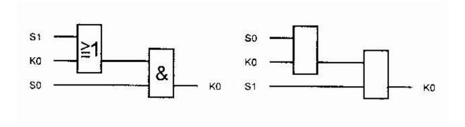
Of course, an RS flip-flop can also be programmed to realize a seal-in circuit. As PLC commands are always processed sequentially, the command processed last has priority. In the case of a reset priority, the switching condition for resetting the RS flip-flop must be programmed last.
