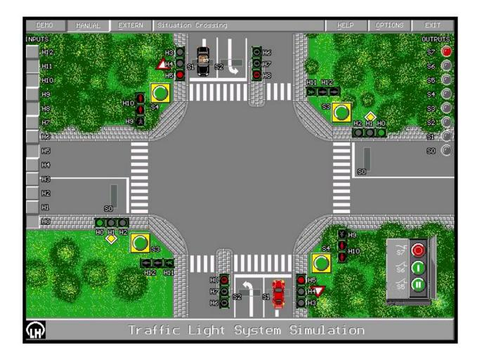
A crossing is displayed on the screen. A main road with single-lane traffic in either direction is shown. The pair of traffic-light units HO to H2 regulates the flow of automobile traffic here.
