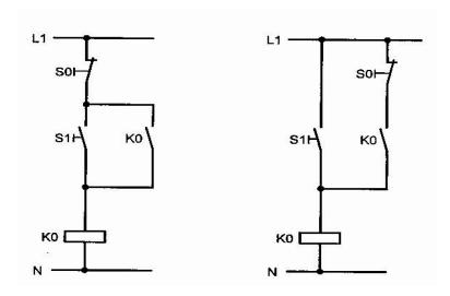
These two circuit diagrams are to be converted into logic diagrams. As SO is an NC-contact, it must be scanned for a 1-signal. Complete the logic diagram on the right.
