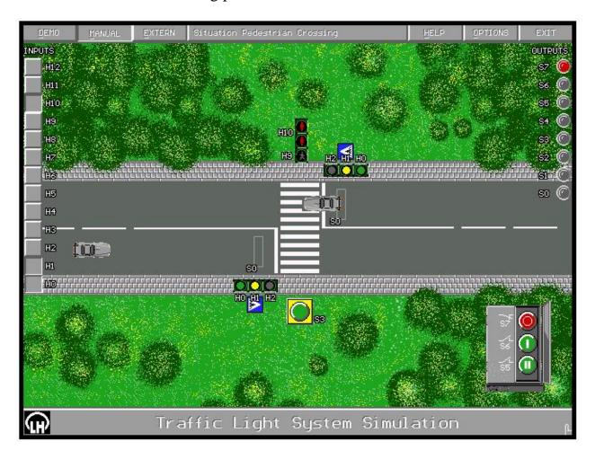
A road with a single lane in either direction is shown across the screen. A pedestrian crossing is located in the middle. Two sets of traffic lights each with three lights H0 (green), H1 (yellow) and H2 (red) are present for regulating the automobile traffic flow. The traffic lights are controlled in parallel. One set of traffic lights with the lights H9 (green) and H10 (red) is present for pedestrians. For reasons of clarity, only one set of traffic lights is shown here. In reality, there is
