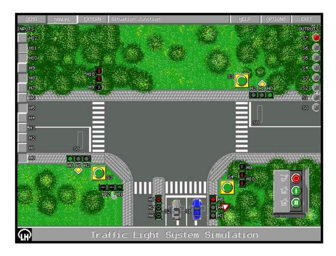
A main road with one lane in either direction is shown across the screen. A junction with a side road is located in the middle. The junction has a left-turning and a right-turning lane.
