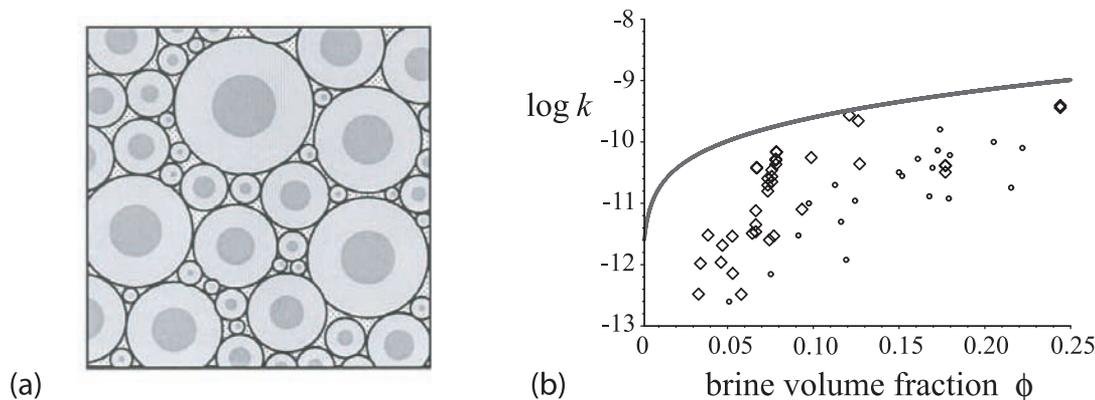
**Figure 11. (a) Hashin-Shtrikman coated cylinders provide an optimal geometry which attains the two-point void upper bound for the vertical fluid permeability. (b) The lognormal pipe bounds capture all our lab and field data on the vertical permeability of sea ice.**
