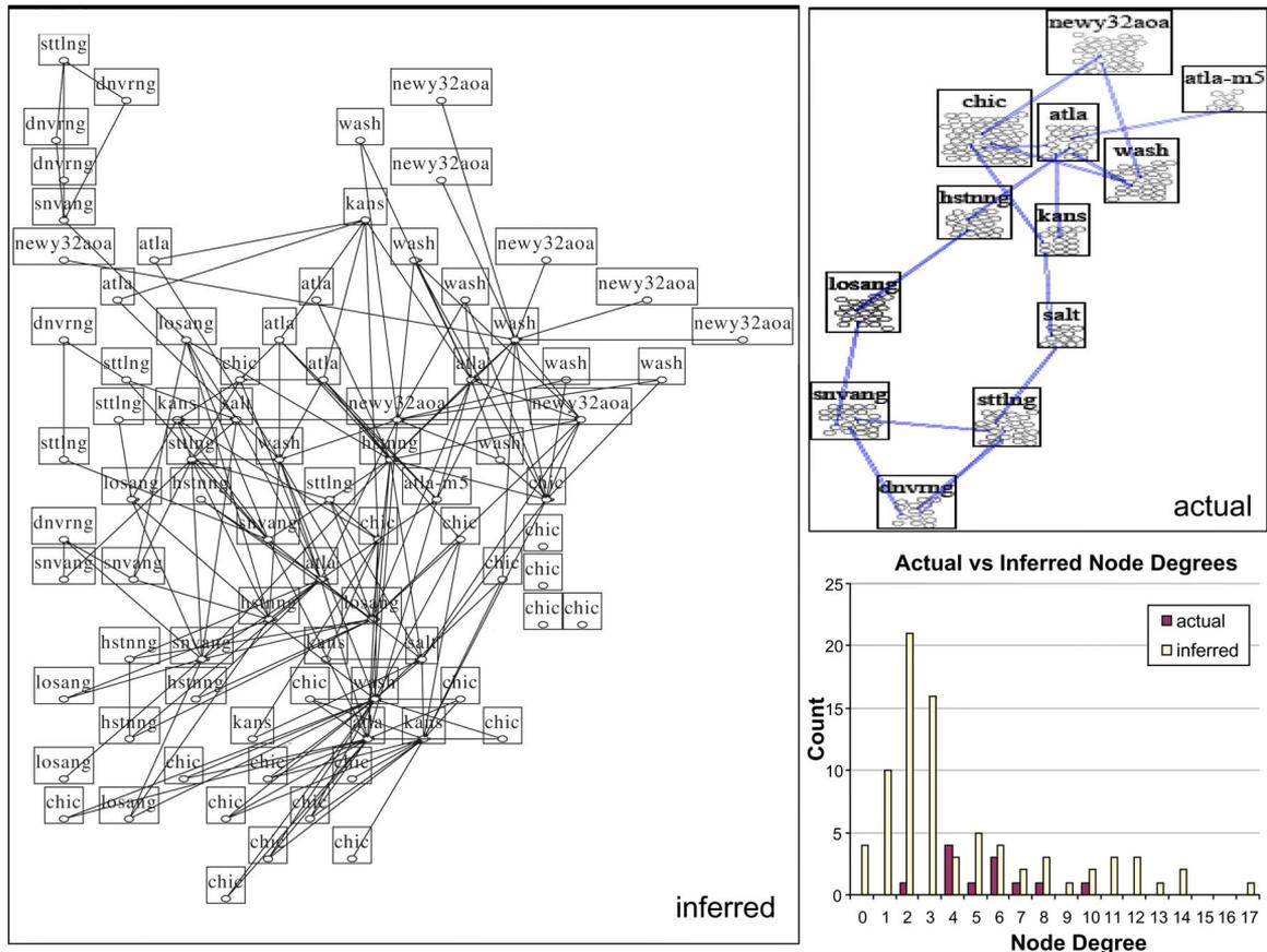
**Figure 3. The IP alias resolution problem in practice. This is re-produced from [48] and shows a comparison between the Abilene/Internet2 topology inferred by Rocketfuel (left) and the actual topology (top right). Rectangles represent routers with interior ovals denoting interfaces. The histograms of the corresponding node degrees are shown in the bottom right plot. © 2008 ACM, Inc. Included here by permission.**
