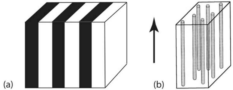
**Figure 10. (a) The conductivity of a two-phase composite in a vertical electrical field is maximized by laminate structures parallel to the field. (b) The vertical fluid permeability of a porous medium is maximized by vertical pipes with appropriate radii.**
