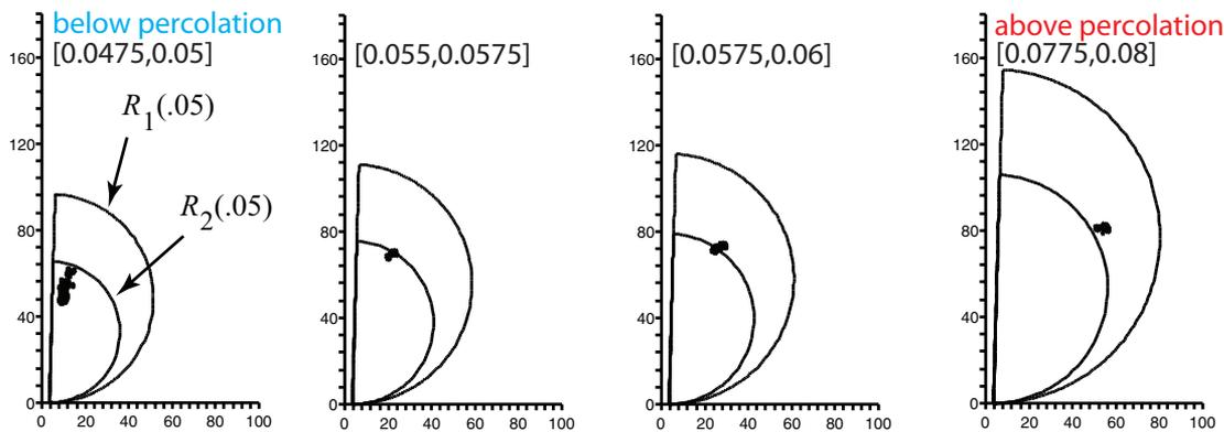
Figure 21. Comparison of ice tank data on the complex permittivity of sea ice at 50 MHz over ranges of  $\phi$  with the elementary (outer) and isotropic (inner) bounds. The data violate, or lie outside, the isotropic bounds as brine volume increases through the percolation threshold and an anisotropic, connected brine structure is formed.
