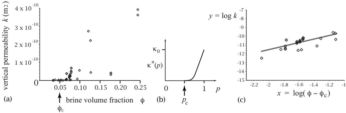
**Figure 16. (a) Data for  $k$  taken *in situ* on Arctic sea ice, displayed on a linear scale. (b) The effective permeability  $\kappa^*(p)$  in a lattice percolation model, displayed on a linear scale. (c) Comparison of Arctic permeability data in the critical regime (25 data points) with percolation theory in (15). In logarithmic variables the predicted line has the equation  $y = 2x - 7.5$ , while a best fit of the data yields  $y = 2.07x - 7.45$ , assuming [5]  $\phi_c = 0.05$ .**
