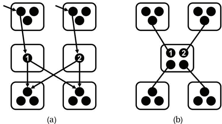
**Figure 2. The IP alias resolution problem.** Paraphrasing Fig. 4 of [50], traceroute does not list routers (boxes) along paths but IP addresses of input interfaces (circles), and alias resolution refers to the correct mapping of interfaces to routers to reveal the actual topology. In the case where interfaces 1 and 2 are aliases, (b) depicts the actual topology while (a) yields an "inflated" topology with more routers and links than the real one.
