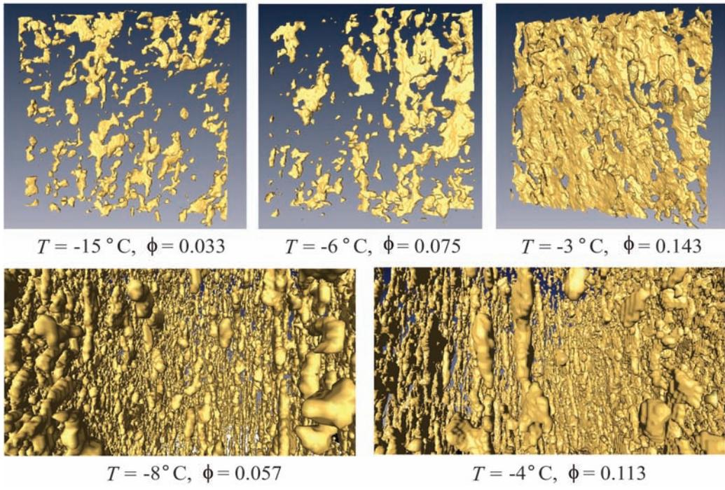
Figure 15. X-ray CT volume rendering of brine layers within a lab-grown sea-ice single crystal with  $S = 9.3$  ppt. The (non-located)  $8 \times 8 \times 2$  mm sub-volumes (top row) illustrate a pronounced change in the micro-scale morphology and connectivity of the brine inclusions during warming. Images from a cylinder of height 8 mm and diameter 21 mm are shown in the bottom row.
