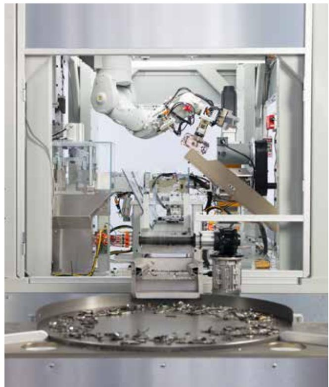
**Figure 7.** Apple has a new iPhone-destroying robot called Daisy that can disassemble 200 phones in an hour. Source: Courtesy of Apple Inc.
