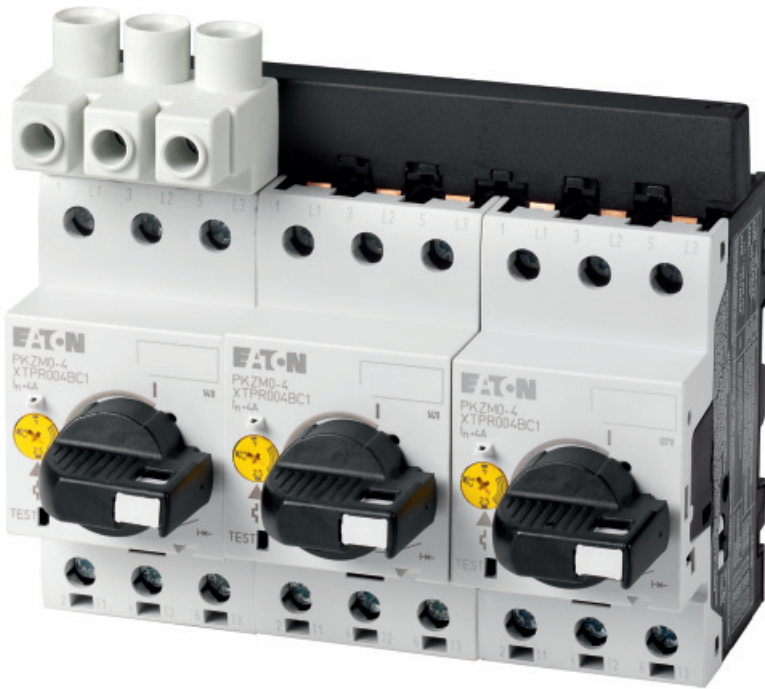
Figure 3: An array of PKZM0 motor-protective switches with commoning link and incoming terminal accessories. The common power feed terminal BK25...-E provides the increased air and creepage clearances required on the incoming side of UL 508 Type Self-protected combination motor controllers/starters. The terminal block is not necessary for applications in Canada should it be possible to accommodate the necessary supply conductor cross-sections without its usage. All handles must be padlockable in the OFF position. Application of these controllers in motor branch circuits only.
