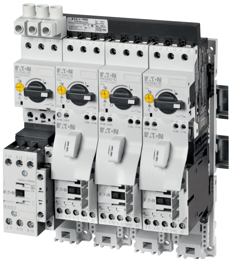
Figure 4: A "Type F Combination Motor Controller" construction results from matching and certifying "Type E" devices with suitable load side controllers such as contactors.
