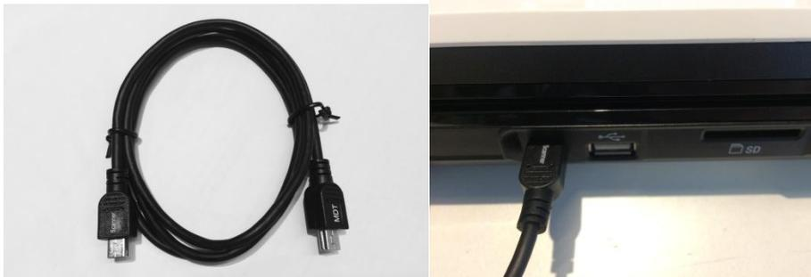
2. Plug the other end of the special USB cable with marked “MDT” to the Device or the Cradle
