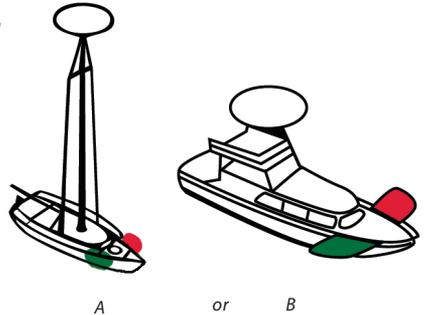
Vessels less than 39.4 feet long, including vessels equipped with electric outboard motors, may show the lights in either figure 1 or 2.
