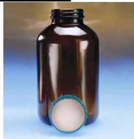
Glass bottles must be used. The type of cap required will depend upon the analyte and method the lab is using. Talk to the lab to be sure.
