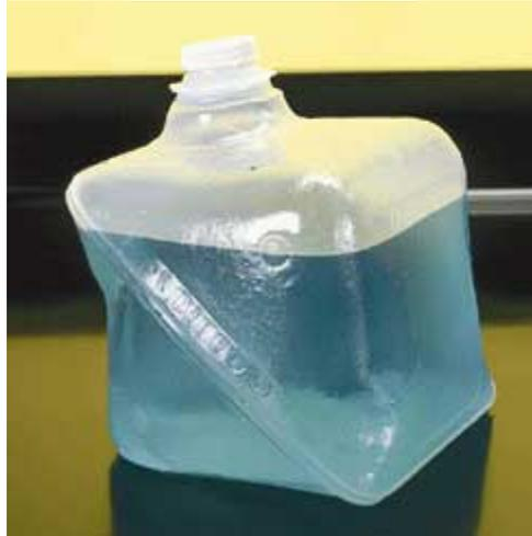
Plastic cubitainers or equivalent which can hold 10 L samples are used.
