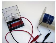
4. Move the magnet near the wire and watch the Ammeter to see what happens. The needle should move showing you that electricity has been generated.
