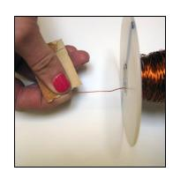
3. Connect the alligator clips from the Ammeter to the exposed wire of one spool (least amount of wire).
