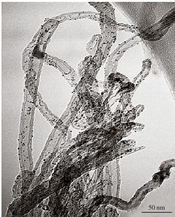
**Fig. 3.30** Transmission electron microscopy image showing rhodium nanoparticles supported on the surface of an MWNT (from [3.306])
