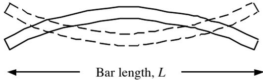
**Figure 7.1: First mode of vibration.** This is the simplest way for a bar or pipe to vibrate transversely in a standing wave condition with both ends free. This mode generates the fundamental frequency.
