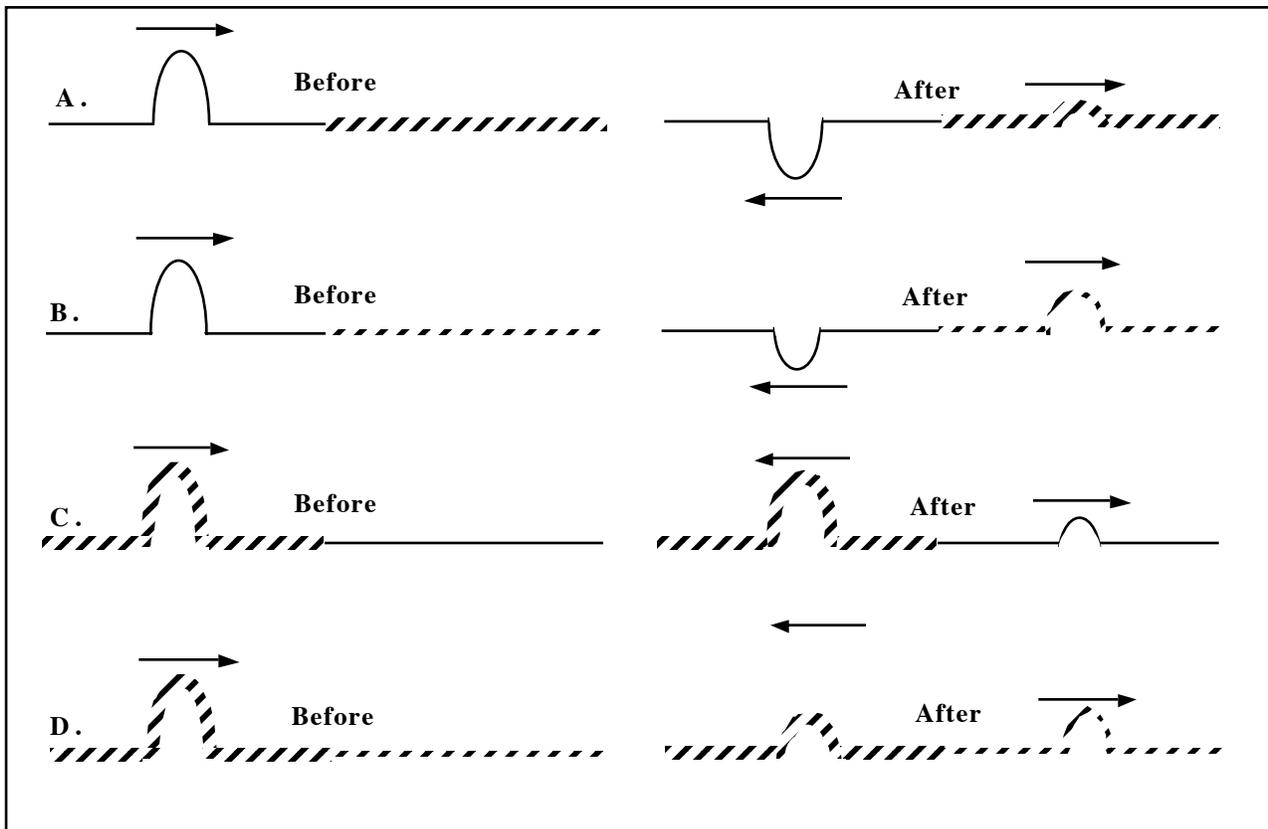
Figure 2.7: Wave pulse encountering medium with different impedance
