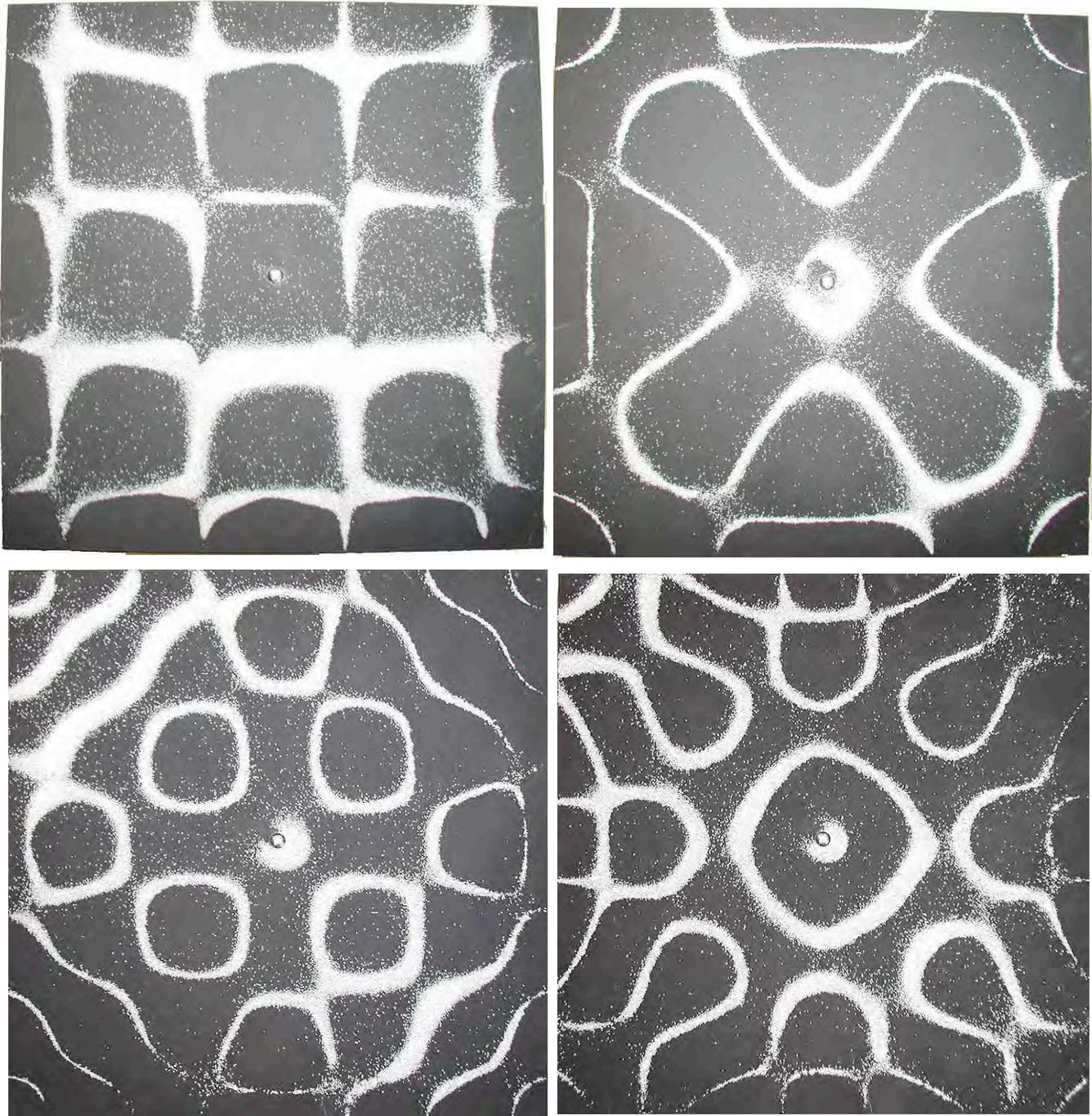
**Figure 2.2:** A flat square metal plate is driven in four of its resonance modes. These photographs show each of the resulting complicated two-dimensional standing wave patterns. Sand poured onto the top of the plate bounces off the antinodes, but settles into the nodes, allowing the standing wave to be viewed. The head of a drum, when beaten, and the body of a guitar, when played, exhibit similar behaviors.
