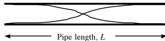
**Figure 6.6:** First mode of vibration. This is the simplest way for a column of air to vibrate (in an open pipe) in a standing wave condition. This mode generates the fundamental frequency.
