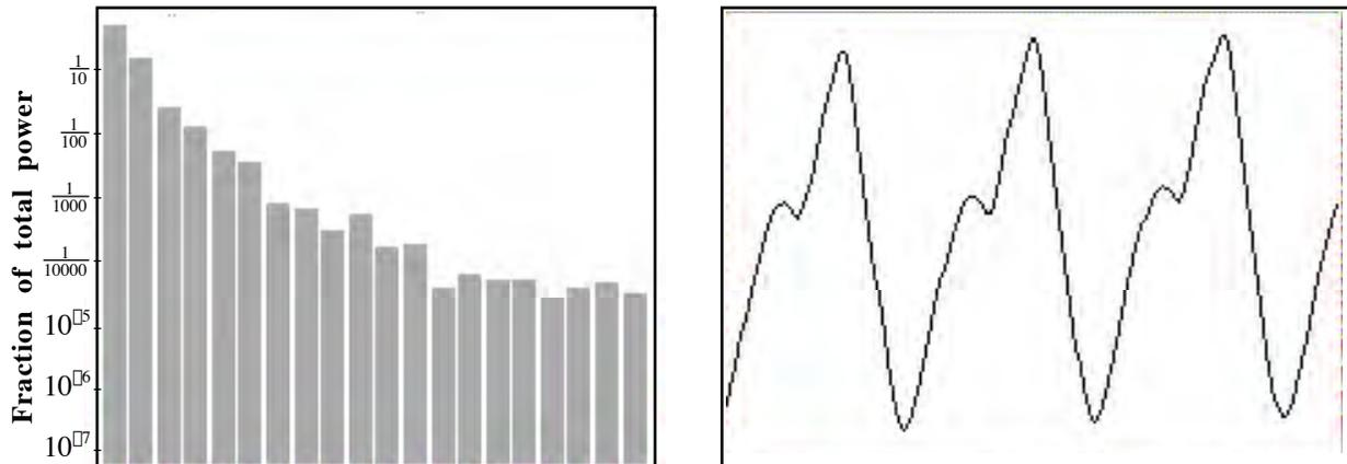
Figure 3.5:  $E_5$  played on the [VIOLIN](#). Note the dominance of the fundamental frequency. The most powerful overtone is the 1<sup>st</sup>, but only slightly more than 10% of the total power. The higher overtones produce much less power. Of the higher overtones, only the 2<sup>nd</sup> overtone produces more than 1% of the total power. The result is a very simple waveform and the characteristically pure sound associated with the violin.
