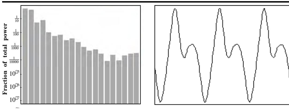
Figure 3.9:  $B_4$  played on the **BASSOON**. The power spectrum is much different for this high note played on the same bassoon. Over two octaves higher than the note producing the power spectrum in Figure 3.8, the first two harmonics dominate, producing almost all the power. The third and fourth harmonics produce far less than 10% of the total power and all the remaining higher harmonics produce less than 1% combined. The result is a simple waveform with an almost flute-like sound.
