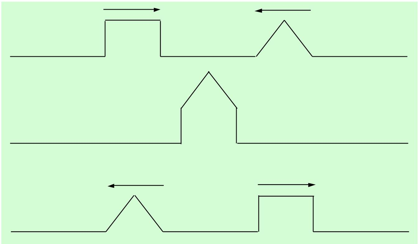
**Figure 1.8: Wave superposition.** Note in the middle drawing that the wave shape is simply the arithmetic sum of the amplitudes of each wave. Note also in the bottom drawing that the two waves have the same shape and amplitude as they had before encountering each other.
