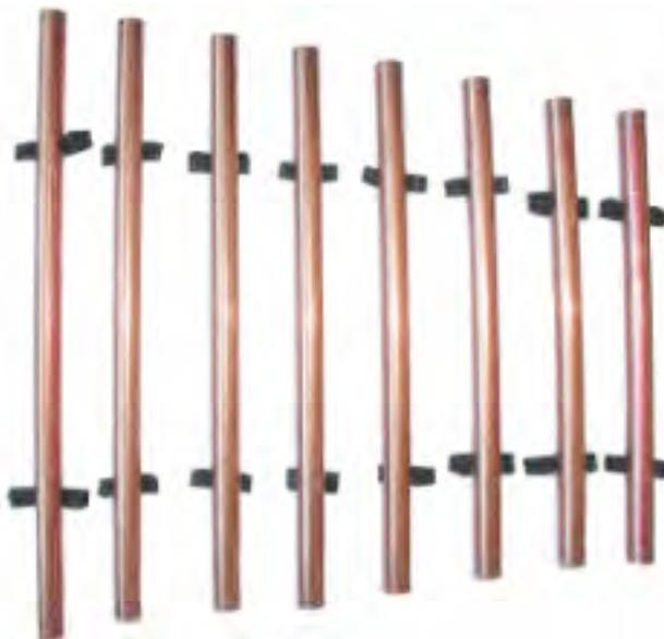
**This “xylophone,” made from a single 10-foot length of 1/2” copper pipe plays the C<sub>5</sub> major scale.**
