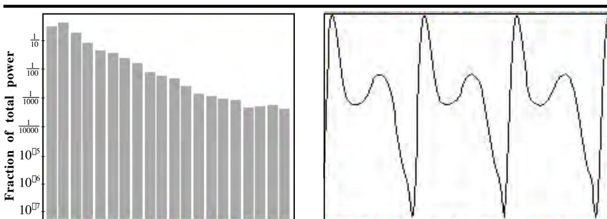
Figure 3.11:  $D_5$  played on the [TRUMPET](#). The fundamental frequency and the first two overtones dominate the power spectrum, with all three contributing over 10% of the total power. The next five harmonics all contribute above 1% of the total power. However, even with the much greater prominence of the 3<sup>rd</sup> through 7<sup>th</sup> overtones, when compared to the bassoon's  $B_4$  note, the waveform graphs of the trumpet  $D_5$  and the bassoon  $B_4$  are surprisingly prominent.
