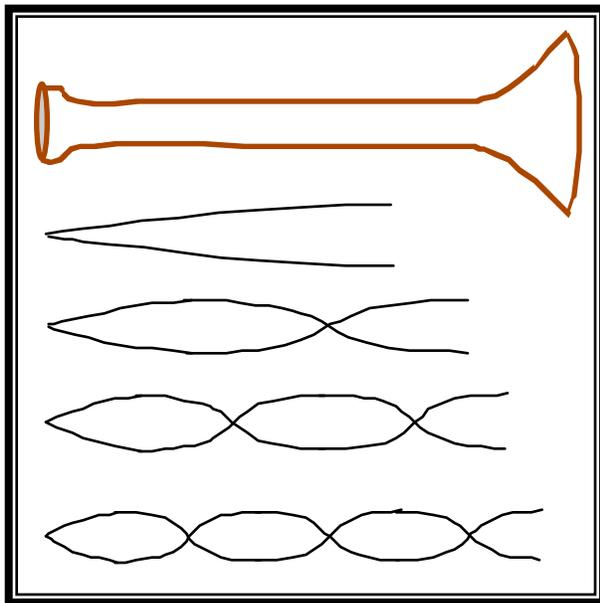
**Figure 6.11:** The bell of a brass instrument causes lower modes to reflect prior to reaching the end of the instrument. This smaller wavelength for the lower modes increases their frequencies, forcing them to approach the harmonicity of an open pipe.
