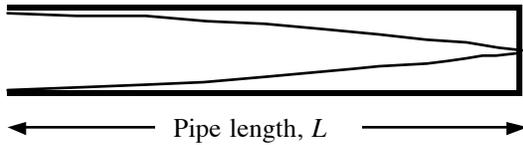
**Figure 6.9: First mode of vibration.** This is the simplest way for a column of air to vibrate (in a closed pipe) in a standing wave condition. This mode generates the fundamental frequency.
