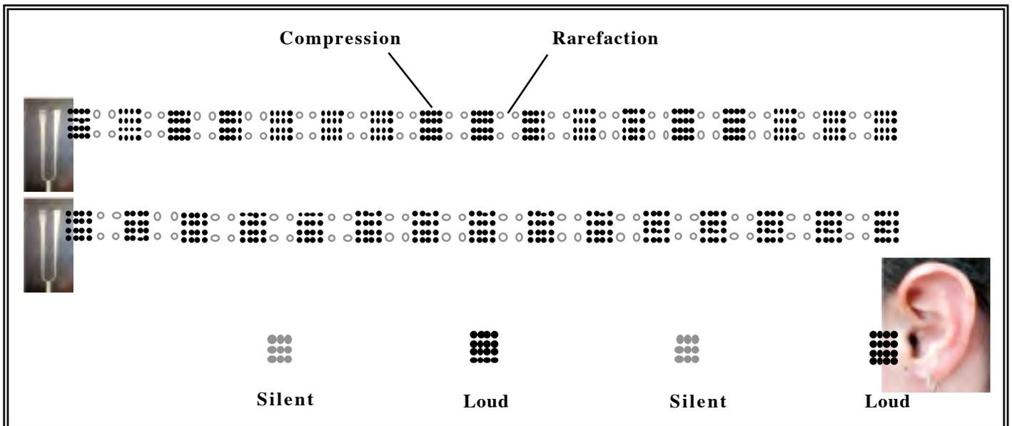
**Figure 3.12: Beats.** The two tuning forks have slightly different frequencies. This causes the sound waves produced by each one to interfere both constructively and destructively at various points. The constructive interference causes a rise in the intensity of the sound and the destructive interference causes silence. This pattern is repeated over and over causing the phenomenon of beats.
