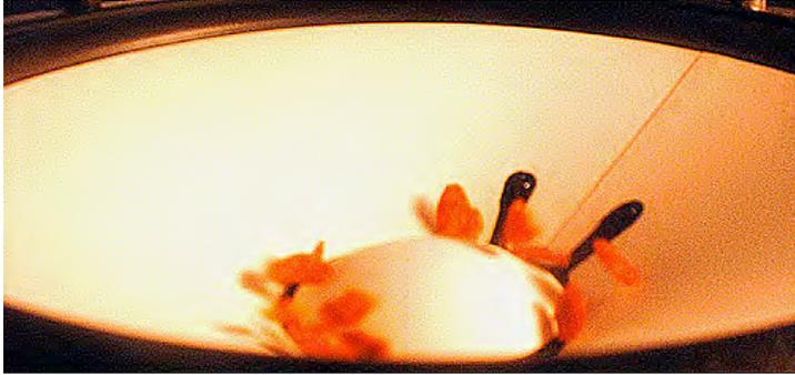
**Figure 1.7: The front of a speaker cone faces upward with several pieces of orange paper lying on top of it. Sound is generated when an electric signal causes the speaker cone to move in and out, pushing on the air and creating a compressional wave. The ear can detect these waves. Here these vibrations can be seen as they cause the little bits of paper to dance on the surface of the speaker cone.**
