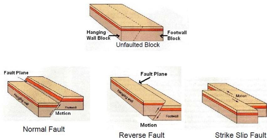
Figure 1.9 Types of faults
