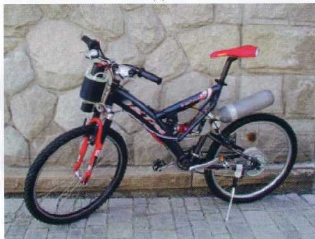
CHAPTER 9, COLOR FIGURE 9.5 (a) This 600-W power supply unit developed by NovArs/Manhattan Scientific is based on a polymer electrolyte fuel cell that uses compressed hydrogen and air to produce electric power. (b) Manhattan Scientifics' Hydrocycle presented in June 2000. On the fuel cell bicycle, compressed hydrogen flows from a 2-liter cylindrical tank to the fuel cell. (Photographs courtesy of Manhattan Scientifics).
