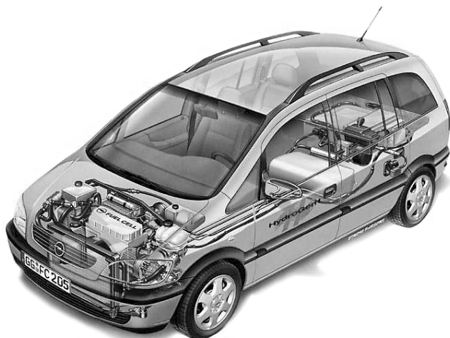
FIGURE 10.2 HydroGen 1 fuel cell prototype produced by General Motors/Opel in 2000. HydroGen 1 runs 400 km on a 75-liter tank of liquid hydrogen. (Photograph courtesy of Adam Opel AG.) (Please check Color Figure 10.2 following page 9-10.)
