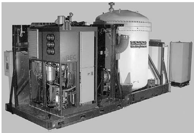
FIGURE 8.14 Pressurized hybrid (micro gas turbine) technology in a 220-kW system for Southern California Edison. (Photograph courtesy of Siemens-Westninghouse.) (Please check Color Figure 8.14 following page 9-10.)
