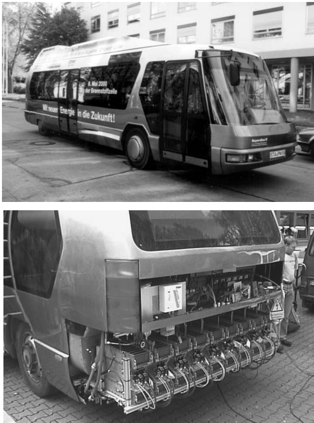
FIGURE 10.19 Bus developed by Proton Motor (with Neoplan). The bus features a special flywheel energy storage device. (Photographs courtesy of Proton Motor.) (Please check Color Figure 10.19 following page 9-10.)
