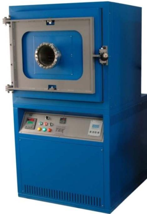
Figure 32. Cascade TEK High Vacuum Oven
