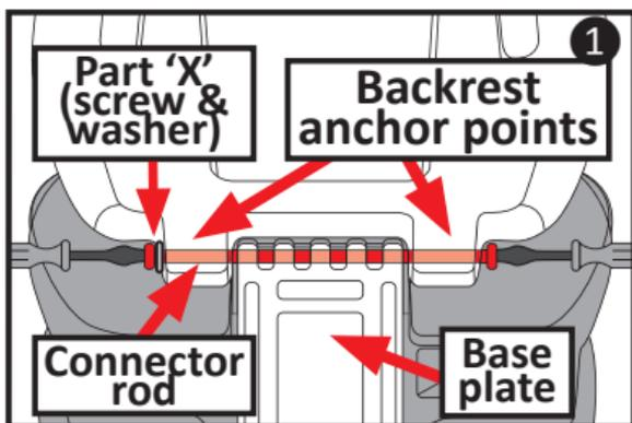
**TIP:** If connector rod does not pass through easily, make sure it is aligned with holes and tap screw head lightly to guide it through the plastic.
