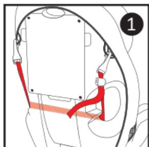
2. Thread the vehicle seat belt through the belt slot opening and out the other side. See illustrations for proper routing path of Lap-and-Shoulder Belt ② or Lap-Only Belt ③.
