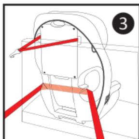
5. Tighten vehicle seat belt by placing your knee on the seat base and by using your full weight to push the child restraint down ④ as you simultaneously release the extra belt length until seat belt is taught and has no slack ⑤.
