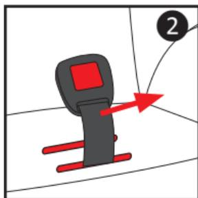
5. Push the buckle upwards through the fabric seat pad.
