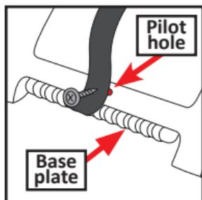
**! Before tightening screw, make sure belt strap is pointing upwards and that the **RED** belt guide opening is facing forward. **DO NOT** overtighten screw.**
