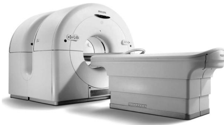
FIGURE 17.3 Philips Medical Systems Gemini CT_PET combo scanner. The rear section of the Gemini is the CT scanner while the front section has the PET scanner. This system allows registration of CT anatomical images with PET physiological information. (Courtesy of Philips Medical Systems, Amsterdam, the Netherlands.)
