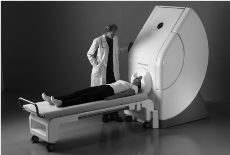
FIGURE 12.5 MEG machine with large SQUID. (Image courtesy of Elekta.)
