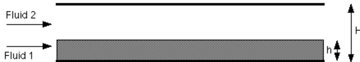
Two-layer, horizontal two-fluid flow
