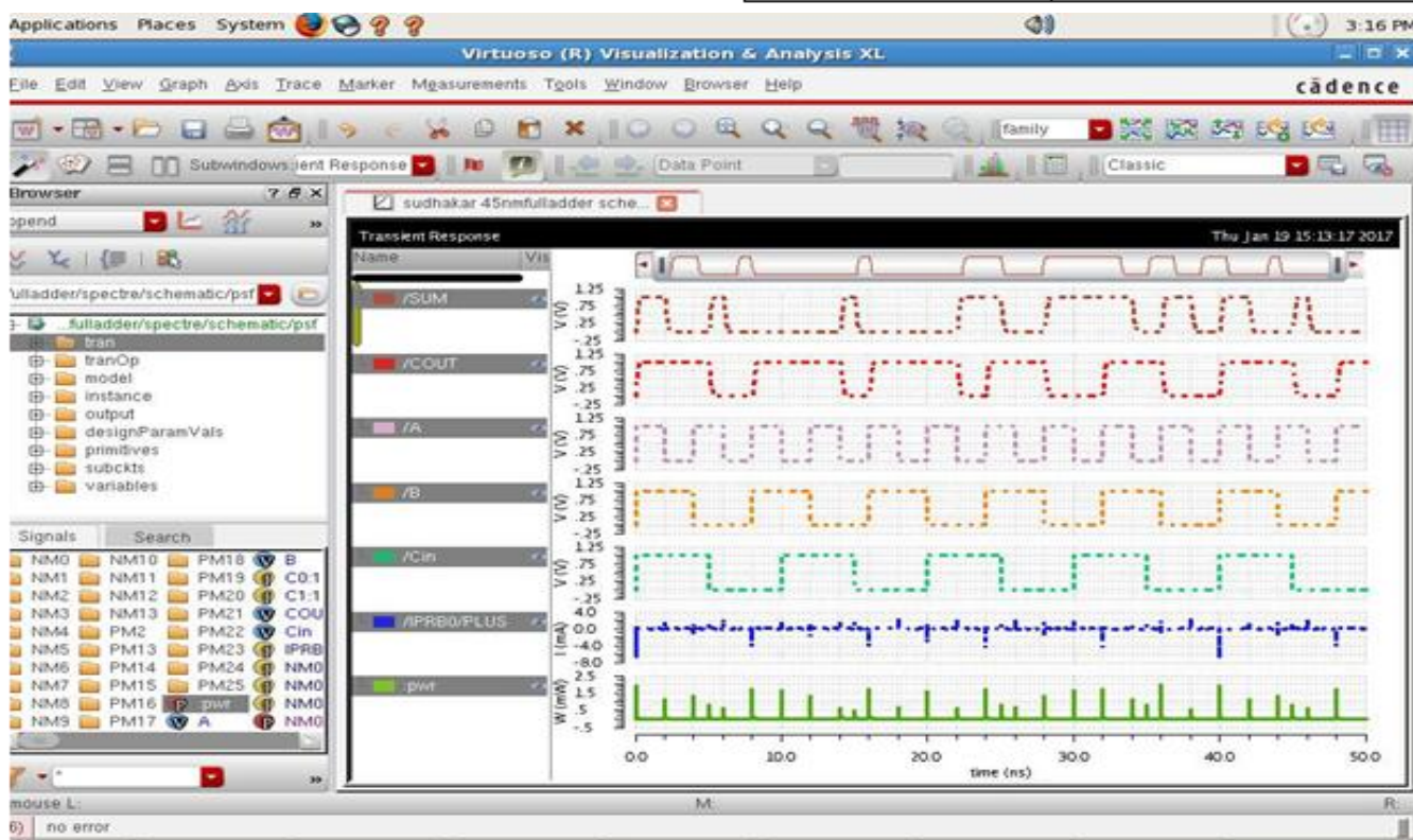
determine 18: Output Waveform of 28T full Adder in 45nm technology at 50MHz frequency & 1V
