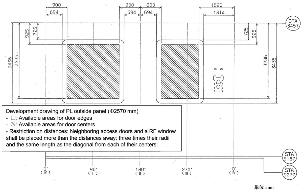
Figure 4.1.2-5 RF transparent window ( $\Phi 400$  mm)
