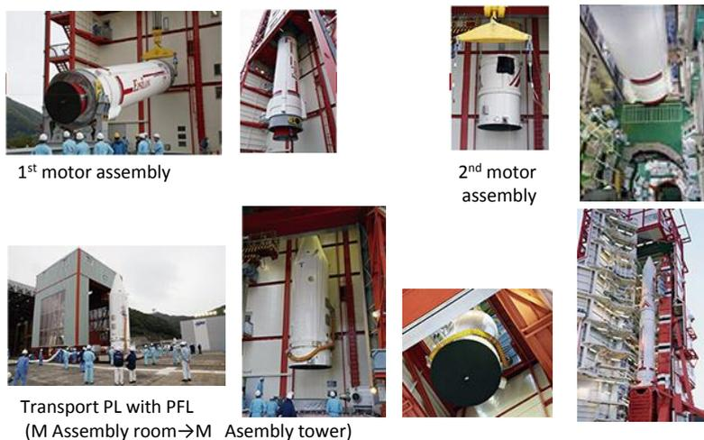
Figure 5.1.3-4 LV Assembly in M Assembly Tower
