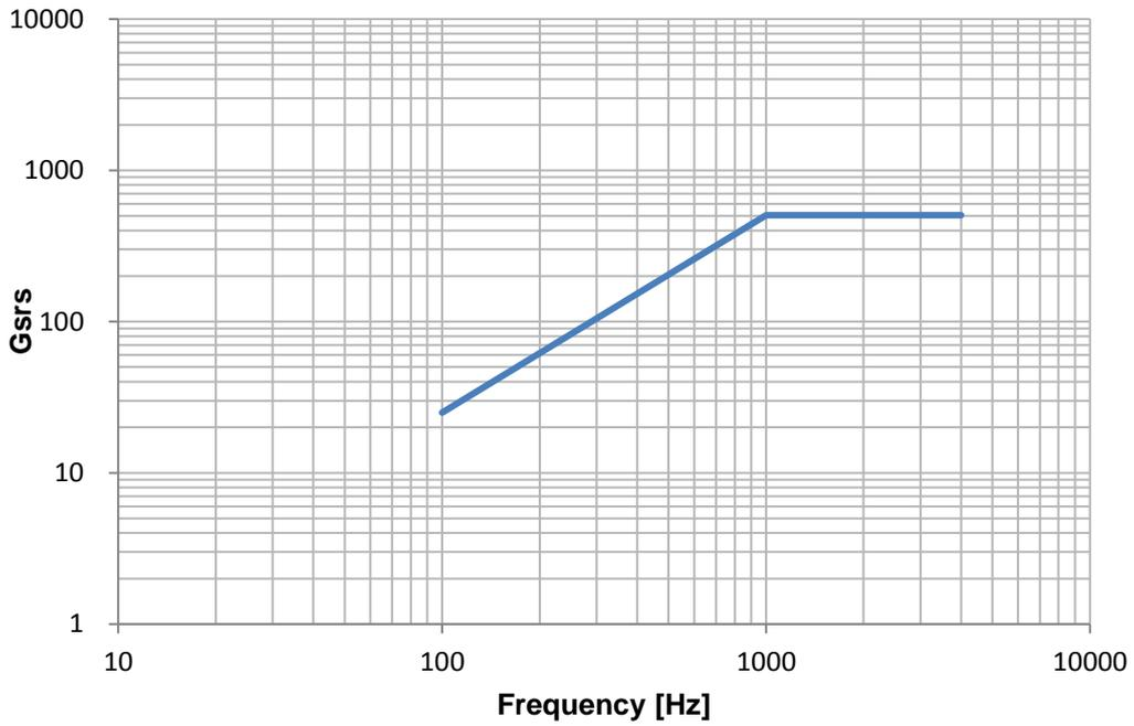
Figure 4.5.1-5 Standard Shock Environment of 40-60 kg PL
