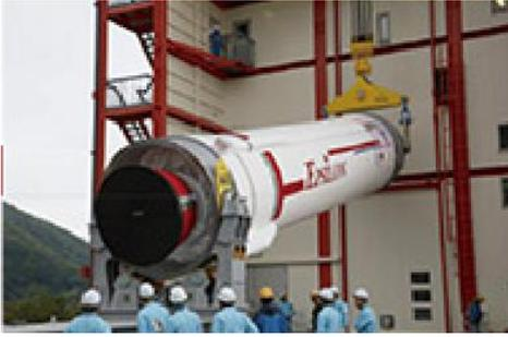
Assembling 1<sup>st</sup> motor**(1) First Stage (SRB-A3)**
