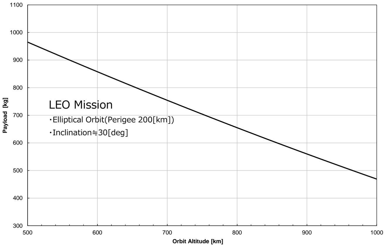
Figure 3-14 Launch Capability (Optional Configuration (with PBS))
