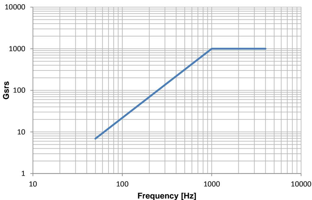
**Figure 4.5.1-4 Standard Shock Environment of 170-1200 kg PL**
