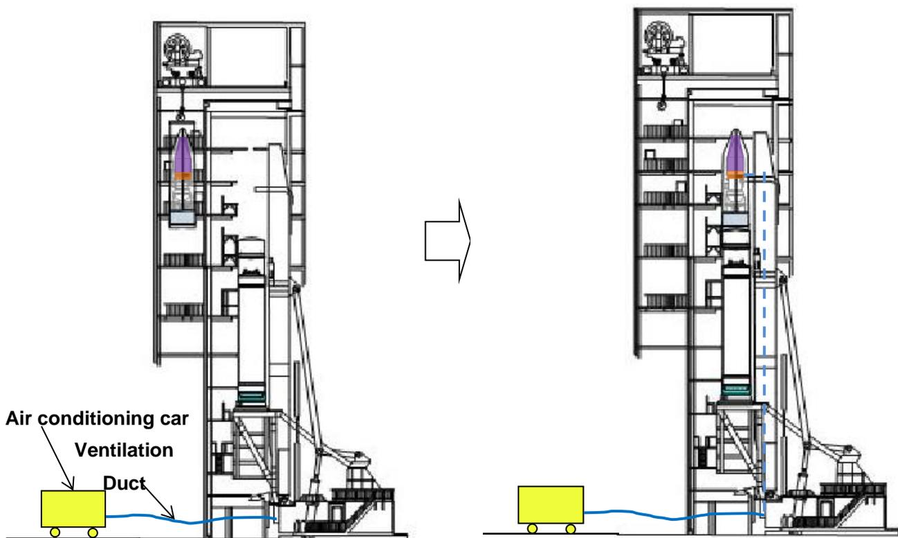
Figure 6.4-10 Mating with 2nd Stage of LV
