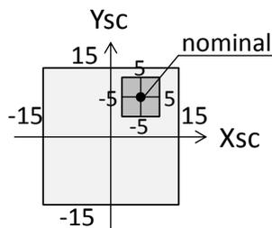
Figure 4.2.2-3 Limit of C.G. (Xsc, Ysc) of Micro satellite (B)
