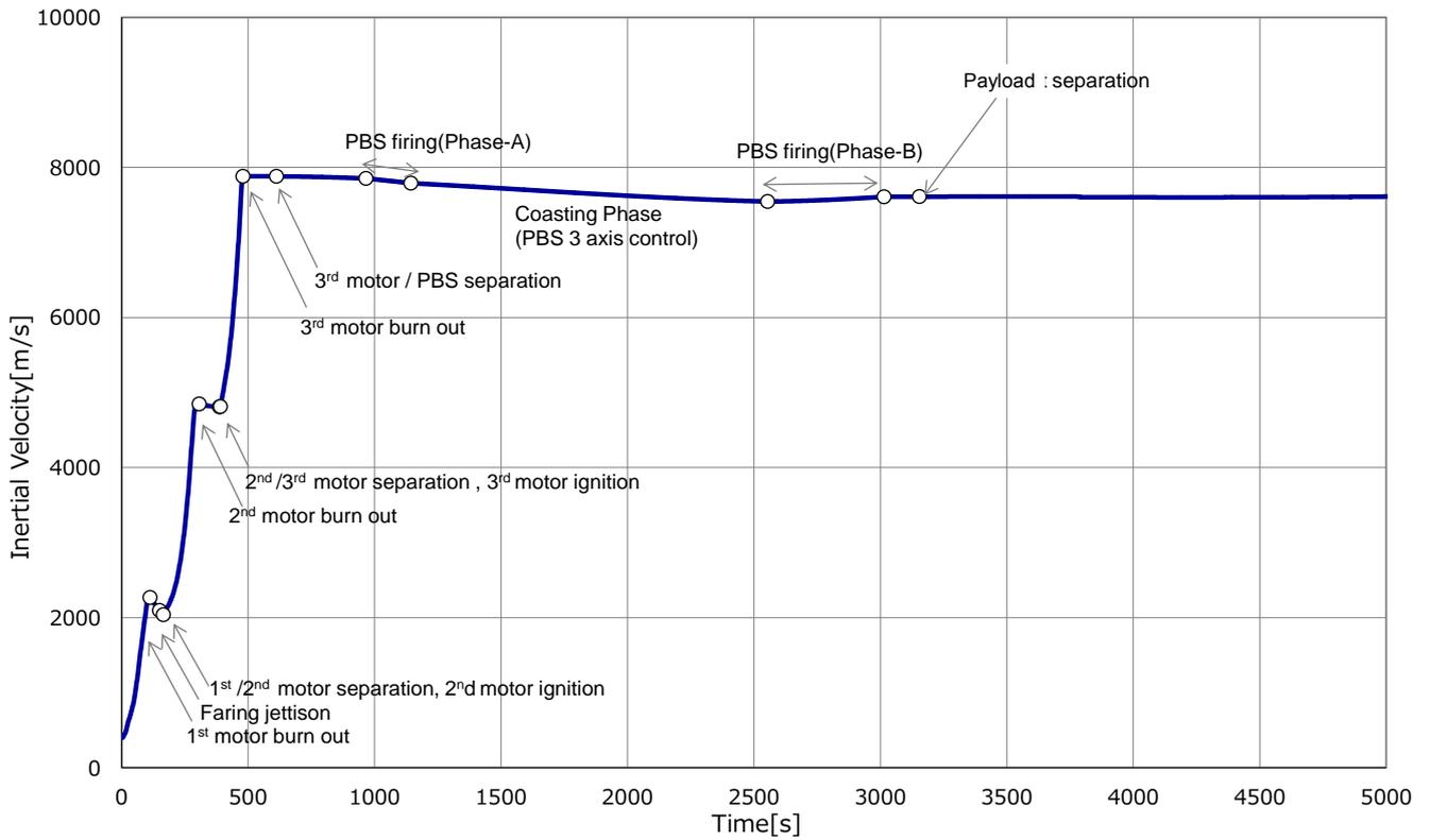
Figure 3-7 Nominal velocity for SSO mission (with PBS)
