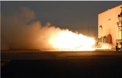
Combustion test of 2<sup>nd</sup> motor**(2) Second Stage (M-35)**
