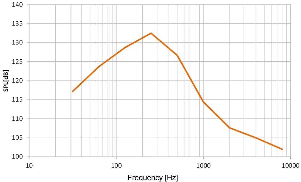
**Figure 4.5.1-3 Acoustic Vibration Environment**
