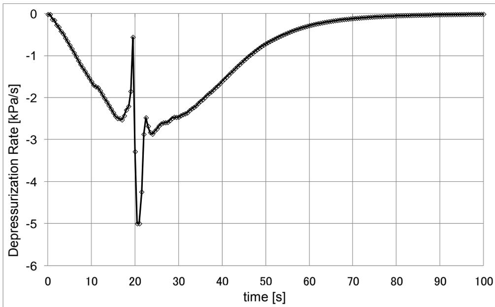
Figure 4.5.1-8 Typical Depressurization Rate Profile inside PLF
