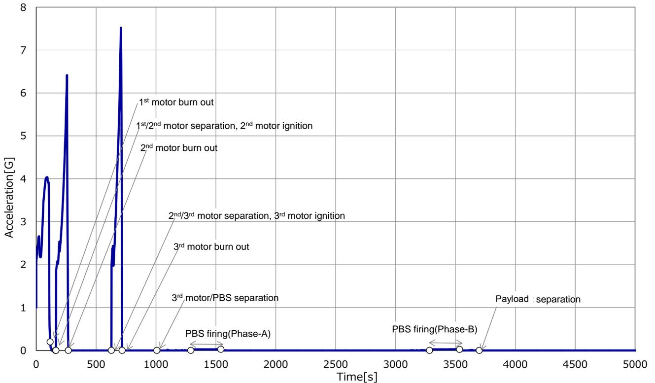
Figure 3-12 Nominal acceleration for LEO mission (with PBS)
