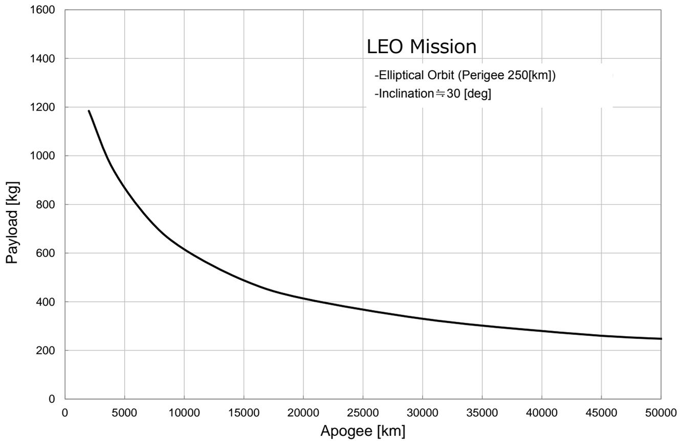
Figure 3-13 Launch Capability (Basic Configuration (without PBS))
