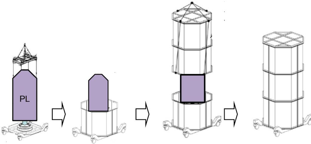
Figure 6.4-3 Preparation for Transfer to Clean Booth
