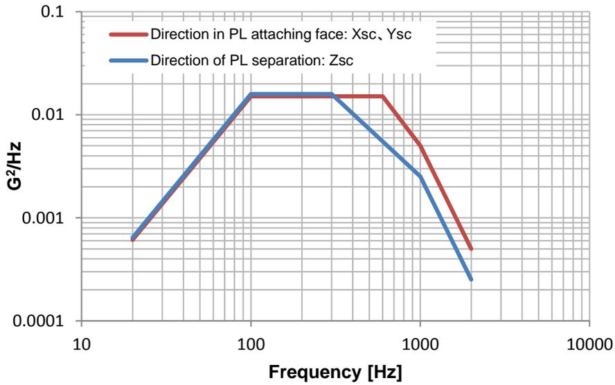
Figure 4.5.1-1 Random Vibration Environment of Micro Satellite
