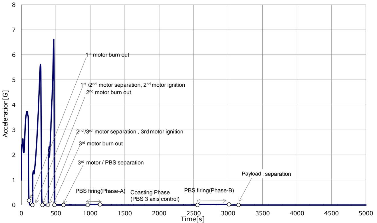
Figure 3-8 Nominal acceleration for SSO mission (with PBS)
