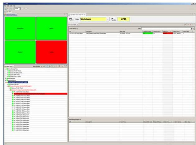
Figure 1: ANKA alarm panels. Top left corner represents the grouping on the machine into Storage Ring, Booster, Transfer Lines and Microtron. A single alarm due to an extraction power supply having different read and set values is shown.
