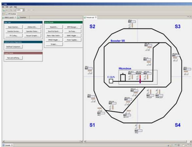
Figure 2: ANKA CSS panels. On the left side gives access to any device under EPICS control, and on the right side the pictorial representation of the selected devices.
