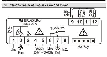
NOTE: The compressor relay is 20(8)A or 16(6)A depending on the model.
