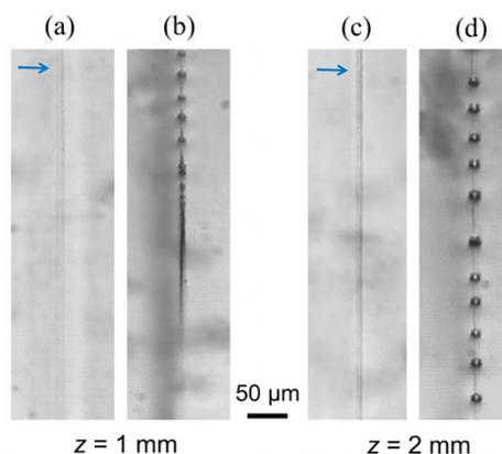
Figure 2. Effect of DVB concentration on droplet formation inside the channel. (a) and (c) correspond to 0.5 wt% DVB and 95.5 wt% ethanol, (b) and (d) to 10 wt% DVB and 90 wt% ethanol. The flow direction is upward. Arrows indicate the grey lines which show nanodroplets in the case of 0.5 wt% DVB
