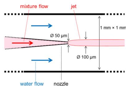
Figure 1. Flow configuration of the 3D co-flow microfluidic jet
