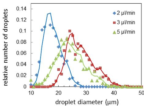
Figure 4. Size distribution of microdroplets for various  $Q_{jet}$  at  $z_{drop}$
