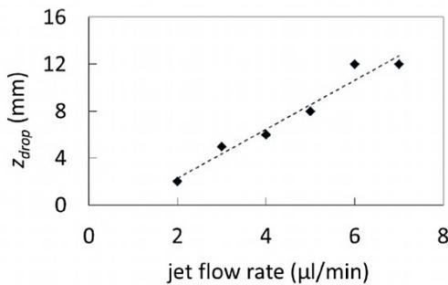
Figure 3. Position of microdroplet formation in terms of jet flow rate
