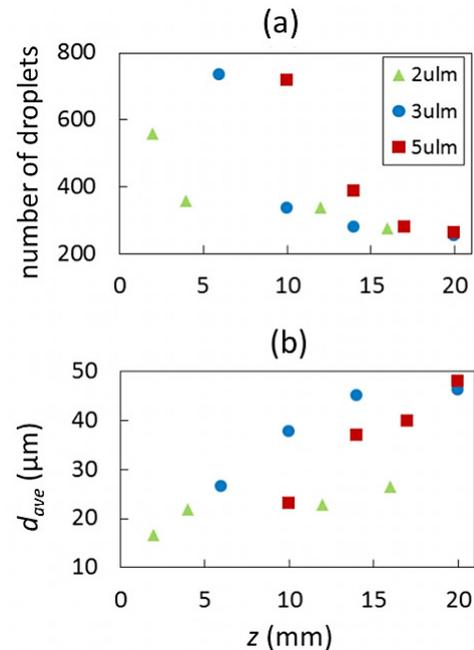
Figure 5. Change of number (a) and average size (b) of droplets along the channel
