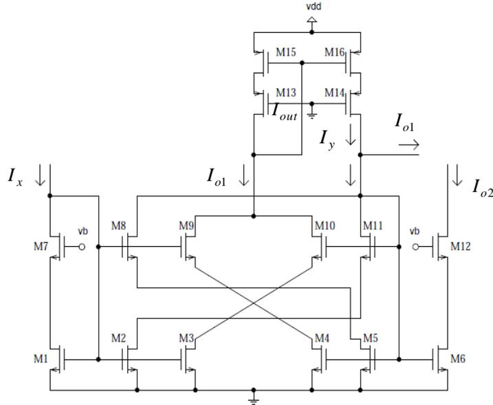
Fig.3 : proposed geometric mean circuit
