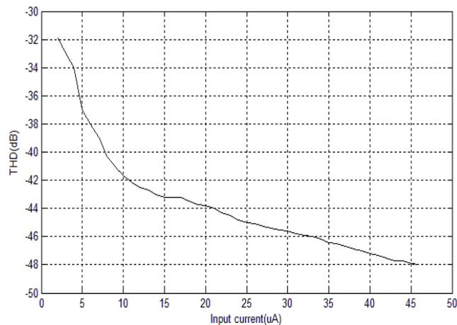
Fig. 6: Nonlinearity performance of the filter
