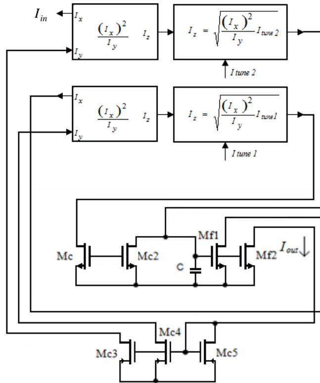
Fig.2: Block diagram of the SRD first-order LPF
