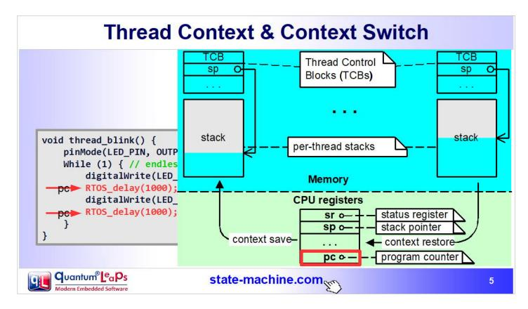
How does the RTOS achieve multitasking? Well, each thread in an RTOS has a dedicated private **context** in RAM, consisting of a private stack area and a thread-control-block (TCB).
