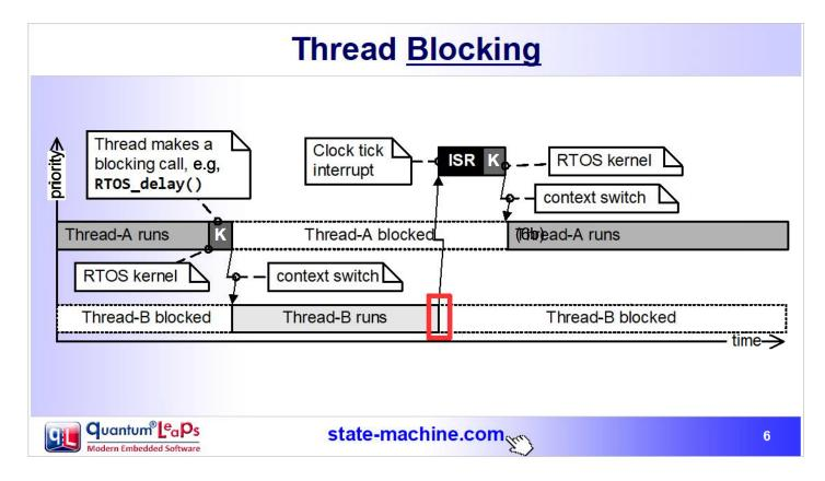
For example, a call to RTOS\_delay() from Thread-A results in a context switch to Thread-B.
