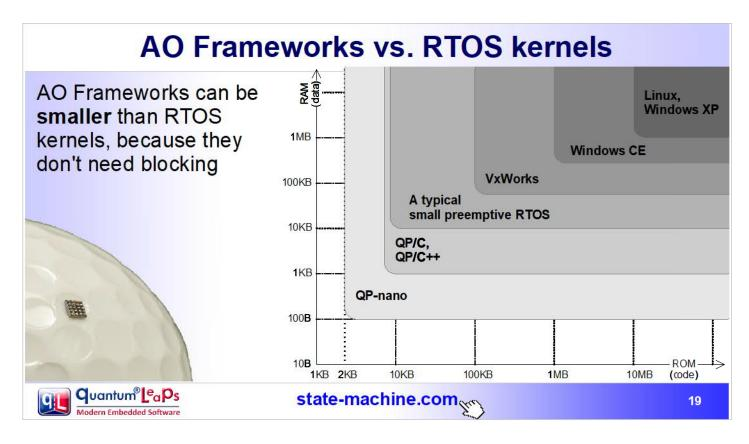
In the resource-constrained embedded systems, the biggest concern has always been about the size and efficiency of Active Object (Actor) frameworks, especially that commercial frameworks of this type accompanying various modeling tools have traditionally been built on top of a conventional RTOS, which adds memory footprint and CPU overhead to the final solution.
