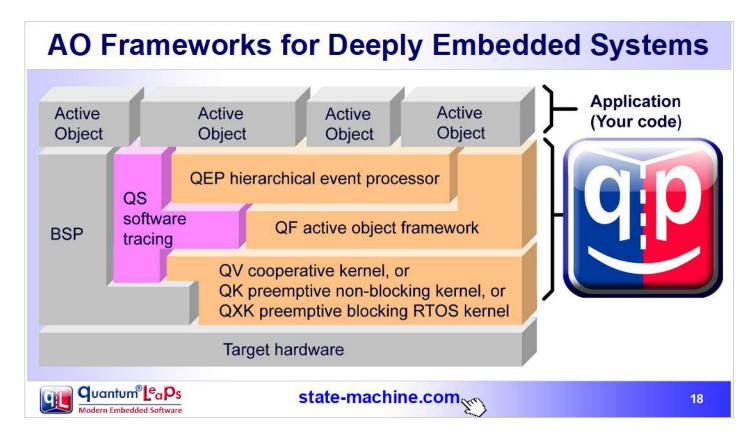
So, how do you bring it all together, in a consistent active object framework? Well, as it turns out most of such frameworks end up with a similar layered structure. Here, for example, is the structure of a minimal active object framework for RTE systems called QP:
