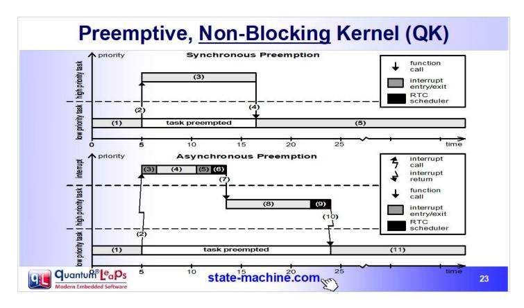
The second non-standard kernel provided in QP is really interesting. It is a very efficient, **preemptive**, priority-based, **non-blocking** kernel called QK. This kernel does not allow threads to block in the middle of run-to-completion step, but allows them to **preempt** each other (such threads are classified as "basic threads" in the OSEK/VDX terminology). The non-blocking limitation is irrelevant for event-driven active objects, where blocking is not needed anyway.
