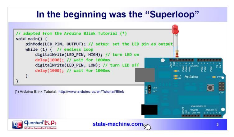
Smaller embedded systems are typically designed as a "superloop" that runs on a bare-metal CPU, without any underlying operating system. This is also the most basic structure that all embedded programmers learn in the beginning of their careers.
