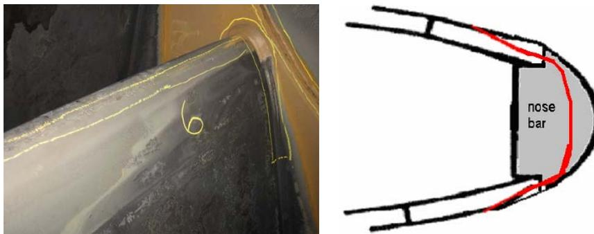
**Figure 20.** Airfoil Impeller Blade with Erosion
