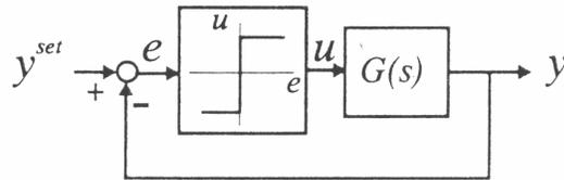
When constant cycles appear after the system has been activated, the ultimate gain and ultimate frequency of the open-loop system can be approximated by measuring the magnitude and period (see the following figure) and by the following equations:
