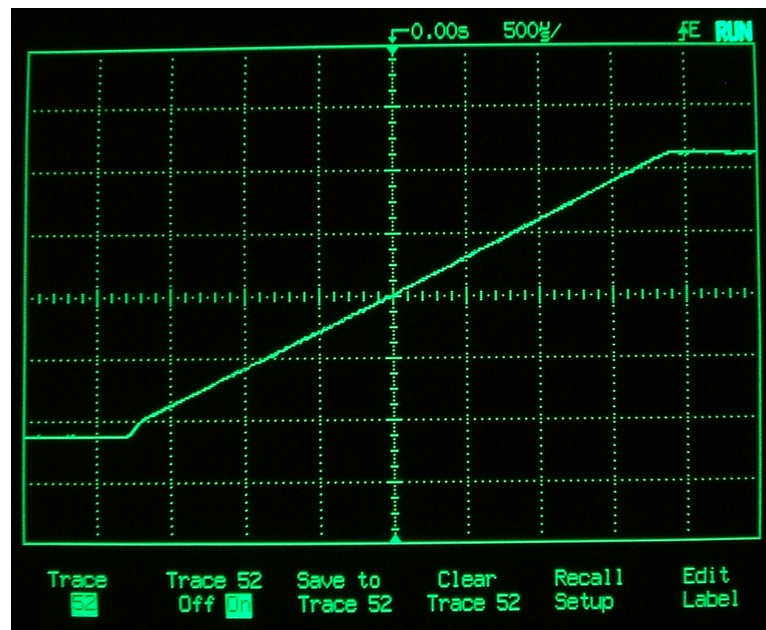
Figure 4.13: Experimental results of the DC transfer characteristic of the circuit in Fig. 4.11.
