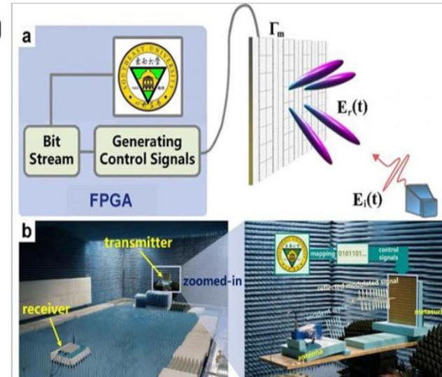
(a) Schematic of the proposed BFSK wireless communication system based on the time-domain digital coding metasurface. (b) Experimental scenario of the BFSK wireless communication system. (c-d) The received messages by the BFSK wireless communication system for different receiving angles, showing stable communication abilities. Courtesy of Science China Press.
