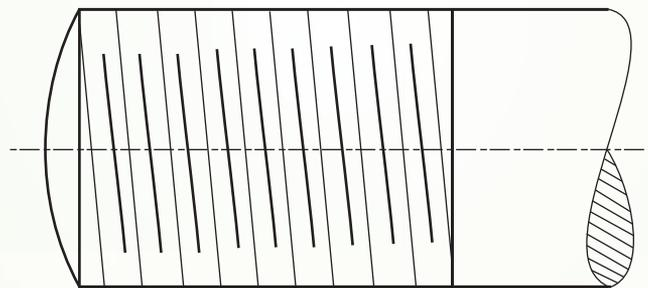
**(A) PARALLEL THREAD**
