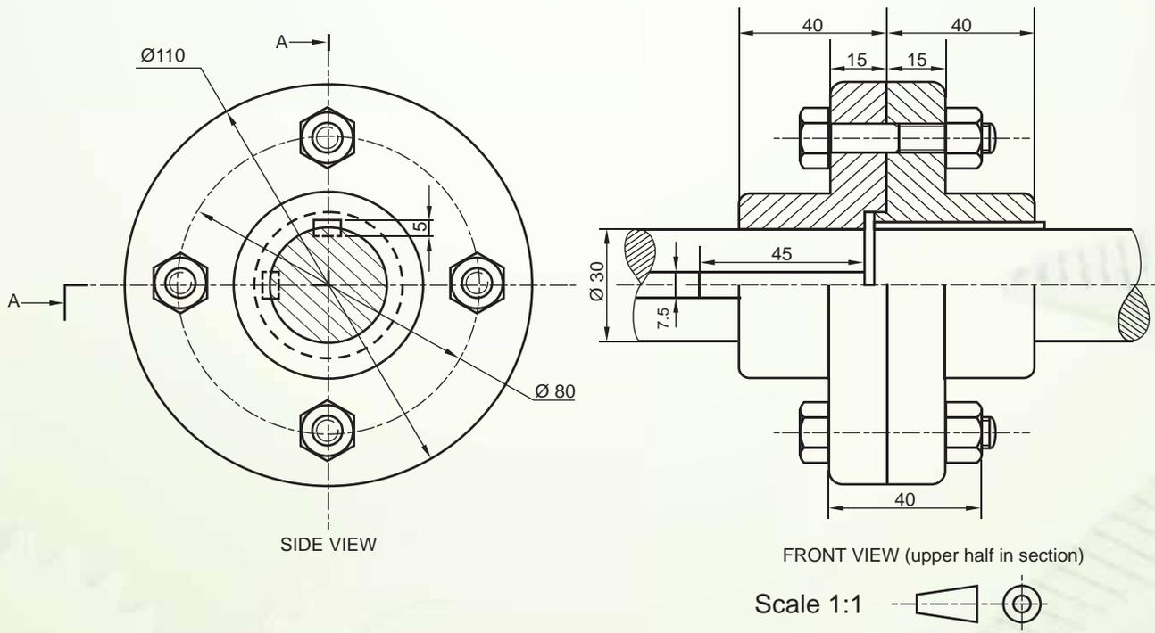
ASSEMBLED VIEWS OF AN UNPROTECTED FLANGE COUPLING
