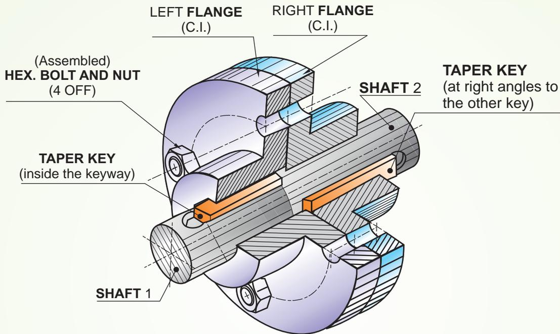
**ASSEMBLY OF AN UNPROTECTED FLANGE COUPLING
