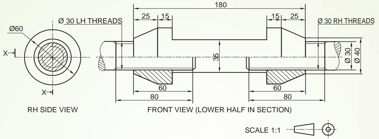
**ASSEMBLED ORTHOGRAPHIC VIEWS OF A TURNBUCKLE.**
