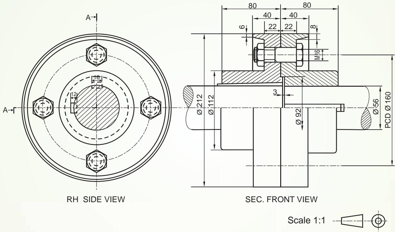
ASSEMBLY OF A PROTECTED FLANGE COUPLING
