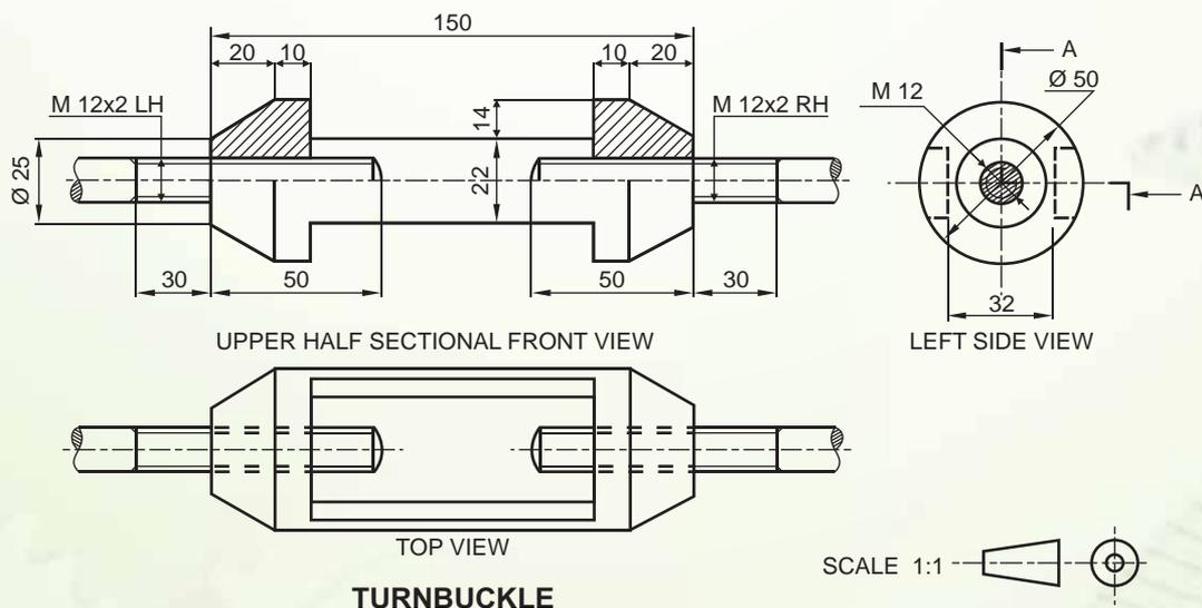
**ASSEMBLY OF A TURNBUCKLE (ORTHOGRAPHIC VIEWS)**
