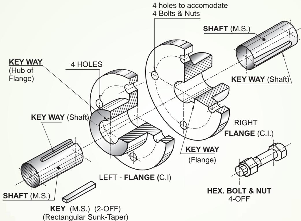
DETAILS OF AN UNPROTECTED FLANGE COUPLING
