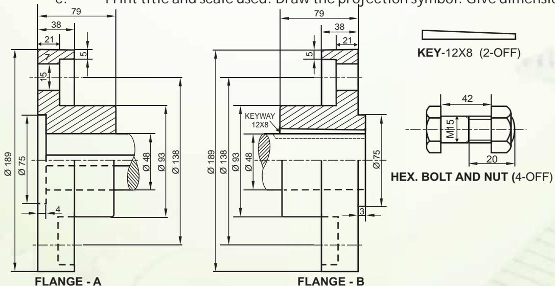
DETAILS OF A PROTECTED FLANGE COUPLING
