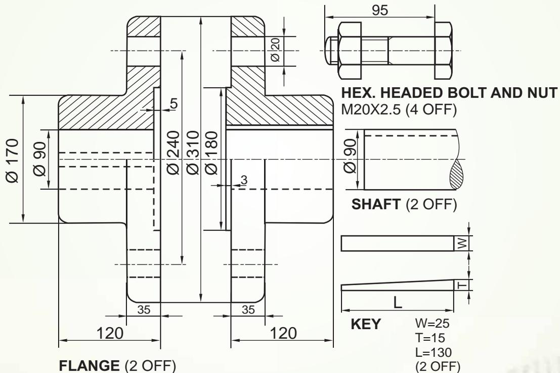
DETAILS OF AN UNPROTECTED FLANGE COUPLING
