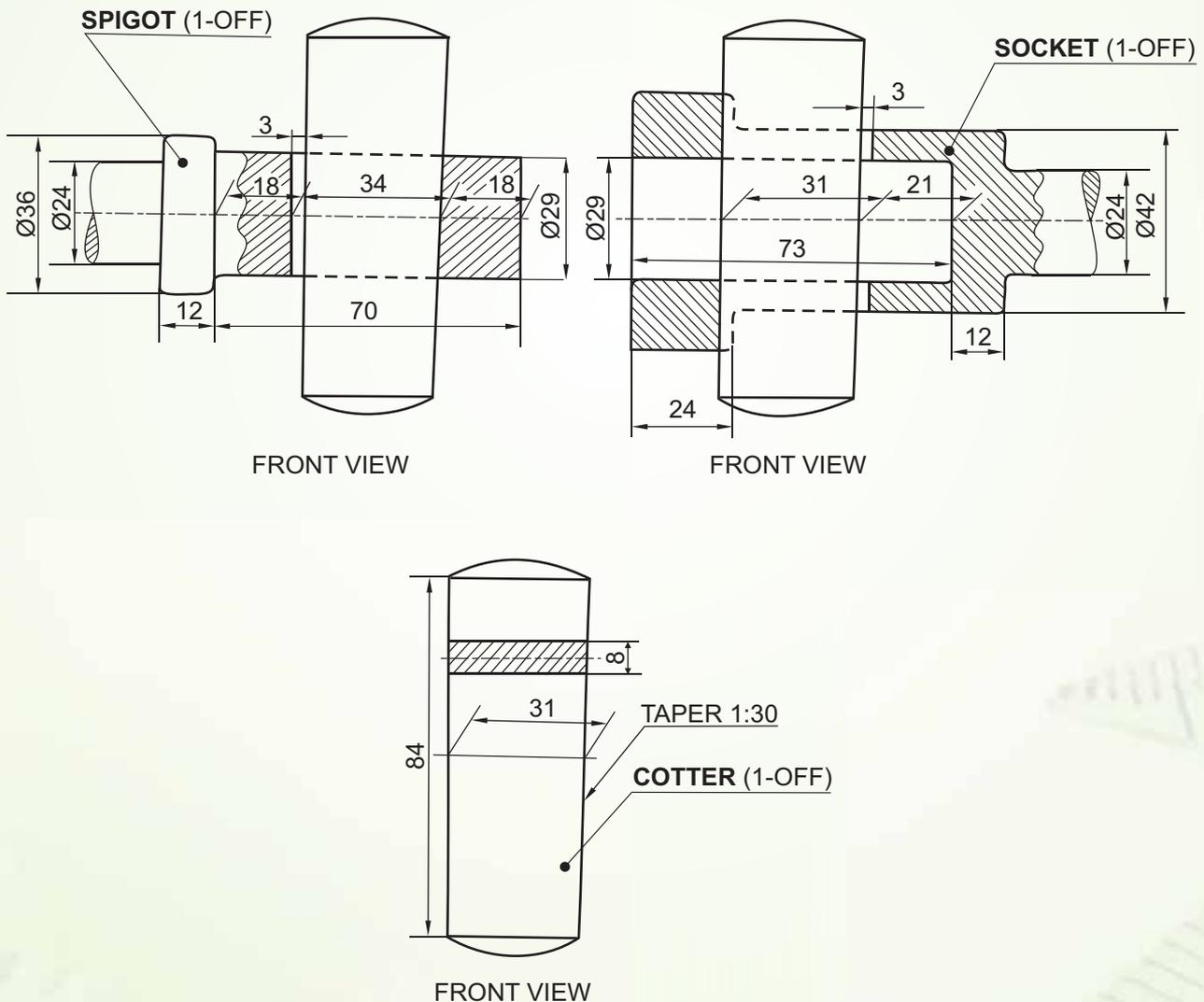
**DETAILS OF A SOCKET AND SPIGOT COTTER JOINT**
