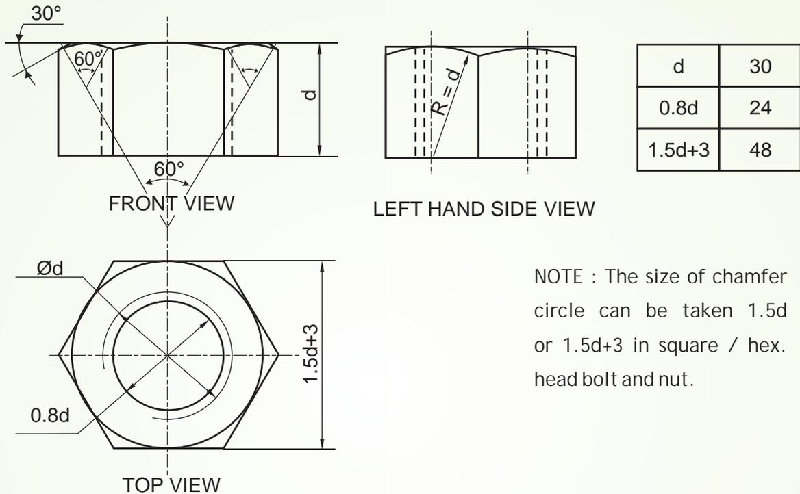
NOTE : The size of chamfer circle can be taken 1.5d or 1.5d+3 in square / hex. head bolt and nut.
