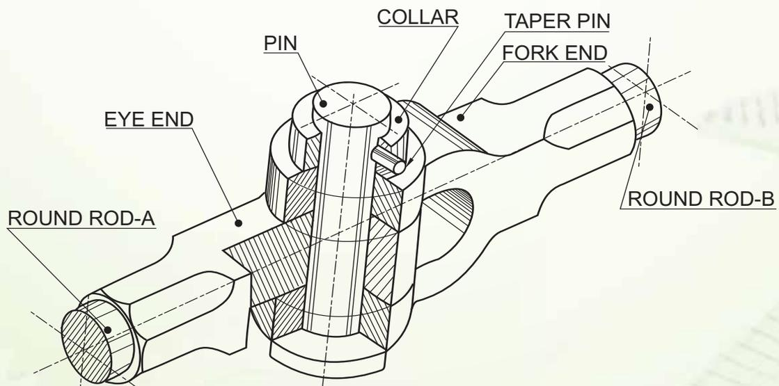
**SECTIONAL ASSEMBLY OF A KNUCKLE JOINT**
