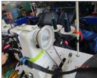
Photo of non-conformity 7.17 No safeguards of pulley.JPG
